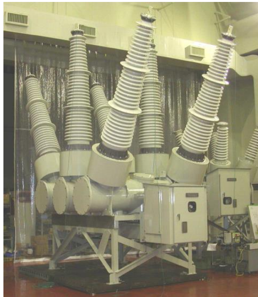
Fig. 1.4 168 kV/40 kA double-break tank-type vacuum circuit breaker [8] .
