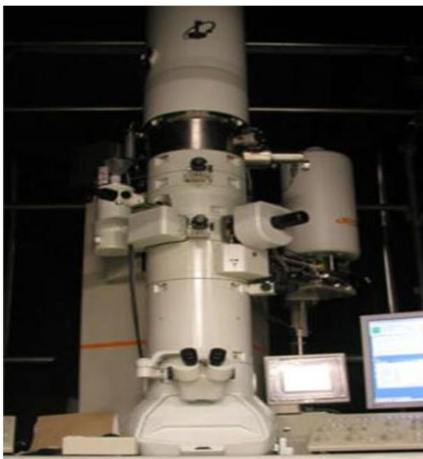
**Figure 2.4** Transmission electron microscope (JEM-2100, JEOL).
