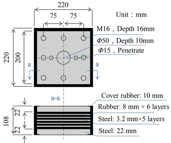
Fig. 3: Bearing specimen
