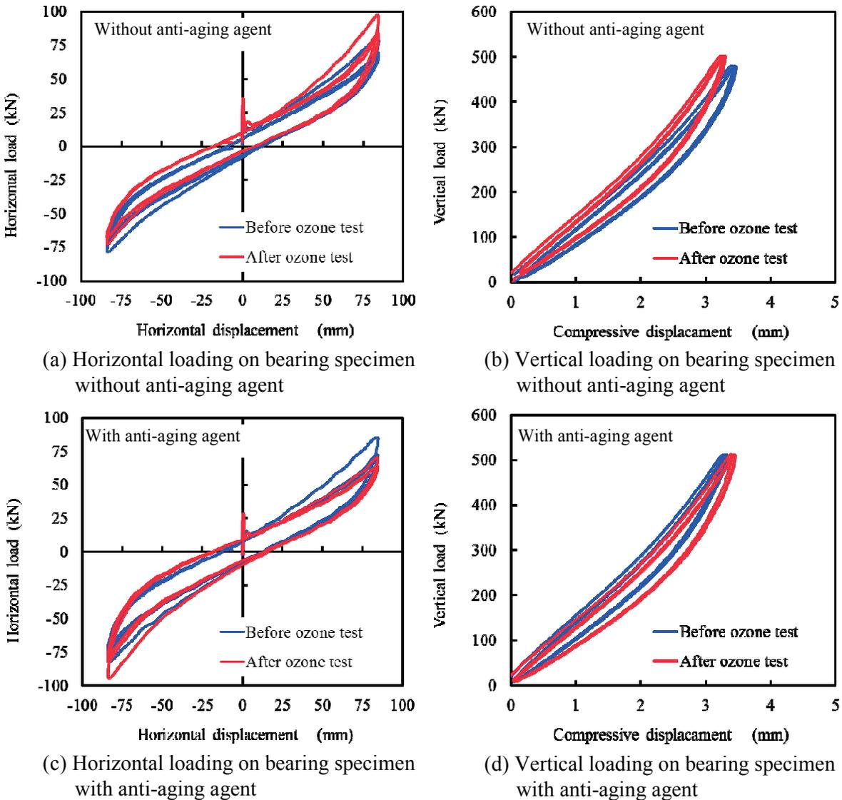
Fig. 9: Results of loading experiment on bearing specimens
