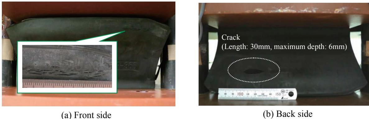
Fig. 8: Cracks of bearing specimen with anti-aging agent
