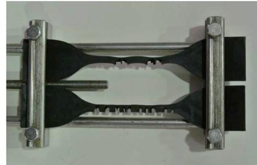
*Fig. 7: Damaged dumbbell specimen (23 degrees Celsius, Ozone 100 pphm, pre-strain 80%)*
