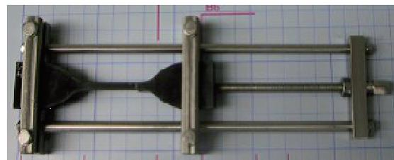
*Fig. 2: Dumbbell specimen with pre-strain*
