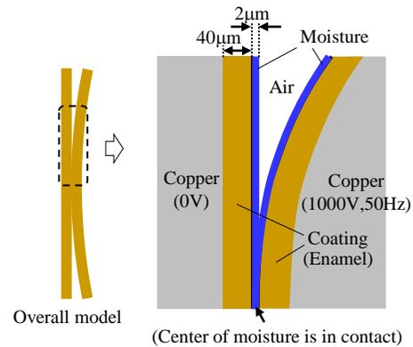
Figure 9. Calculation model for electric field distribution.
