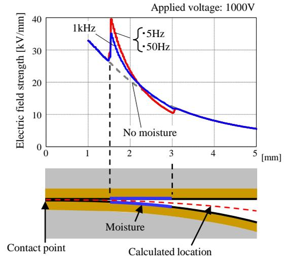
**Figure 12.** Electric field strength when moisture layer is attached to coil coating except contact point.
