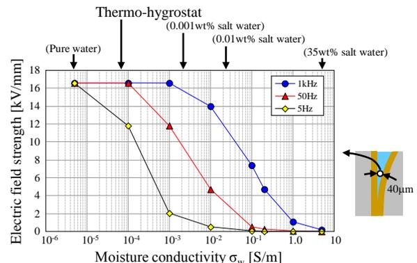
Figure 10. Electric field strength in air gap as a function of moisture conductivity.
