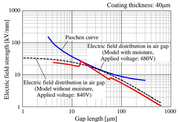
**Figure 13.** Relationship between electric field distribution in air gap and Paschen curve (Moisture layer is attached to coil coating except contact point).
