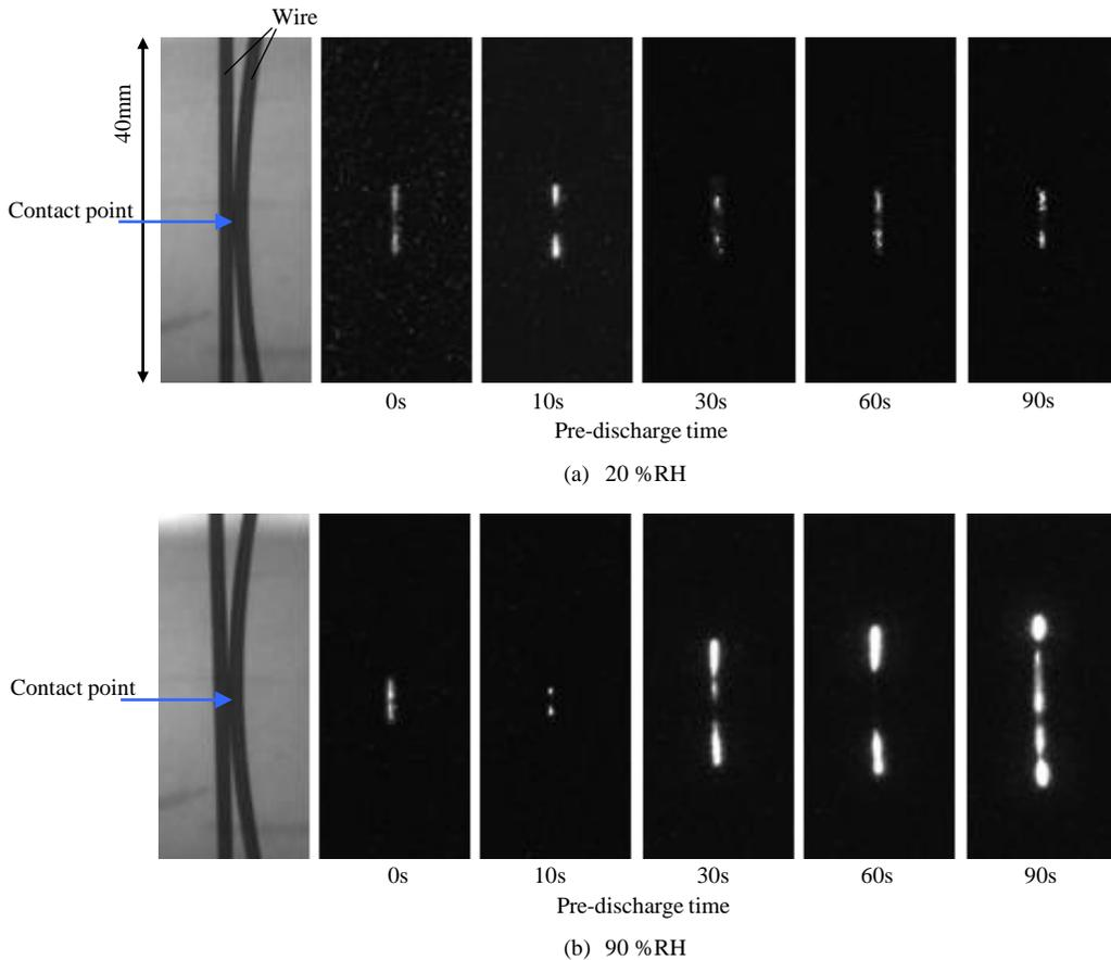
Figure 7. PD luminescence images for different ambient humidity (at PDIV @ 50 Hz, Sample A)
