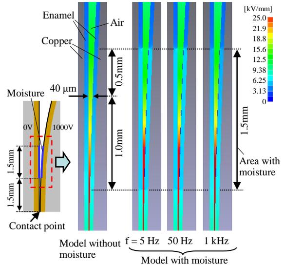
**Figure 11.** Electric field distribution for different frequencies (Moisture layer is attached to coil coating except contact point).
