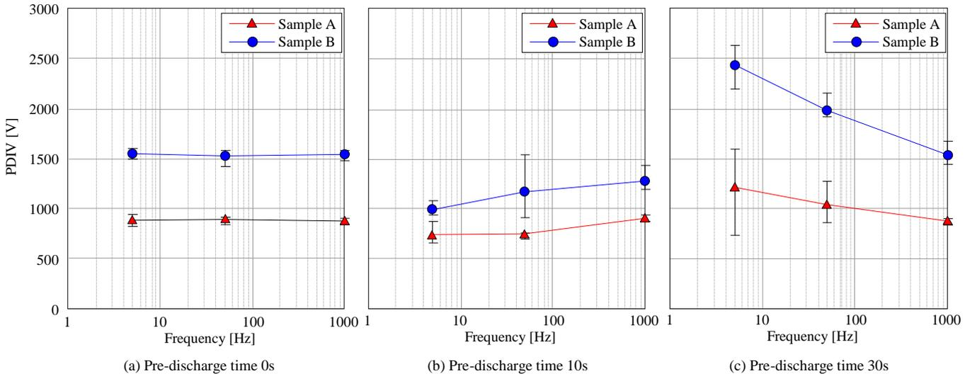
Figure 6. Frequency dependence of PDIV for different insulation thickness and pre-discharge time (90 %RH).
