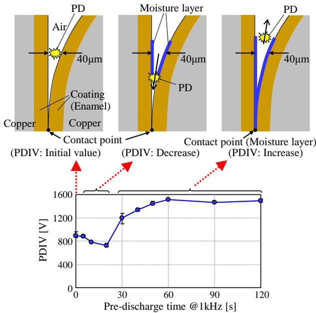
**Figure 17.** Change of moisture adhesion area, PD location and PDIV value for pre-discharge time at high humidity.
