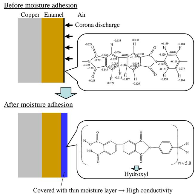
Figure 8. Mechanism of moisture in the air to adhere to coating surface<sup>[12]</sup>.
