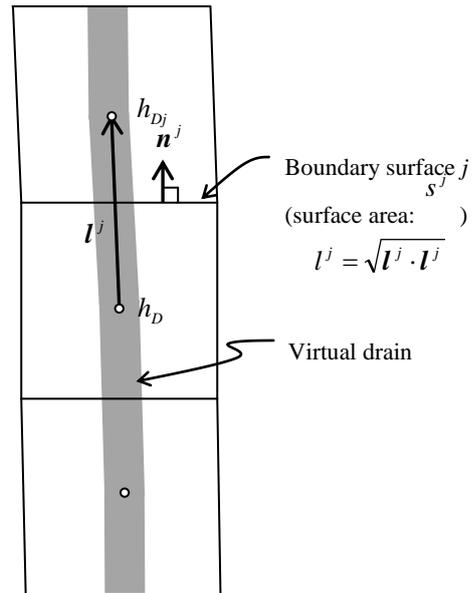
Fig. 1. Virtual drain contained in mesh.
