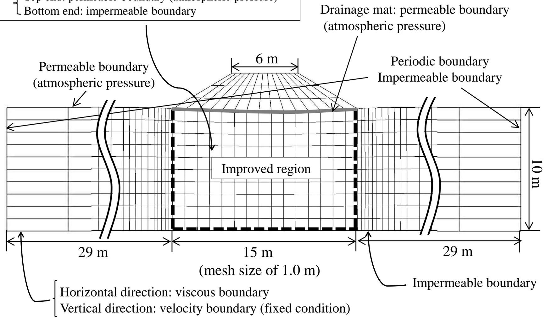
Fig. 4. Finite element mesh and boundary conditions (approximate model).
