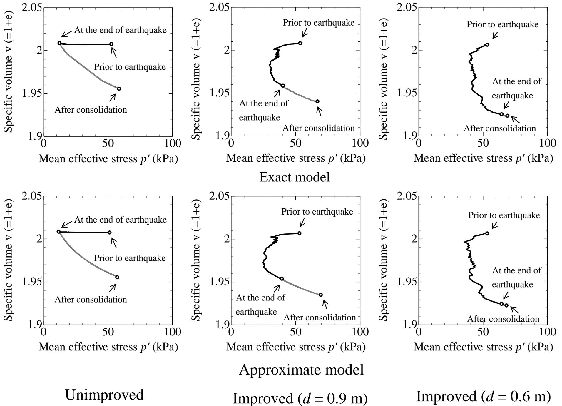
Fig. 15. Relationships between the mean effective stress and the specific volume.
