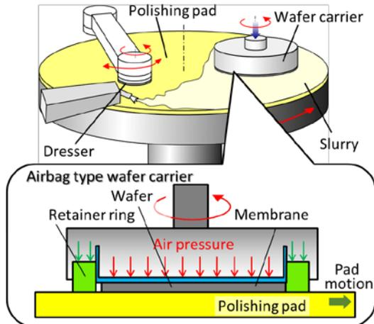
Fig. 1. Schematic illustration of general configuration of CMP process.
