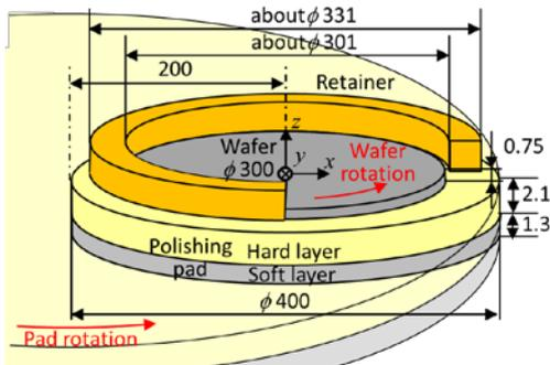
Fig. 4: Structural analysis model.
