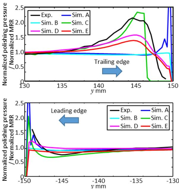
**Fig. 7.** Polishing pressure profiles around trailing edge (upper) and leading edge (lower) comparing with normalized MRR profile.
