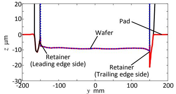
Fig. 6. Estimated contact surface deformations of polishing pad, wafer and retainer ring.
