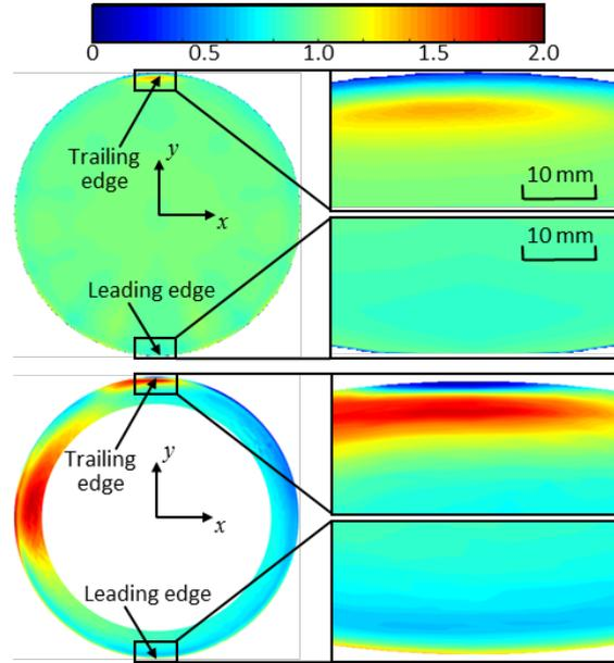
Fig. 5. Simulated contact pressure distributions (upper) and normalized MRR distribution (lower).
