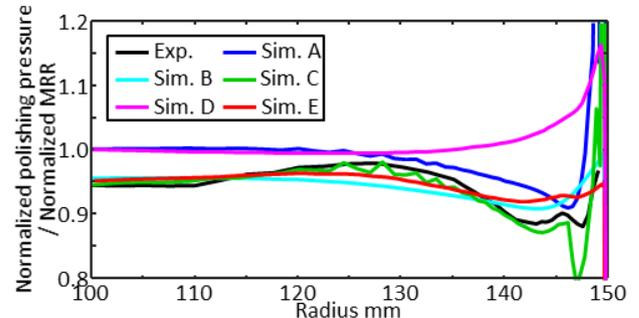
**Fig. 8.** Radially-averaged polishing pressure profiles compared with MRR.
