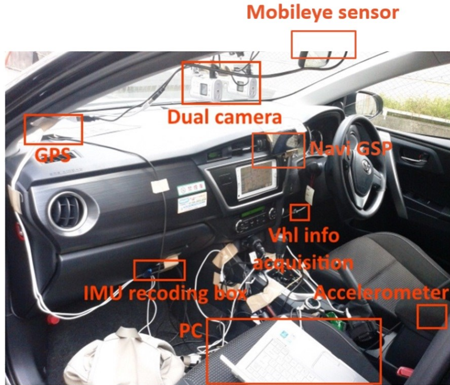
Figure 2.12: Internal combustion engine vehicle sensing setup.
