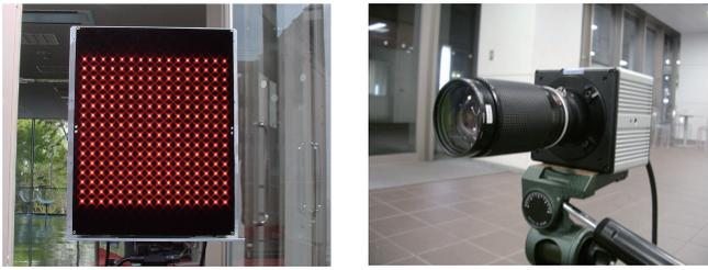
(a) LED array (b) High-speed camera
