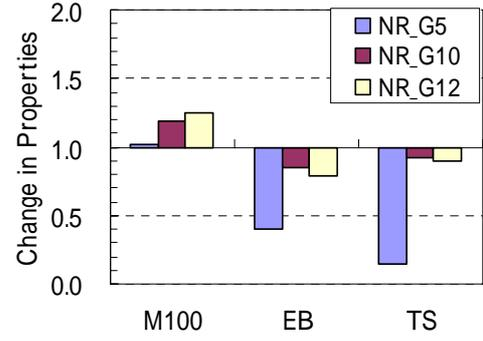
Fig.12 Change in properties of NR (pre-strain=40%, 720 hours)
