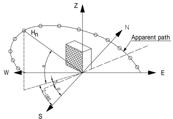
Fig.14 Angle diagram for finding solar radiation on vertical surfaces
