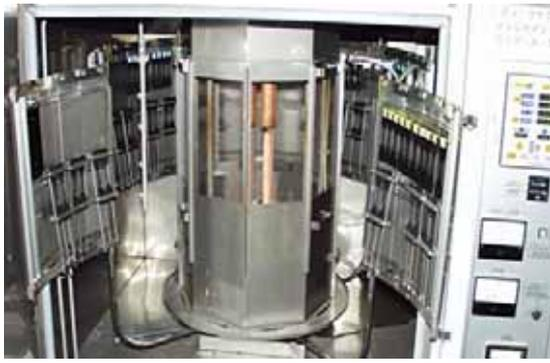
Fig.5 Dew cycle sunshine weather meter
