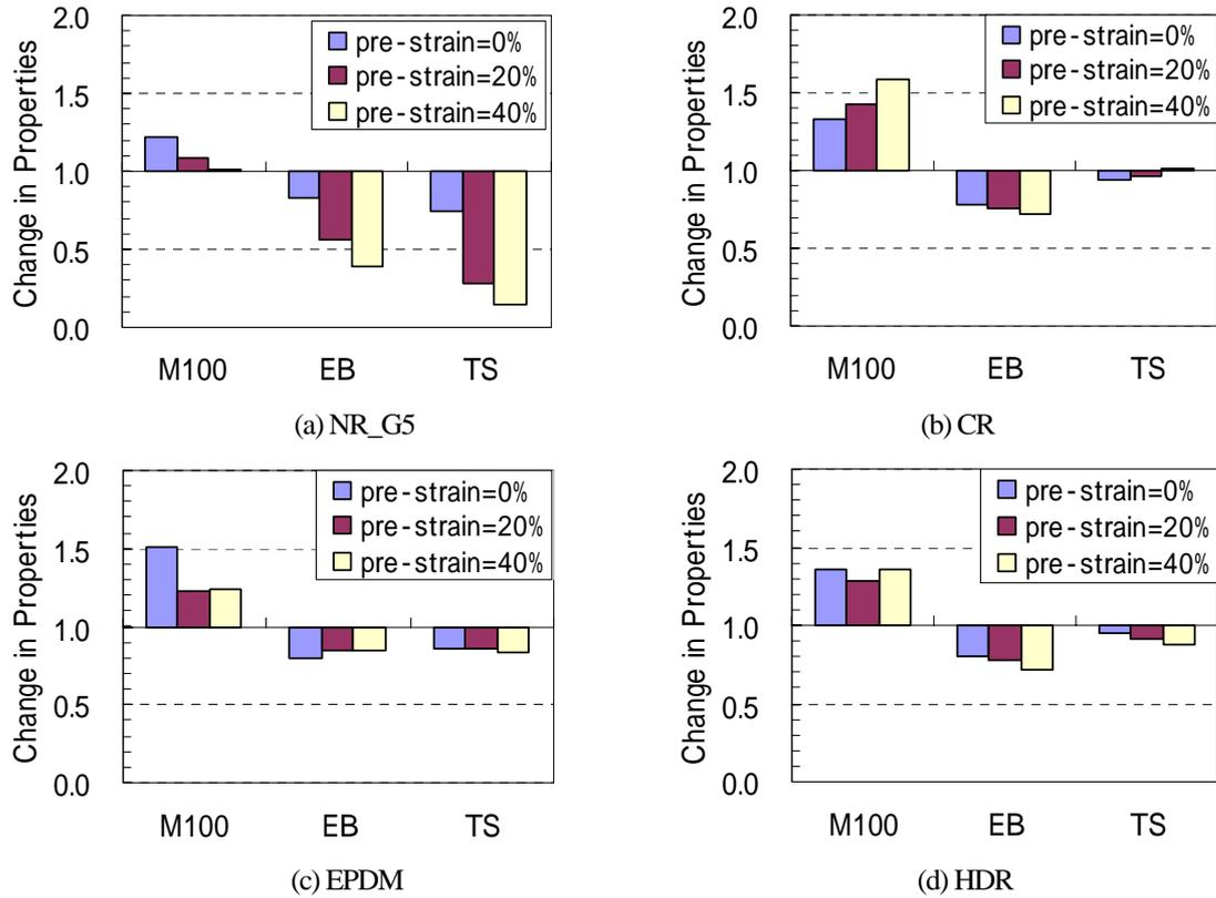
Fig.8 Influence of pre-strain on ultraviolet deterioration (720 hours)
