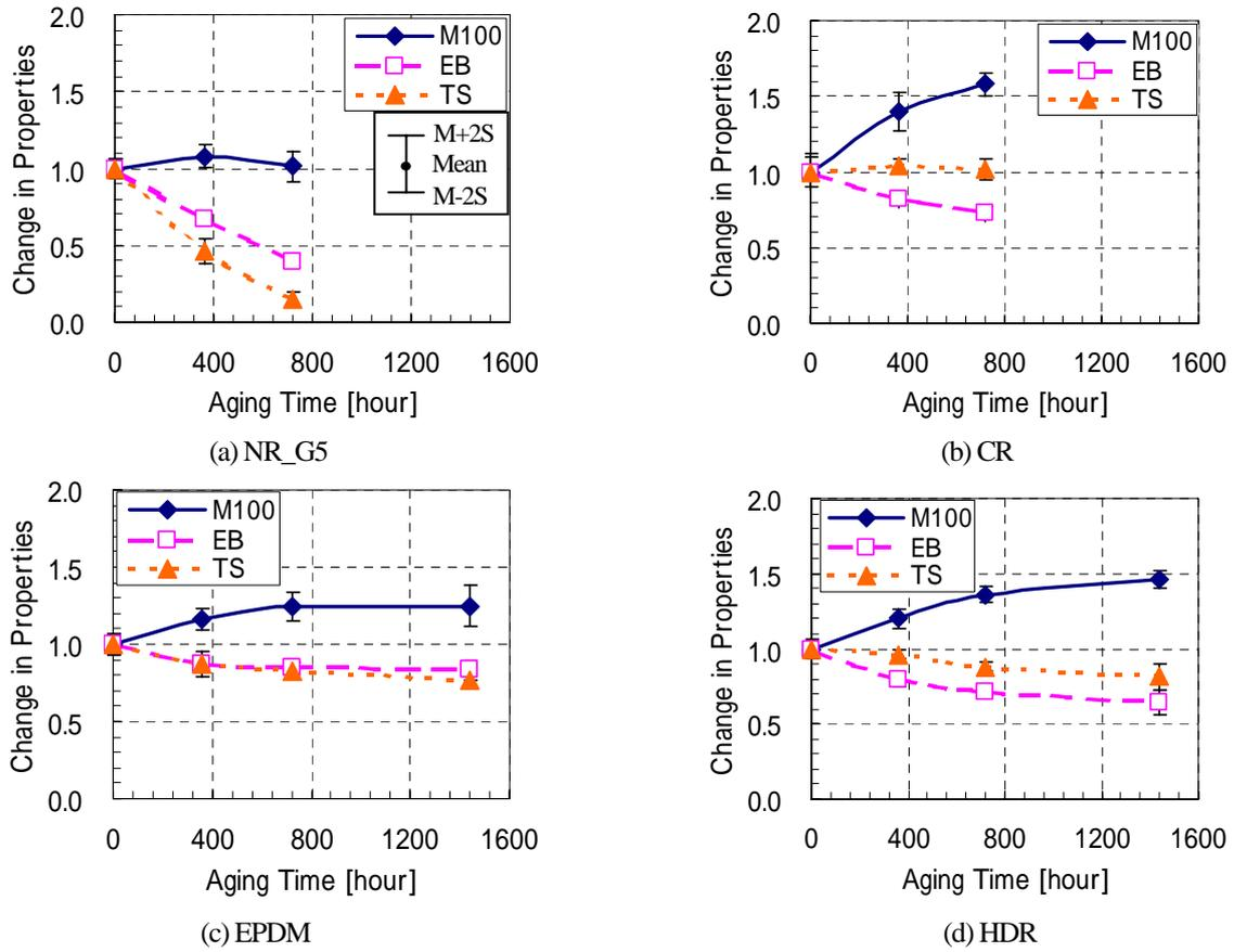
Fig.7 Time-dependency of rubbers subjected to ultraviolet irradiation (pre-strain=40%)
