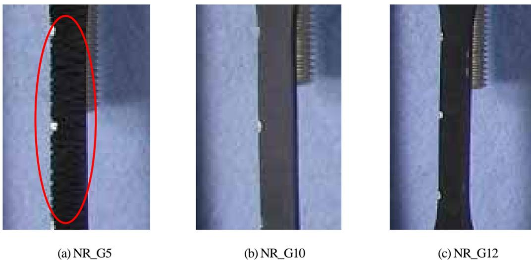
Fig.10 Appearance of NR samples after 720 hours' ultraviolet irradiation
