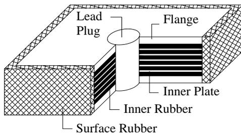
Fig.1 Bridge rubber bearing
