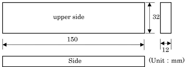
**Figure 1. Test Specimen**
