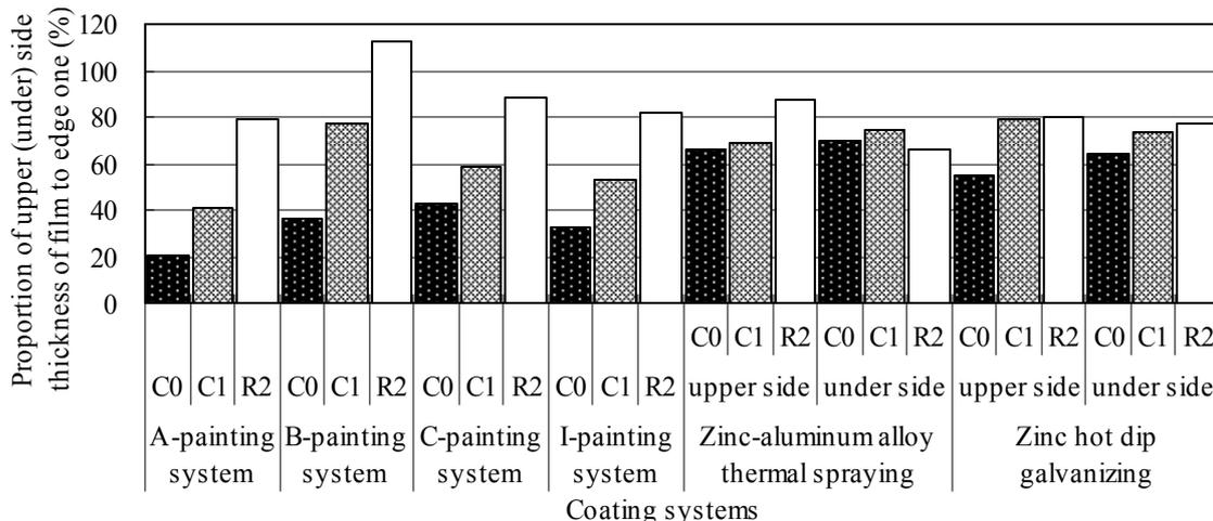
Figure 5. Thickness of coating films
