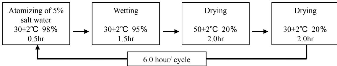
Figure 4. Accelerated exposure test condition (S6-cycle)
