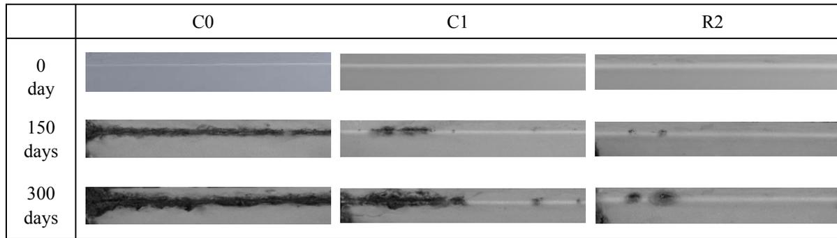
**Figure 6. Corrosion progress (A-painting system)**
