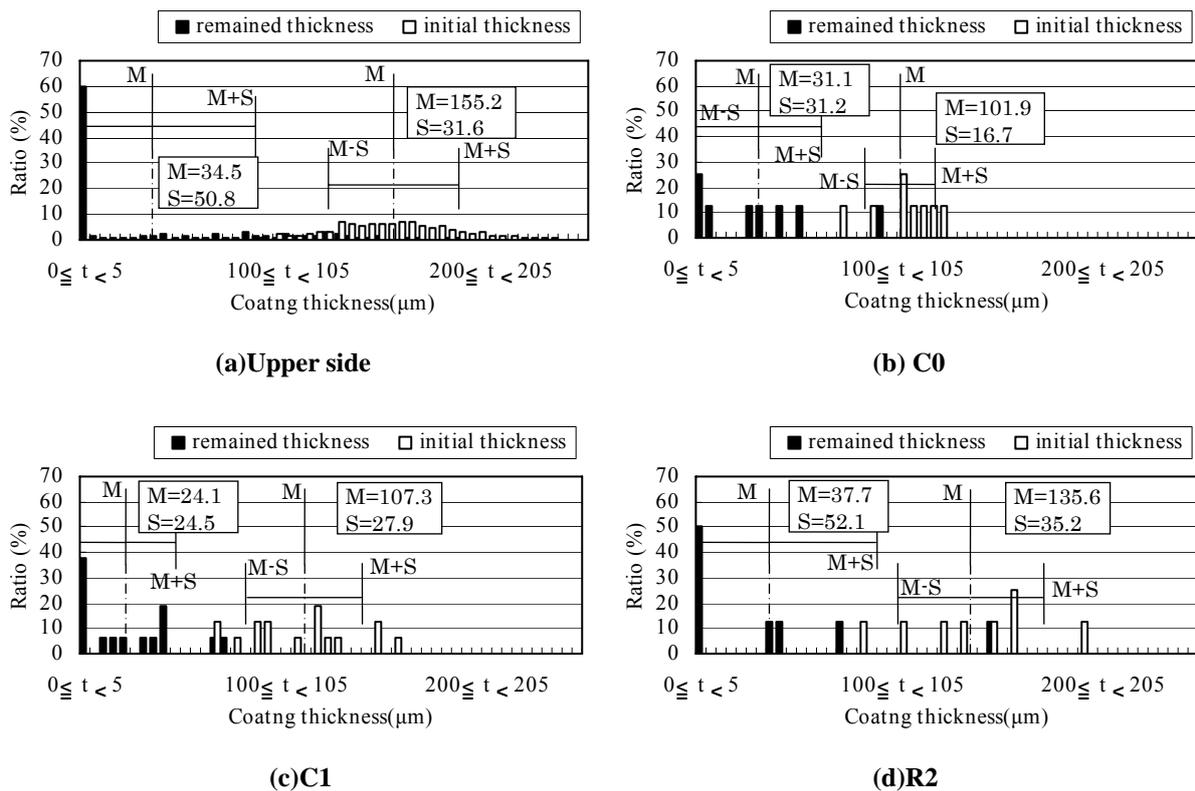
Figure 8. Distributions of coating thickness (zinc-aluminum alloy thermal sprayed coating)
