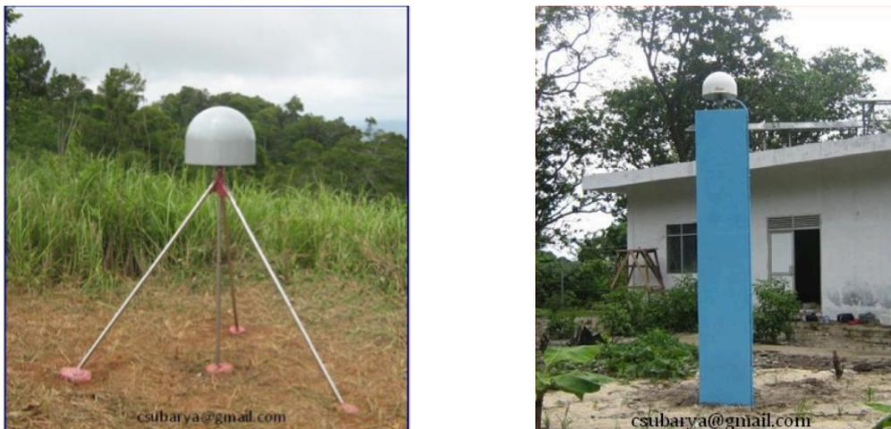
Figure 4.2. Example of cGPS pillar. Left. CSGT in Sagaranten. Right. CUJG in Ujung Kulon.
