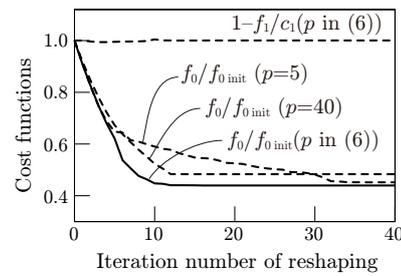
Fig. 4. Iteration histories of cost functions with respect to reshaping.
