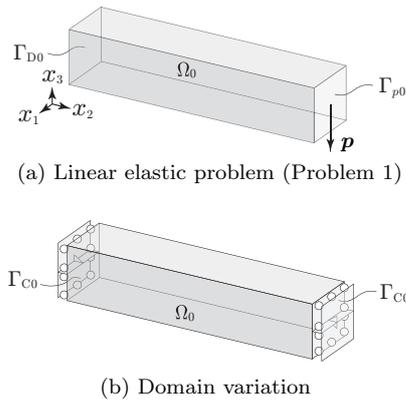
Fig. 2. Boundary conditions in the cantilever problem.
