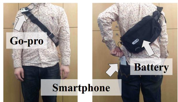
**Fig. 2** Recording equipment worn by subjects. Note that the video camera is only for data annotation purposes and is not part of the target system.
