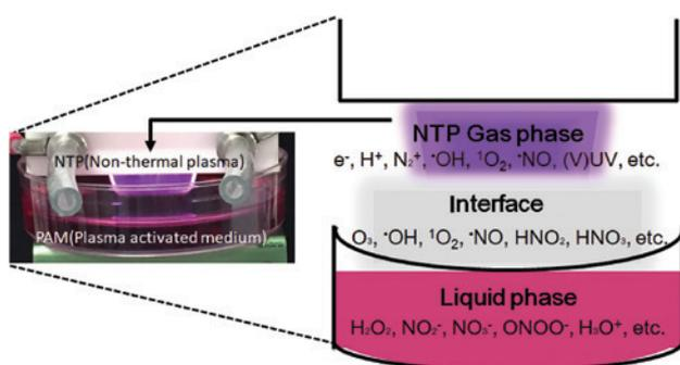
**Figure 1:** Interactions between NTP and liquid in PAM.
