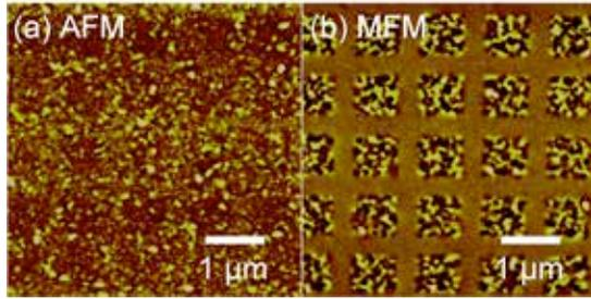
Fig. 5. (a) AFM and (b) MFM images of an ion-beam patterned MnGa film on Si substrate with a pitch size of 1000 nm.
