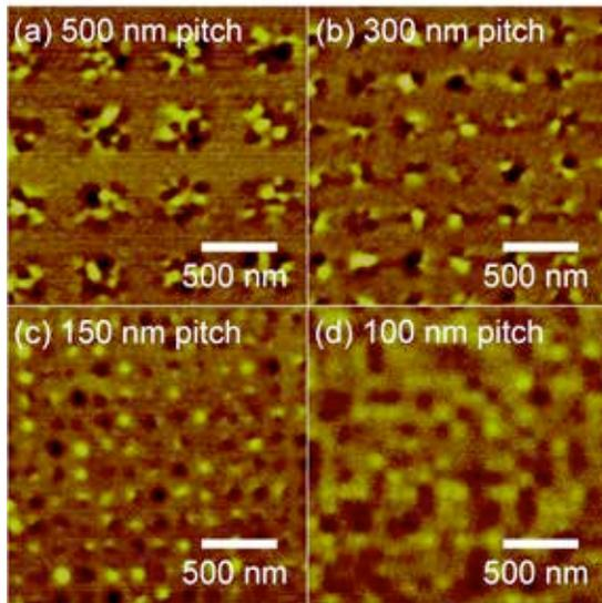
Fig. 6. MFM images of an ion-beam patterned MnGa film on Si substrate with pitch sizes of (a) 500, (b) 300, (c) 150, and (d) 100 nm.
