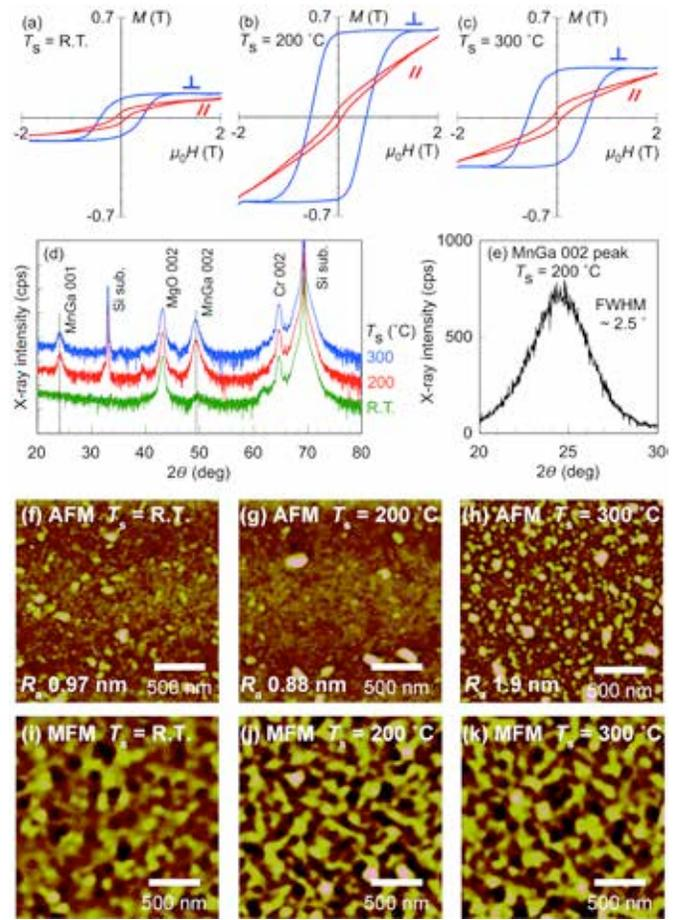
Fig. 4. (a) – (c)  $M$ - $H$  curves, (d) XRD patterns, (e) rocking curve of MnGa 002 peak, (f) – (h) AFM images, and (i) – (k) MFM images of MnGa films grown on the Cr buffer layer annealed at  $T_a^{\text{Cr}} = 800$  °C. The substrate temperature  $T_s$  during the growth of MnGa layer was varied at R.T., 200, and 300 °C. The dashed lines in Fig. (d) show the peak positions of the bulk MnGa.
