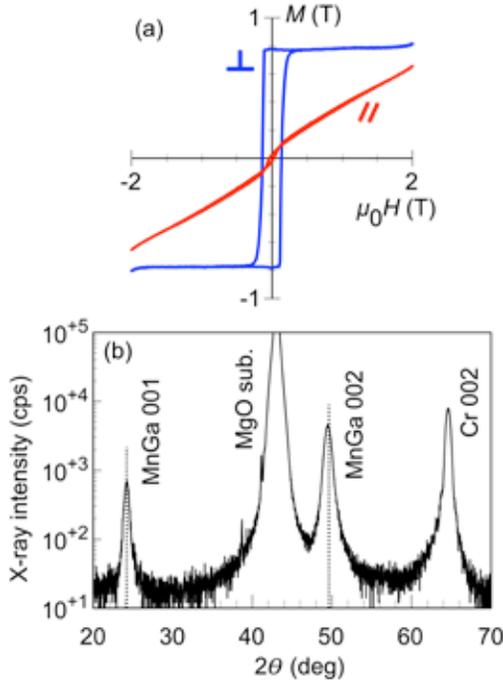
Fig. 1. (a) Out-of-plane and in-plane  $M$ - $H$  curves and (b) out-of-plane XRD pattern of a MnGa film grown on a MgO substrate. The dashed lines in Fig. (b) represent diffraction angles estimated from bulk values.
