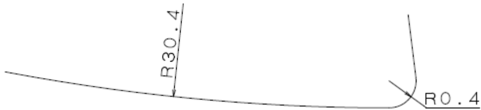
(c) Shape of wiper part Type C.
