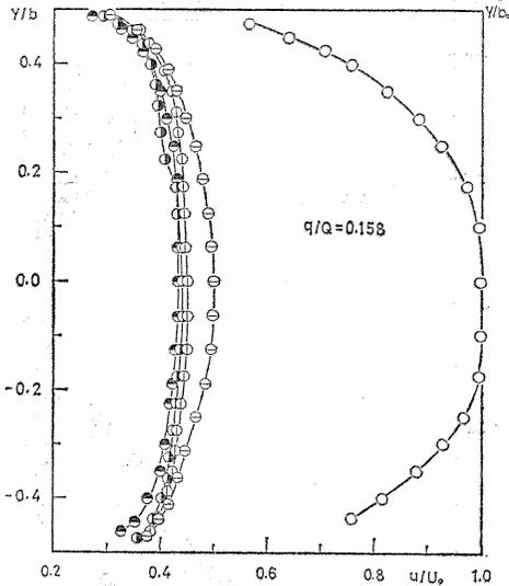
Fig. 4. Velocity distributions in the transverse direction with suction,  $2\theta=20^\circ$ ,  $AR=2$ , designation of marks is the same to Fig. 3.
