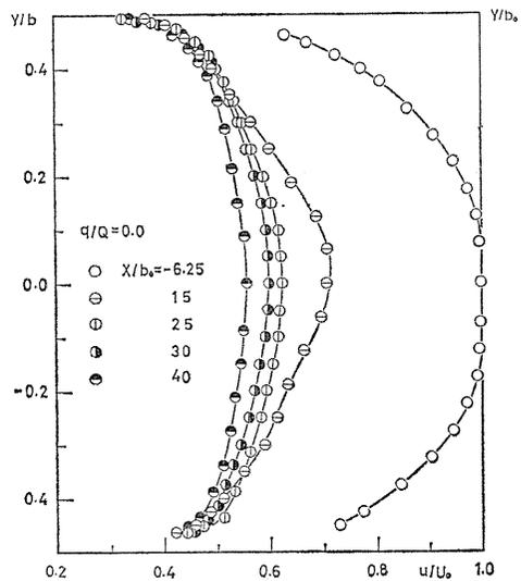
Fig. 3. Velocity distributions in the transverse direction without suction,  $2\theta = 20^\circ$ ,  $AR = 2$ .
