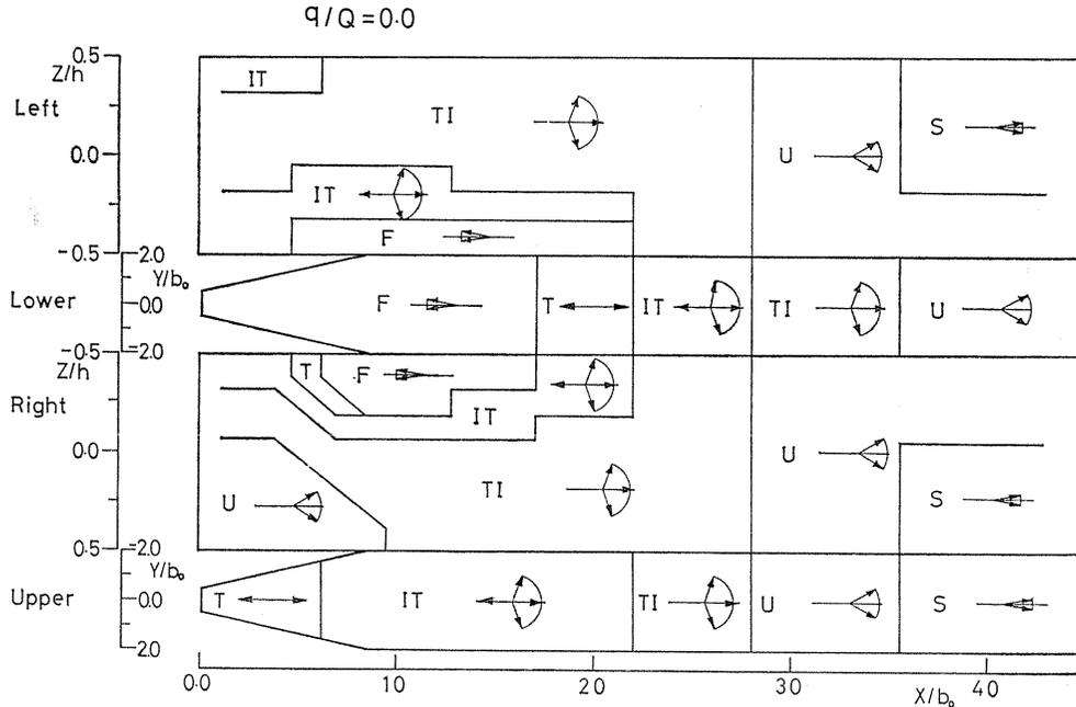
Fig. 18b. Flow pattern in the diffuser with suction,  $2\theta=20^\circ$ ,  $AR=4$ .
