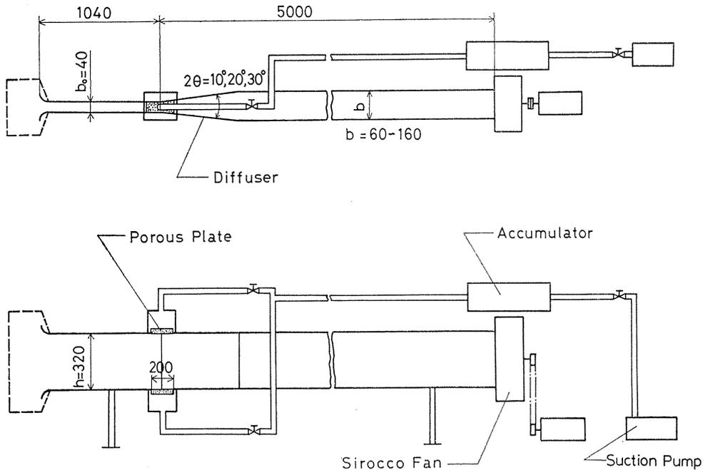
Fig. 1. Wind tunnel and suction system.
