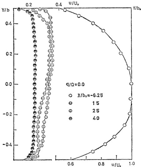
Fig. 8. Development of the transverse velocity distribution without suction,  $2\theta = 20^\circ$ ,  $AR = 4$ .
