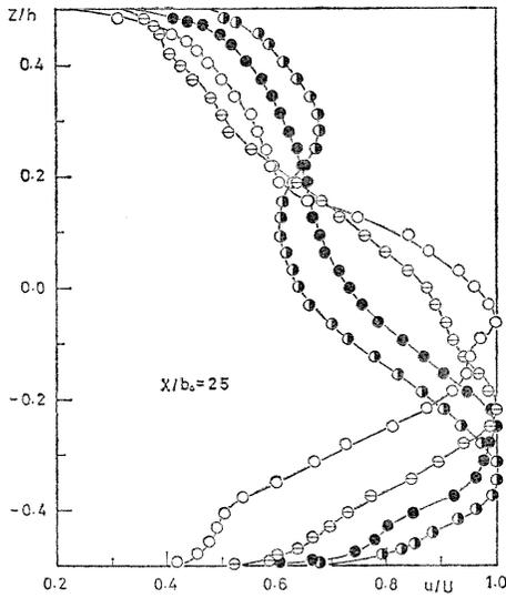
Fig. 12. Deflection of flow in the spanwise direction with suction at  $x/b_0=25$ ,  $2\theta=20^\circ$ ,  $AR=4$ , designation of marks is the same to Fig. 11.
