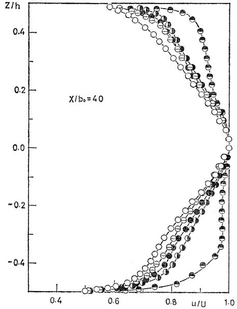
Fig. 7. Variation of the spanwise velocity distribution with suction at  $x/b_0 = 40$ ,  $2\theta = 20^\circ$ ,  $AR = 2$ , designation of marks is the same to Fig. 5.
