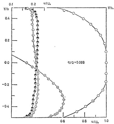
Fig. 9. Large variation of the velocity distributions in the transverse direction with suction  $q/Q = 0.066$ ,  $2\theta = 20^\circ$ ,  $AR = 4$ , designation of marks is the same to Fig. 8.
