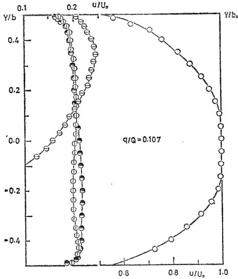
Fig. 10. Variation of the transverse velocity distribution with suction,  $q/Q=0.107$ ,  $2\theta=20^\circ$ ,  $AR=4$ , designation of marks is the same to Fig. 8.
