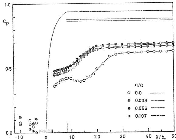
Fig. 15. Step type pressure recovery process,  $2\theta=20^\circ$ ,  $AR=4$ .
