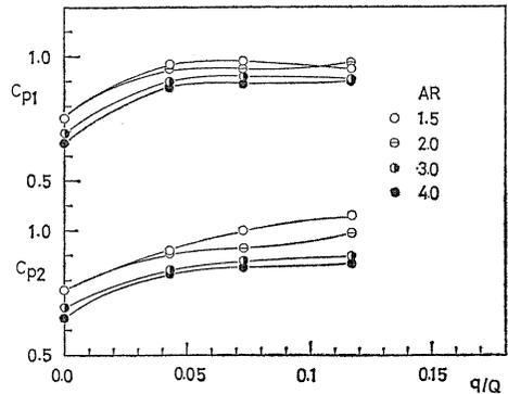
Fig. 17c. Variation of  $C_{p1}$  and  $C_{p2}$ ,  $2\theta=30^\circ$ .
