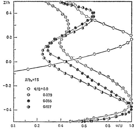
Fig. 11. Wall jet type flow in the spanwise direction at  $x/b_0=15$ ,  $2\theta=20^\circ$ ,  $AR=4$ .
