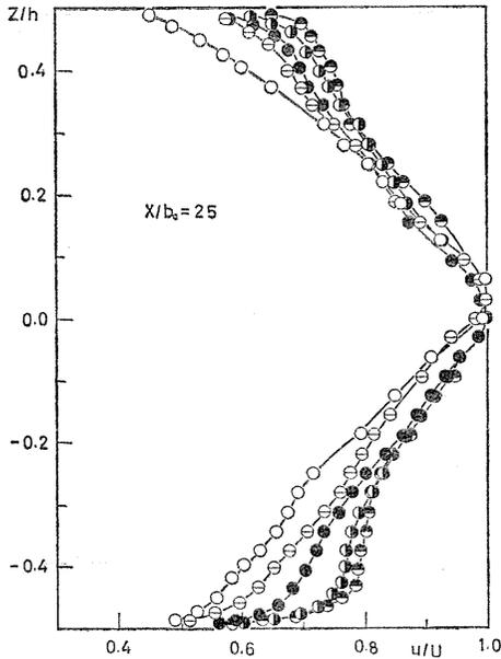
Fig. 6. Variation of the spanwise velocity distribution with suction at  $x/b_0 = 25$ ,  $2\theta = 20^\circ$ ,  $AR = 2$ , designation of marks is the same to Fig. 5.
