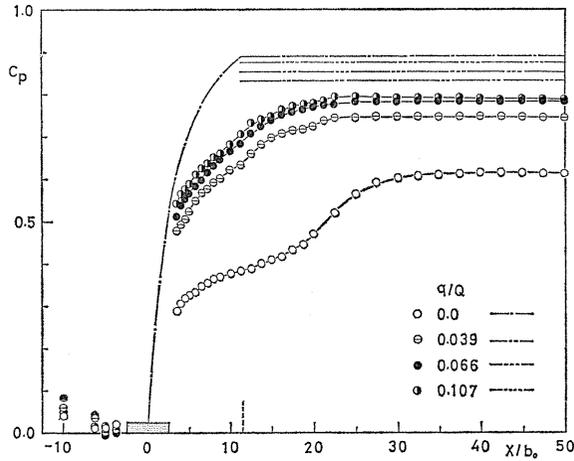
Fig. 16. Step-gradual type pressure recovery process,  $2\theta=20^\circ$ ,  $AR=3$ .
