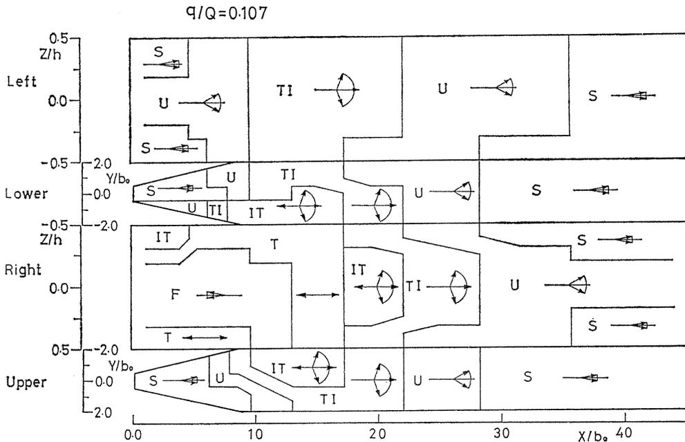
Fig. 18a. Flow pattern in the diffuser without suction,  $2\theta=20^\circ$ ,  $AR=4$ .
