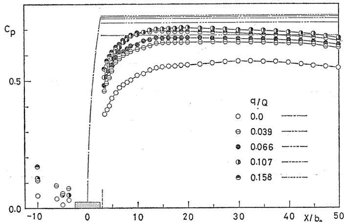
Fig. 14. Gradual type pressure recovery process.  $2\theta=20^\circ$ ,  $AR=2$ .
