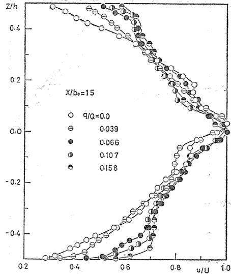
Fig. 5. Variation of the spanwise velocity distribution with suction at  $x/b_0=15$ ,  $2\theta=20^\circ$ ,  $AR=2$ .
