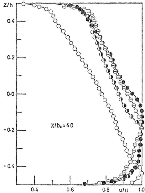
Fig. 13. Variation of the spanwise velocity distribution with suction at  $x/b_0=40$ ,  $2\theta=20^\circ$ ,  $AR=4$ , designation of marks is the same to Fig. 11.
