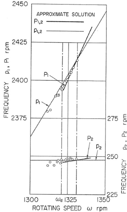
FIG. 8.3. Two vibrations in unstable region near  $\omega_d$
