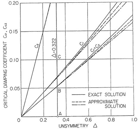
FIG. 3.3. Critical damping coefficients  $c_{c1}$ ,  $c_{c2}$
