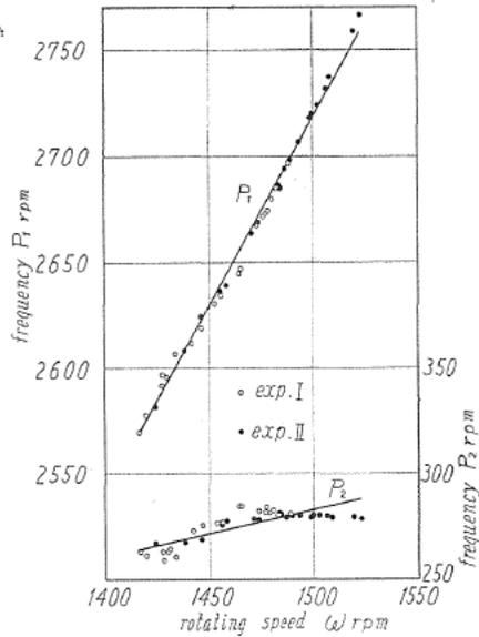
FIG. 6.13. Frequencies  $P_1, P_2$  of unstable vibrations
