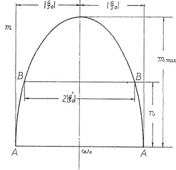
FIG. 5.2. Negative damping coefficient  $m$
