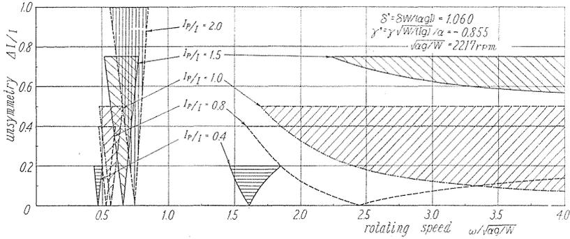
FIG. 2.2. Unstable regions  $[\omega_{c21}, \omega_{c22}]$  and  $[\omega_{c11}, \omega_{c12}]$
