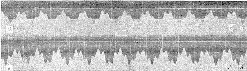
$\omega = 888.0 \text{ rpm}, \omega_0 = 2427.4 \text{ rpm}, \omega'_0 = -651.4 \text{ rpm}, A'/A = 2.4$
