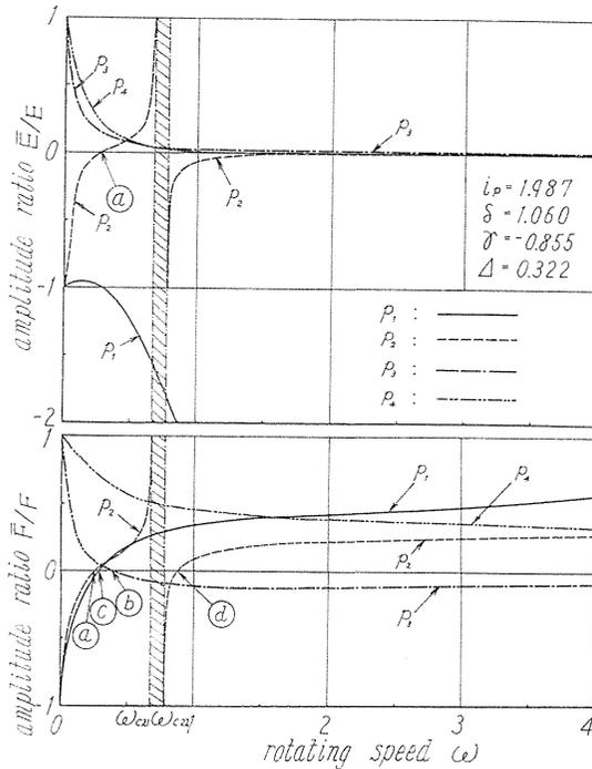
FIG. 2.4. Amplitude ratios of free vibrations (Experiment II)
