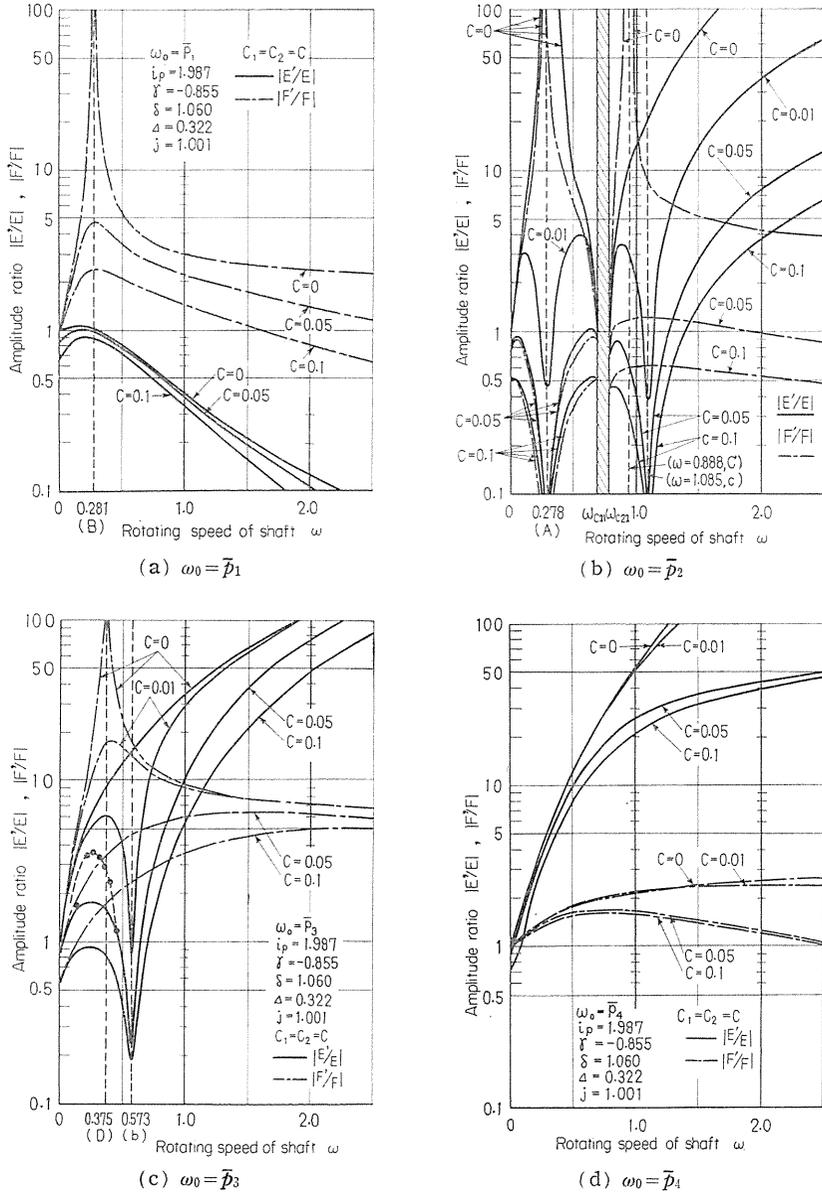
FIG. 4.6. Amplitude ratio-rotating speed  $\omega$  diagrams (experiment B, case II of  $\omega_0 = \bar{p}_i$ )
