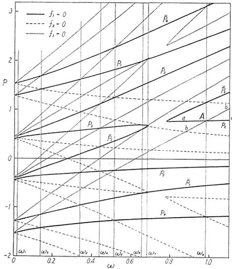
FIG. 5.4  $p-\omega$  curves ( $a:b=1:4$ ,  $\varepsilon \approx 0$ ,  $i_p=1.987$ ,  $\Delta=0.322$ ,  $r=-0.860$ ,  $\delta=1.040$ )
