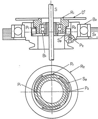
FIG. 4.10. Centrifugal exciter (experiment B)
