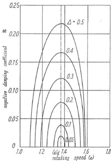
FIG. 6.6. Negative damping coefficient  $m$  ( $i_p=1$ ,  $\delta=1.060$ ,  $\gamma^2=0.731$ ,  $\omega_\alpha=1.3674$ )
