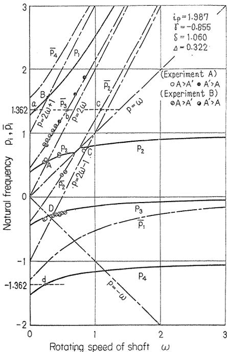
FIG. 4.1. Natural frequency-rotating speed  $\omega$  diagram ( $\omega = 0.683 \sim 0.778$ : unstable region)
