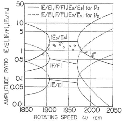
FIG. 7.4. Amplitude ratio of free vibrations near  $\omega_s$  (I-#1200)
