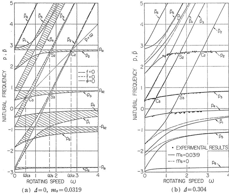
FIG. 7.2. Natural frequency  $p, \bar{p}$  (Experiment I)
