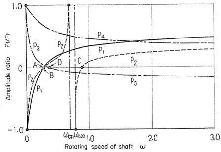
(b) Free vibrations of inclination angles  $\theta_x, \theta_y$
