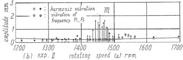
FIG. 6.10. Response curves and negative damping coefficient (experiment I, II)
