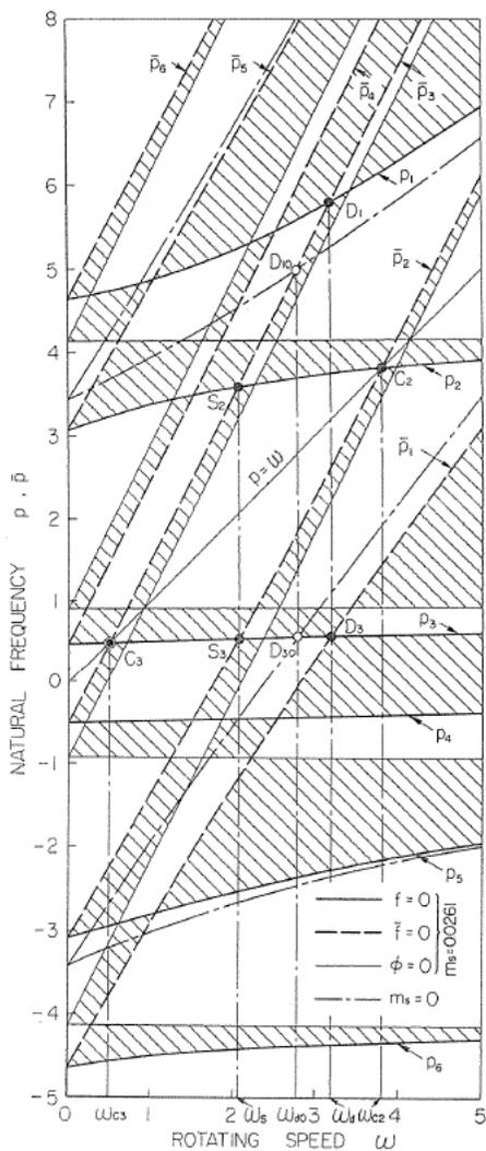
FIG. 7.10. Natural frequency  $p, \bar{p}$  (experiment II,  $\Delta=0$ ,  $m_s=0.0261$ )
