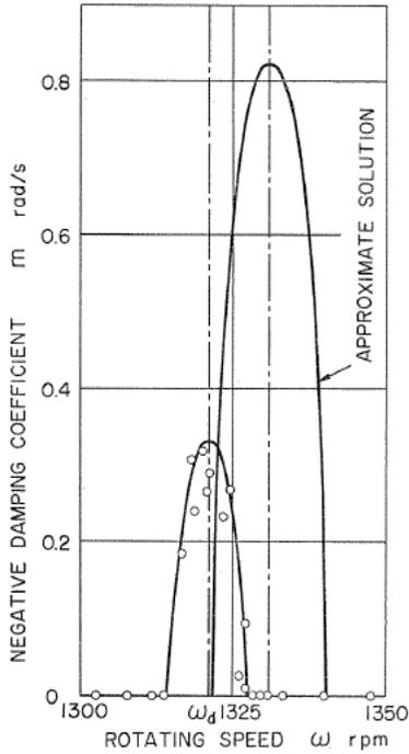
FIG. 8.2. Unstable region near  $\omega_d$
