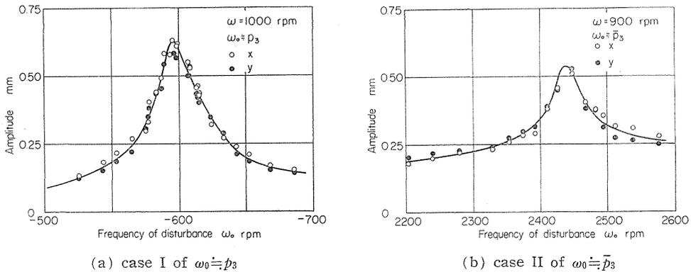
FIG. 4.11. Response curves (experiment B)
