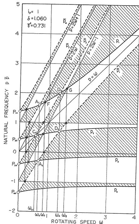
FIG. 6.1.  $p-\omega$  diagram when  $\Delta = 0$ ,
