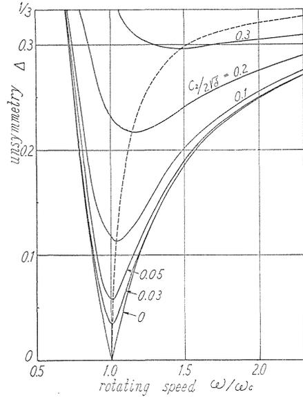
FIG. 3.8. Damping effect on unstable region  $[\omega_{c11}, \omega_{c12}]$
