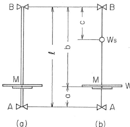
FIG. 7.1. Schematic diagram of shaft system when a mass of shaft is considered
