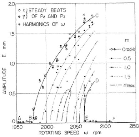
FIG. 7.6.  $E, m-\omega$  diagram (I-#6200)
