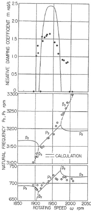
FIG. 7.3.  $m, P_2, P_3-\omega$  diagram near  $\omega_s$  (I-#1200)
