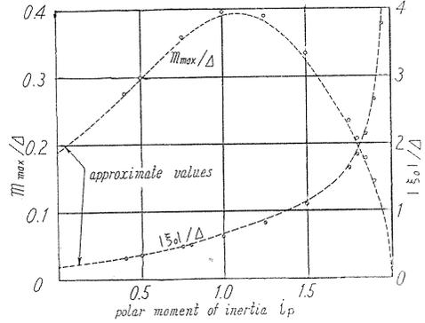
FIG. 6.8. Effects of polar moment of inertia  $i_p$  on  $m_{\max}$  and  $2|\xi_0|$  ( $\delta = 1.060$ ,  $r^2 = 0.731$ )
