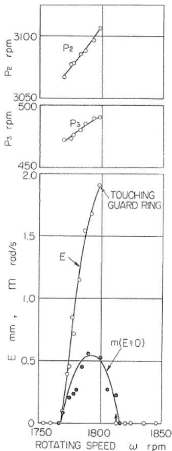
FIG. 7.11.  $P_2, P_3, m, E-\omega$  diagram near  $\omega_s$  (II-#6200) [Angular clearances of ball bearings:  $0.5^\circ$  (upper),  $0.4^\circ$  (lower)]
