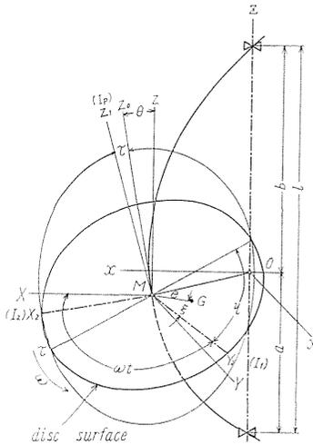
FIG. 3.1. Angular positions of  $\xi, \eta$
