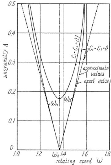
FIG. 6.4. Unstable region near  $\omega_r$  ( $i_p=1$ ,  $\delta=1.060$ ,  $\gamma^2=0.731$ ,  $\omega_\alpha=1.3674$ ,  $|\xi_0|/\Delta=0.6667$ ,  $m_{\max}/\Delta=0.3896$ )
