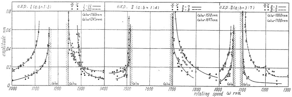
FIG. 2.5. Response curves near  $\omega_{c21}$ ,  $\omega_{c22}$
