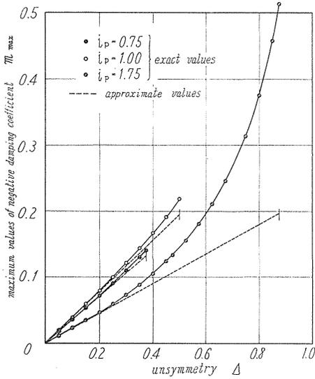
FIG. 6.7.  $m_{\max} - \Delta$  diagram ( $\delta = 1.060$ ,  $r^2 = 0.731$ )
