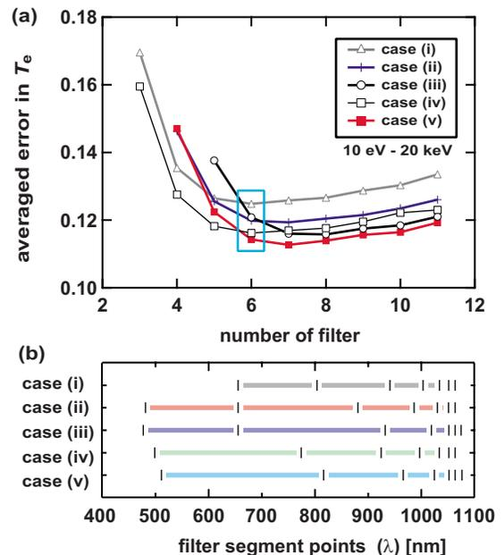
FIG. 3. (Color online) (a) Averaged error in temperature of five different filter designs, i.e., cases (i)–(v). (b) The optimized filter segment points of cases (i)–(v).
