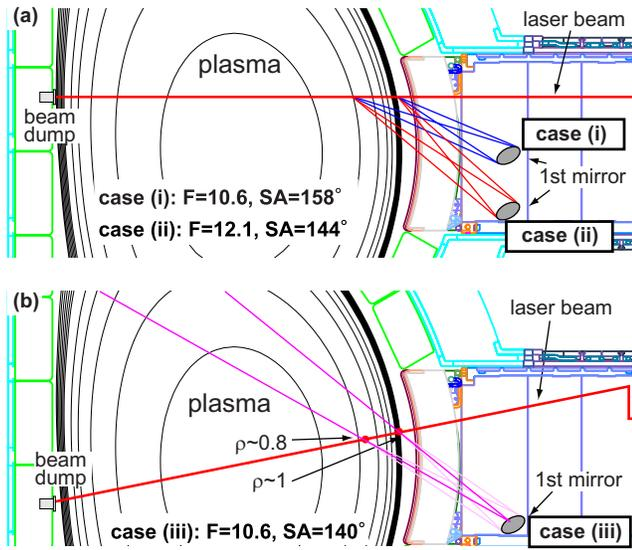
FIG. 1. (Color online) Illustrations of the ITER edge Thomson scattering measurement system in the midplane port (a) shows the case when the laser is injected horizontally, while (b) shows the case when the laser is injected diagonally.
