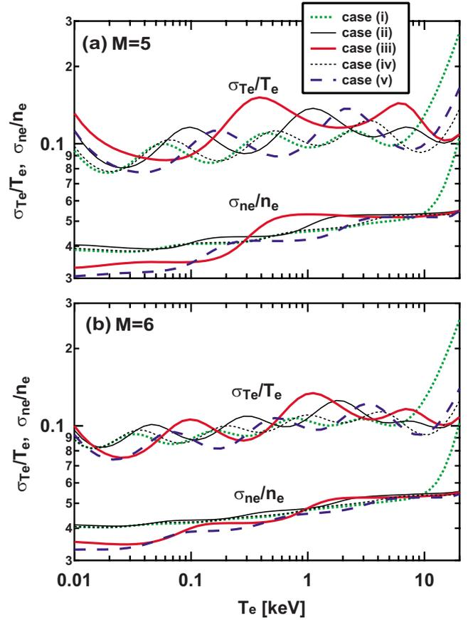
FIG. 4. (Color online) Temperature dependences of the relative estimated errors in  $T_e$  and  $n_e$  for (a)  $M=5$  and (b)  $M=6$  in the five cases (i)–(v) presented in Fig. 3.
