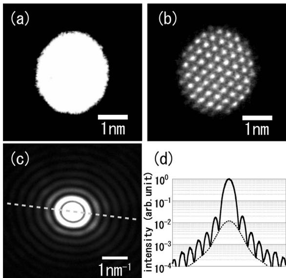
FIG. 1. TEM images of the aperture hole produced by FIB, which are selecting areas in vacuum (a) and in a silicon crystal (b). (c) SAND pattern corresponding to (a). (d) Intensity profile along the dotted line in (c).
