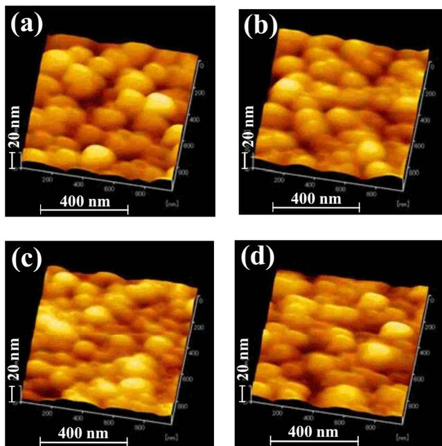
FIG. 2. (Color online) AFM images of the  $(1-x)\text{BiFeO}_3-x\text{PbTiO}_3$  (BF-100xPT) thin films on Pt/TiO<sub>x</sub>/SiO<sub>2</sub>/Si substrates after heat treatment at 600 °C. (a) BF-20PT, (b) BF-30PT, (c) BF-40PT, and (d) BF-50PT.
