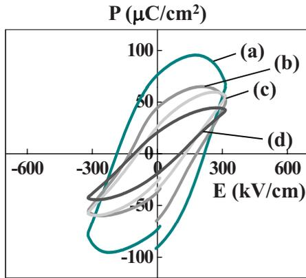
FIG. 4. (Color online)  $P$ - $E$  hysteresis loops of the  $(1-x)\text{BiFeO}_3-x\text{PbTiO}_3$  (BF-100 $x$ PT) thin films on Pt/TiO $_x$ /SiO $_2$ /Si substrates after heat treatment at 600 °C (measured at room temperature). (a) BF-20PT, (b) BF-30PT, (c) BF-40PT, and (d) BF-50PT.
