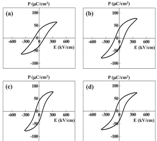
FIG. 9.  $P$ - $E$  hysteresis loops of the 5 mol % Mn-doped  $(1-x)\text{BiFeO}_3\text{-}x\text{PbTiO}_3$  (BF-100xPT) thin films on Pt/TiO<sub>x</sub>/SiO<sub>2</sub>/Si substrates after heat treatment at 600 °C (measured at room temperature). (a) BF-20PT, (b) BF-30PT, (c) BF-40PT, and (d) BF-50PT.
