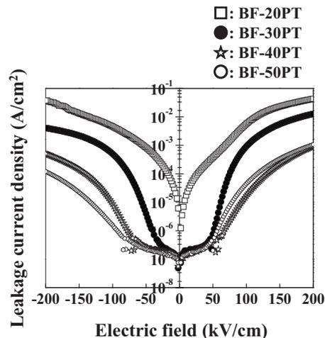
FIG. 3. The leakage current density of the  $(1-x)\text{BiFeO}_3-x\text{PbTiO}_3$  (BF-100xPT) thin films on Pt/TiO<sub>x</sub>/SiO<sub>2</sub>/Si substrates after heat treatment at 600 °C (measured at room temperature). (a) BF-20PT, (b) BF-30PT, (c) BF-40PT, and (d) BF-50PT.
