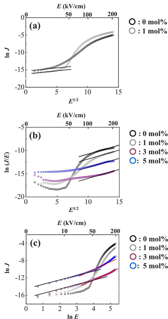
FIG. 7. (Color online) (a)  $\ln J$  vs  $E^{1/2}$ , (b)  $\ln(J/E)$  vs  $E^{1/2}$ , and (c) double logarithm plots for the Mn-doped  $0.7\text{BiFeO}_3\text{-}0.3\text{PbTiO}_3$  thin films on  $\text{Pt}/\text{TiO}_x/\text{SiO}_2/\text{Si}$  substrates after heat treatment at  $600^\circ\text{C}$  (measured at room temperature).
