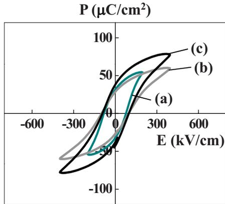
FIG. 8. (Color online)  $P$ - $E$  hysteresis loops of the Mn-doped  $0.7\text{BiFeO}_3\text{-}0.3\text{PbTiO}_3$  thin films on Pt/TiO<sub>x</sub>/SiO<sub>2</sub>/Si substrates after heat treatment at 600 °C (measured at room temperature). Mn content: (a) 1 mol %, (c) 3 mol %, and (d) 5 mol %.
