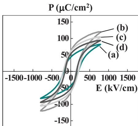
FIG. 10. (Color online)  $P$ - $E$  hysteresis loops of the 5 mol % Mn-doped  $(1-x)\text{BiFeO}_3-x\text{PbTiO}_3$  (BF-100xPT) thin films on Pt/TiO<sub>x</sub>/SiO<sub>2</sub>/Si substrates after heat treatment at 600 °C (measured at -190 °C). (a) BF-20PT, (b) BF-30PT, (c) BF-40PT, and (d) BF-50PT.
