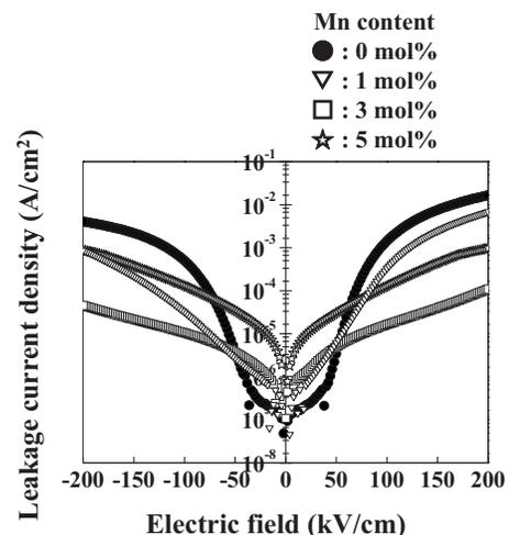
FIG. 6. The leakage current density of the Mn-doped 0.7BiFeO $_3$ -0.3PbTiO $_3$  thin films on Pt/TiO $_x$ /SiO $_2$ /Si substrates after heat treatment at 600 °C (measured at room temperature). Mn content: (a) 0 mol %, (b) 1 mol %, (c) 3 mol %, and (d) 5 mol %.
