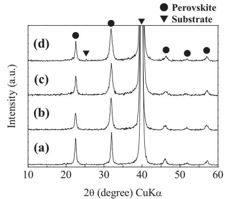
FIG. 1. XRD patterns of the  $(1-x)\text{BiFeO}_3\text{-}x\text{PbTiO}_3$  (BF-100xPT) thin films on  $\text{Pt/TiO}_x/\text{SiO}_2/\text{Si}$  substrates after heat treatment at 600 °C. (a) BF-20PT, (b) BF-30PT, (c) BF-40PT, and (d) BF-50PT.
