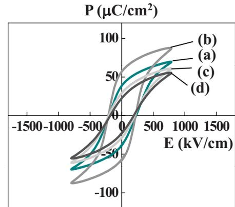
FIG. 5. (Color online)  $P$ - $E$  hysteresis loops of the  $(1-x)\text{BiFeO}_3-x\text{PbTiO}_3$  (BF-100 $x$ PT) thin films on Pt/TiO $_x$ /SiO $_2$ /Si substrates after heat treatment at 600 °C (measured at -190 °C). (a) BF-20PT, (b) BF-30PT, (c) BF-40PT, and (d) BF-50PT.
