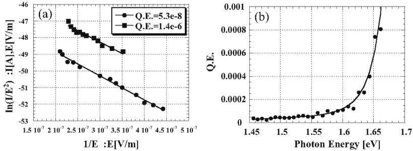
**FIGURE 3.** (a) F-N plot of photo-electron extracted from tip-GaAs, (b) QE of tip-GaAs under applying high gradient field as a function of excitation photon energy.
