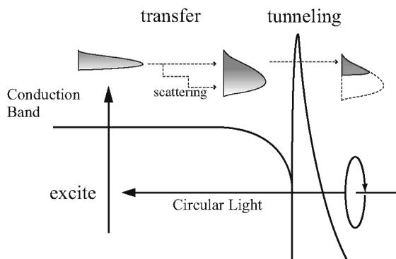
**FIGURE 5.** Schematic of one-dimensional potential model of field emission in p-doped semiconductor. The magnitude of polarization is indicated by the light and shaded regions under the energy distribution curve, where darker shades correspond to higher polarization.
