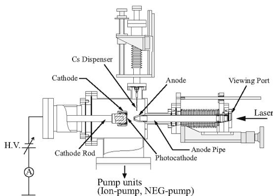
**FIGURE 2.** Schematic of 20-kV DC gun.
