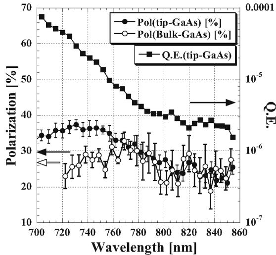
**FIGURE 4.** ESP and QE of tip-GaAs as a function of wavelength.
