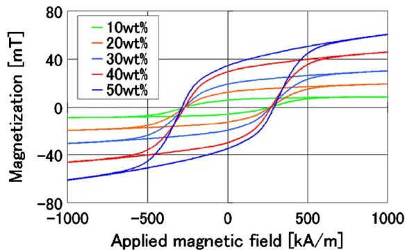
FIG. 4. (Color online) Magnetic characteristics of MPC polymers with different magnetic particle concentrations.
