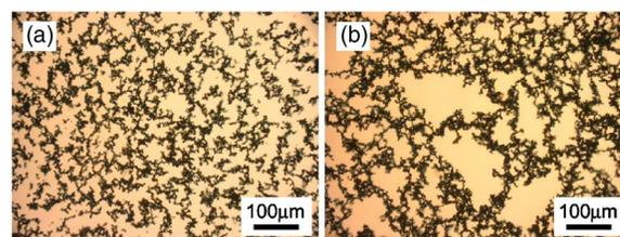
FIG. 1. (Color online) Dispersion of the magnetic particles in liquid photocurable polymer matrix without additives (a) immediately after mixing and (b) 1 h later.
