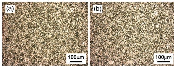
FIG. 2. (Color online) Dispersion of the magnetic particles in a liquid photocurable polymer matrix with the viscosity-increasing agent (a) immediately after mixing and (b) 1 h later.
