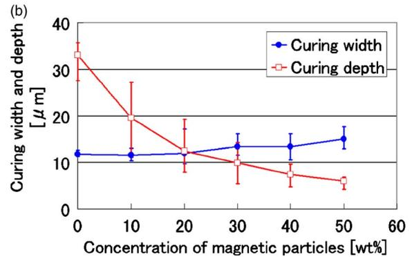
FIG. 3. (Color online) Curing characteristics of MPC polymers. (a) Schematic of sample fabrication. (b) Curing widths and depths of MPC polymers with different magnetic particle concentrations.
