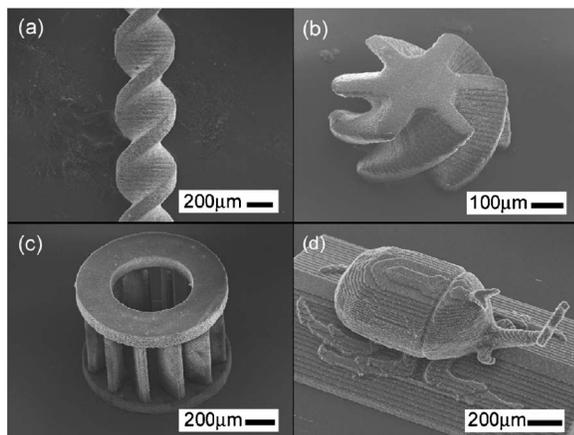
FIG. 5. 3D magnetic microstructures fabricated by microstereolithography: (a) microscrew with a diameter of 500  $\mu\text{m}$ , height of 2 mm, and spiral pitch of 1 mm; (b) microfan with a diameter of 500  $\mu\text{m}$  and height of 250  $\mu\text{m}$ ; (c) microsirocco fan with a diameter of 1 mm and height of 700  $\mu\text{m}$ ; (d) microsculpture (beetle) with a length of 2 mm, width of 1 mm, and height of 660  $\mu\text{m}$ .
