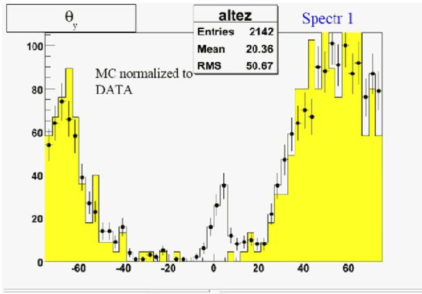
**FIGURE 4.** Dip angle distribution of the tracks recorded. The tracks with the dip angle of  $>20$  degree and  $<-20$  degree are cosmic-rays. A cluster, which can be seen around  $-10$  to  $10$  degree, are the events caused by neutrinos from CERN.
