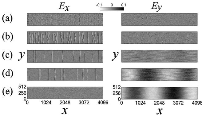
FIG. 1. Spatial profiles of the electric field  $E_x$  and  $E_y$  at different times. (a)  $\omega_{pe}t=50$ , (b)  $\omega_{pe}t=1000$ , (c)  $\omega_{pe}t=4000$ , (d)  $\omega_{pe}t=6000$ , and (e)  $\omega_{pe}t=8000$ . The amplitude is normalized by  $m_e\omega_{pe}V_d/e$ , and the distance is normalized by  $V_{te}/\omega_{pe}$ .
