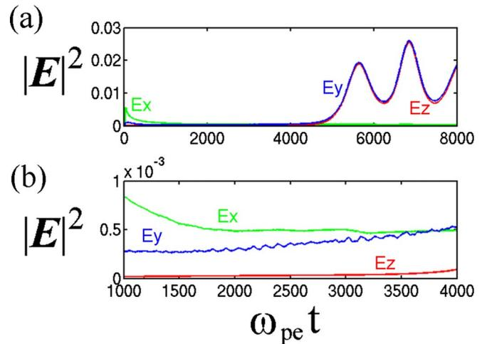
FIG. 2. (Color online) (a) Time history of the electric field energies  $|E_x|^2$ ,  $|E_y|^2$ , and  $|E_z|^2$  normalized by  $m_e^2\omega_{pe}^2V_d^2/e^2$ . (b) Expanded history for  $\omega_{pe}t=1000-4000$ .
