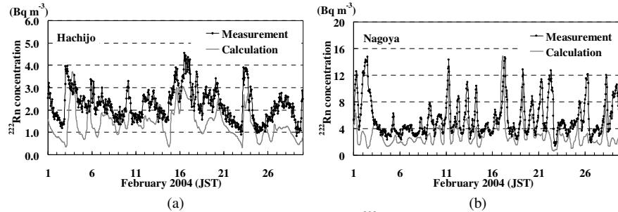
**FIGURE 2.** Comparison of temporal variation in surface  $^{222}\text{Rn}$  concentration between measurement and calculation at Hachijo and Nagoya.
