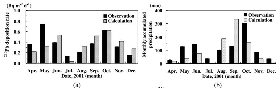
**FIGURE 3.** Comparison of monthly accumulated in  $^{210}\text{Pb}$  deposition and precipitation between observation and calculation.
