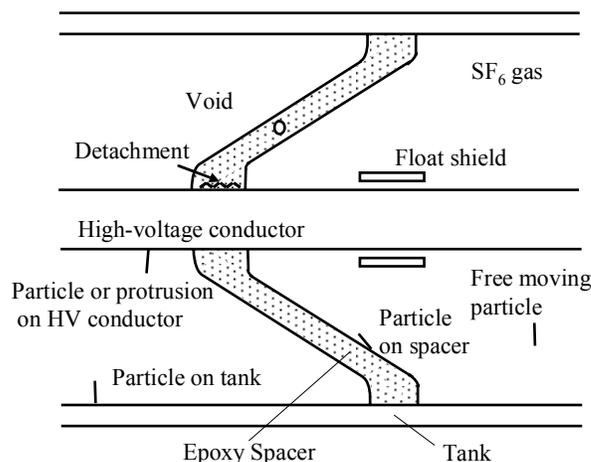
Fig. 1. Example of possible defects in GIS
