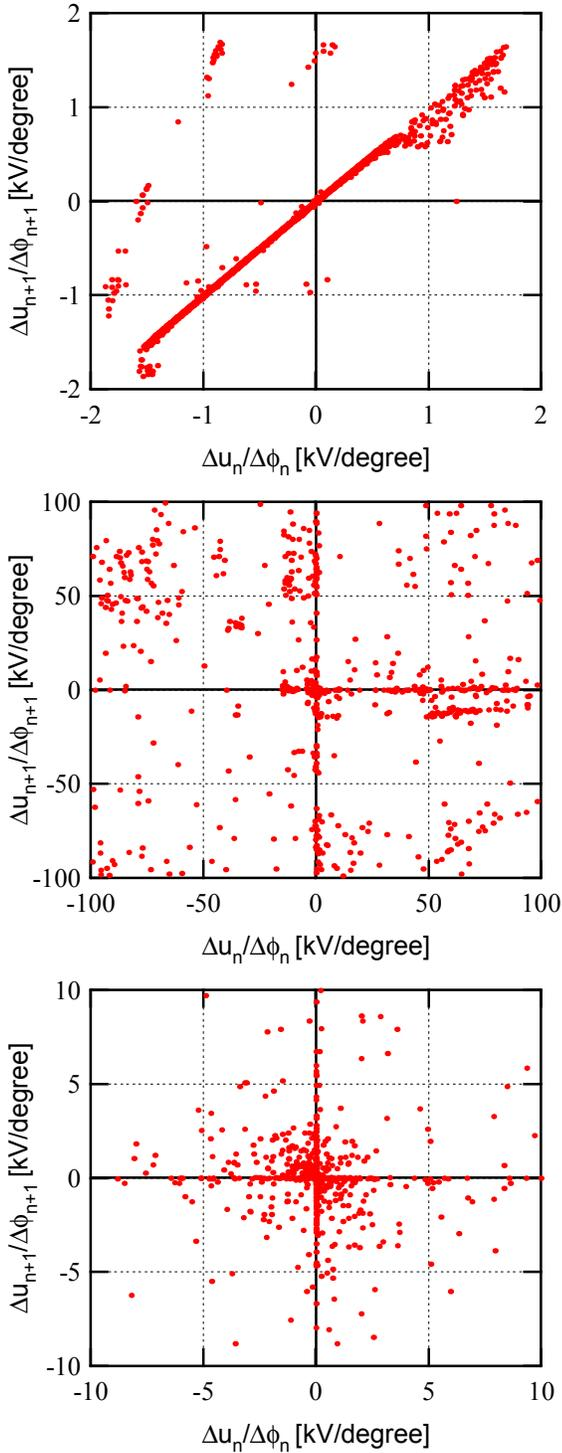
Fig. 7.  $\Delta u / \Delta \phi$  pattern: (a) a particle in a gap. (b) a particle on a spacer. (c) detachment
