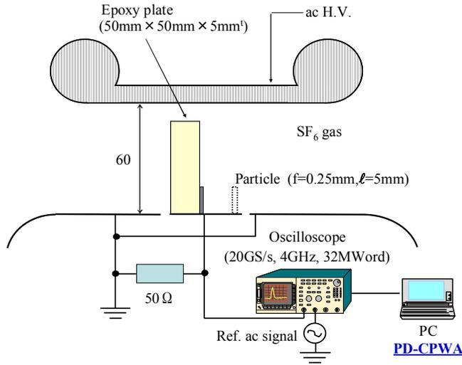
Fig. 2. Electrode setup for metallic particle defects
