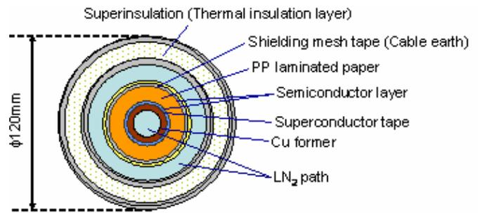
(b) Cross section of 2m HTS cable sample
