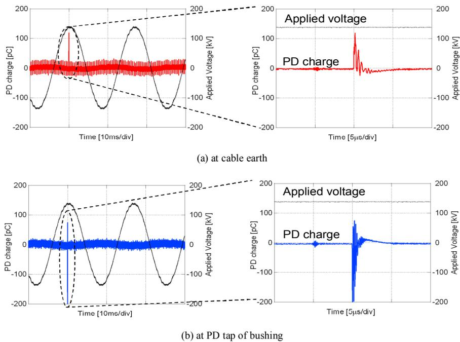
Fig. 4. PD signal waveforms
