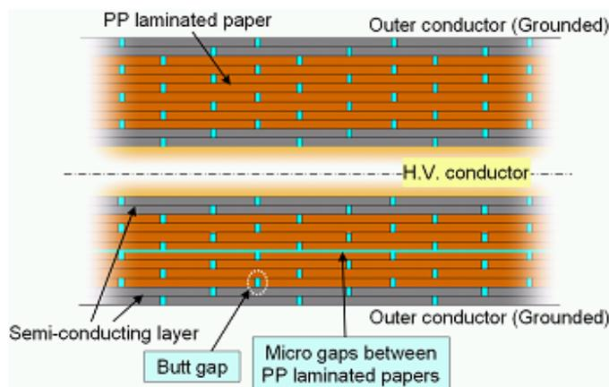
Fig. 1. LN<sub>2</sub>/PP laminated paper composite insulation system
