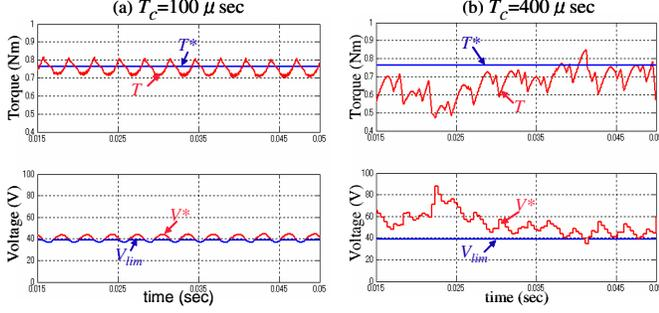
Fig. 10. Simulation results of torque and voltage amplitude when control period are (a)  $100\mu\text{sec}$  and (b)  $400\mu\text{sec}$
