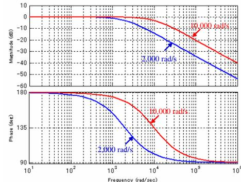
Fig. 5. Bode diagram of  $G_{du}(s)$  when crossover frequencies of PI gain are 2,000 rad/s and 10,000 rad/s in continuous system
