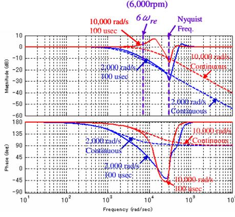
Fig. 7. Bode diagram of  $G_{du}(s)$  when crossover frequencies of PI gain are 2,000 rad/s and 10,000 rad/s in continuous system and 100 $\mu$ sec discrete system
