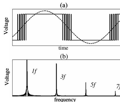
Fig. 2. (a)Waveform of phase voltage in overmodulation range (b)Power spectrum of voltage in overmodulation range
