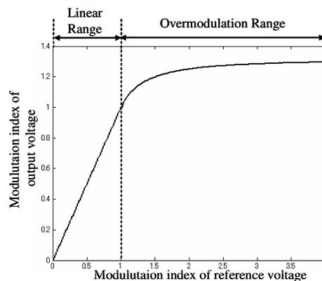
Fig. 1. The nonlinear amplitude relation between reference voltage and output voltage of an inverter
