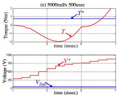
Fig. 37. Simulation results: 5,000 rad/s 500 $\mu$ sec
