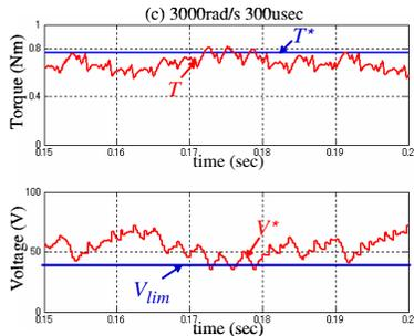
Fig. 25. Simulation results: 3,000 rad/s 300 $\mu$ sec
