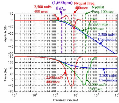
Fig. 9. Bode diagram of  $G_{du}(s)$  when crossover frequencies of PI gain is 2,500 rad/s constant and control periods are 0(continuous), 100 $\mu$ sec and 400 $\mu$ sec
