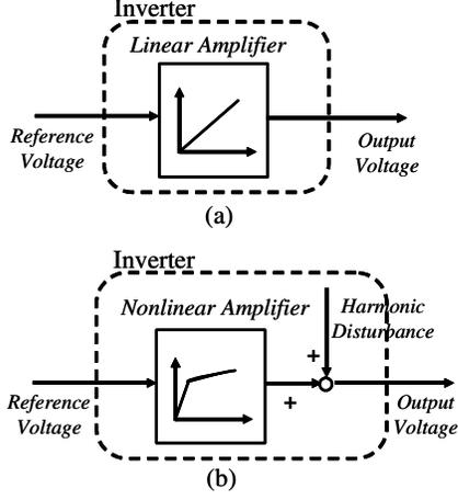
Fig. 3. Model of an inverter in (a) linear range (b) overmodulation range
