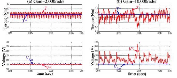
Fig. 8. Simulation results of torque and voltage amplitude when PI gains are (a) 2,000 rad/s and (b) 10,000 rad/s
