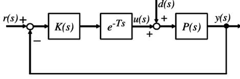
Fig. 6. Block diagram of discrete PMSM current control loop
