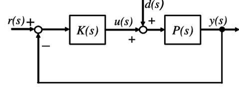
Fig. 4. Block diagram of continuous PMSM current control loop
