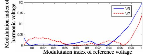
Fig. 11. Relation between modulation index of reference voltage and harmonic voltages
