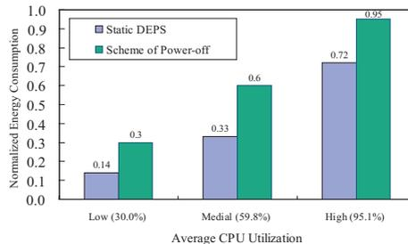
Fig. 3. Normalized energy consumption at different CPU utilizations.
