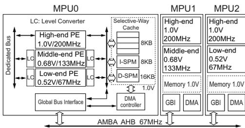
Fig. 4. Prototype of multi-performance processor [10].
