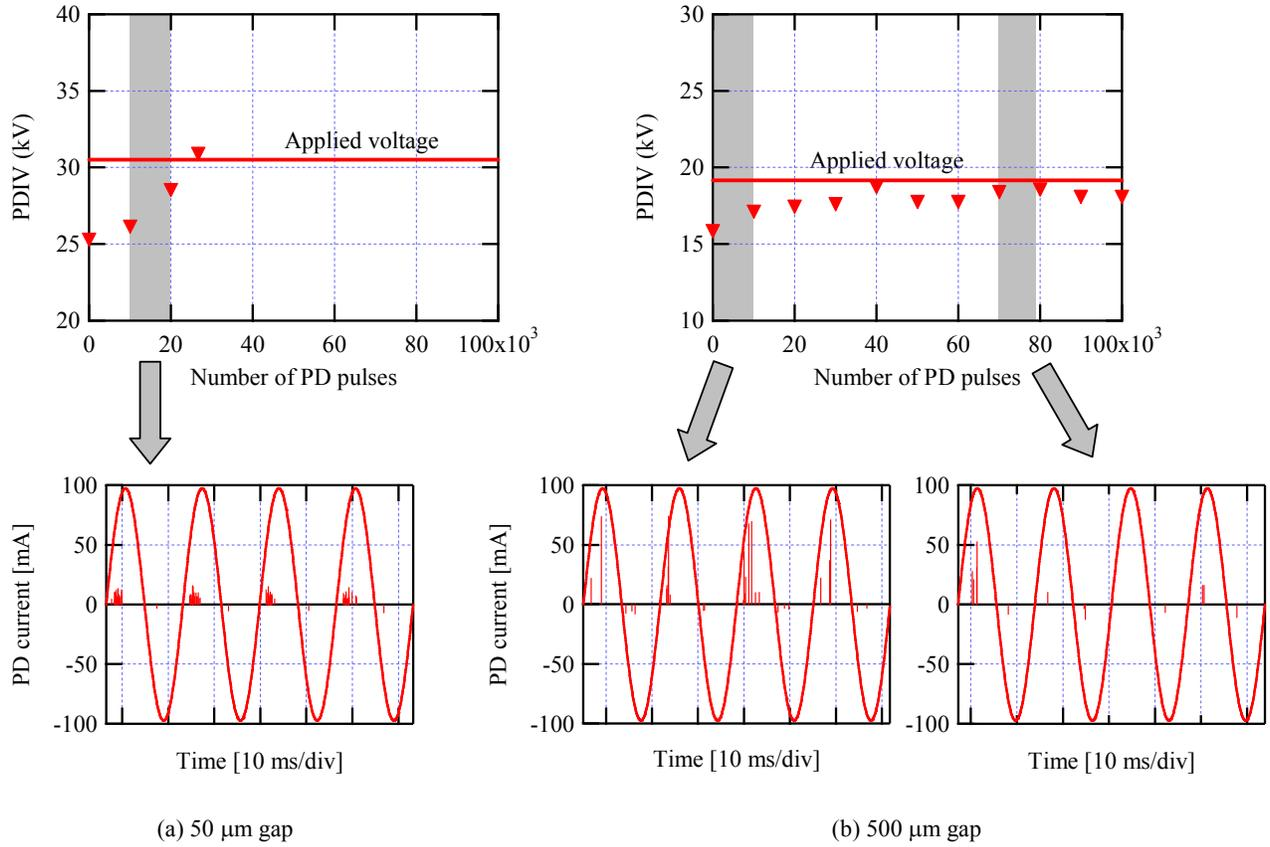
Fig. 3. Dependence of PDIE on successive PD exposure of epoxy samples for small and large gaps
