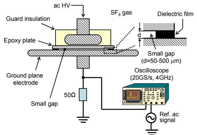
Fig. 1. Schematic diagram for simulating small gap with electrode/epoxy interface in SF<sub>6</sub> gas
