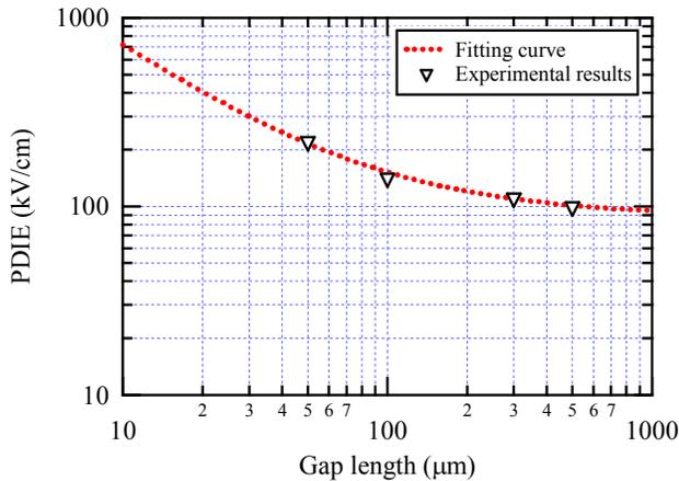
Fig. 2. Experimental PDIE results and its fitting curve corresponding to breakdown field strength in  $\text{SF}_6$  gas
