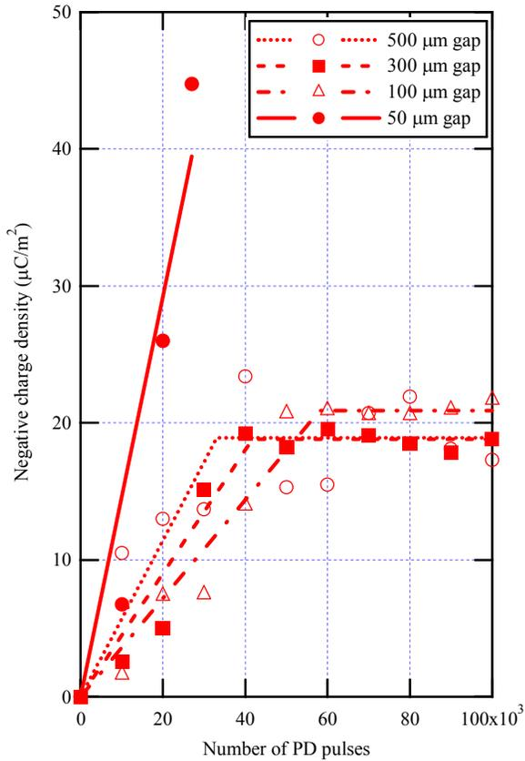
Fig. 4. Accumulated charge density as a function of PD pulses for different gap lengths
