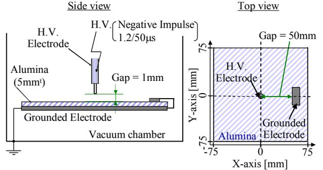
Fig. 4. Electrode configuration (for surface discharge generation).
