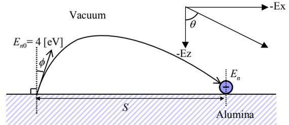
Fig. 9. Schematic model of secondary electron orbit.
