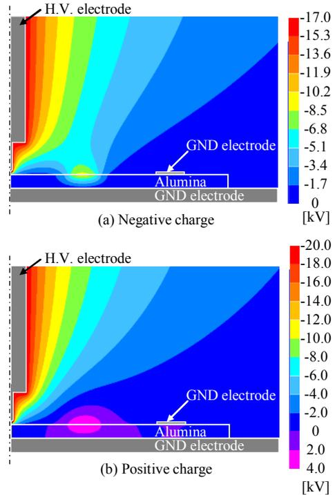
Fig. 10. Equi-potential distribution with surface charge (Case B).
