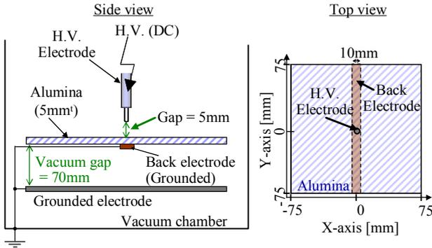
Fig. 2. Electrode configuration (for surface charge generation).
