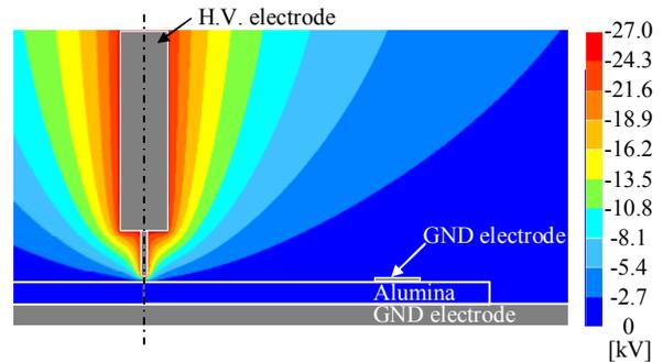
Fig. 5. Equi-potential distribution without surface charge.
