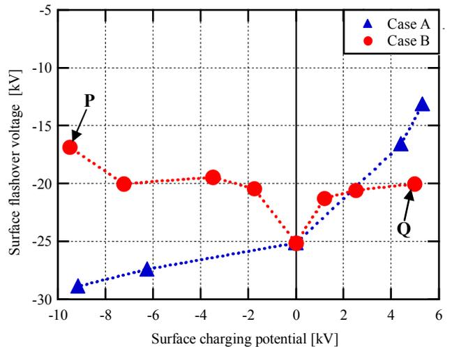
Fig. 7. Influence of surface charging potential on surface flashover voltage.
