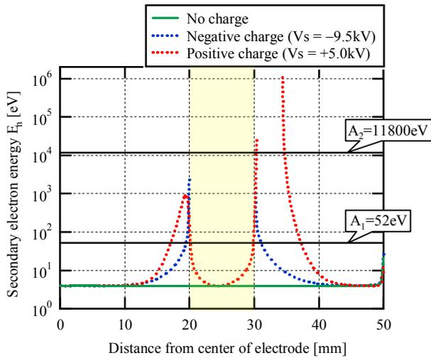
Fig. 13. Secondary electron energy at collision against alumina surface.
