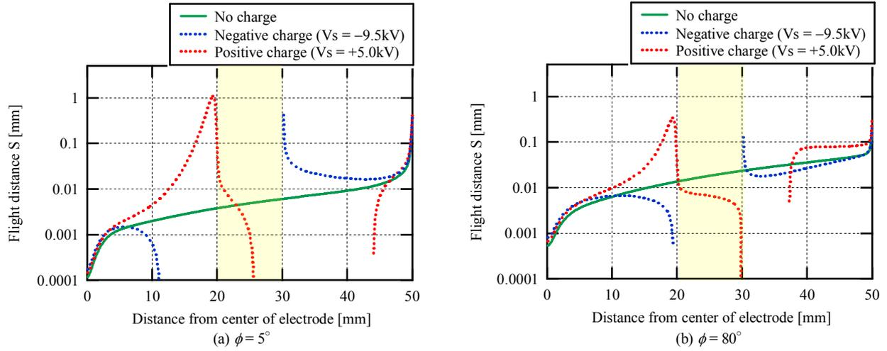
Fig. 12. Flight distance of secondary electron.
