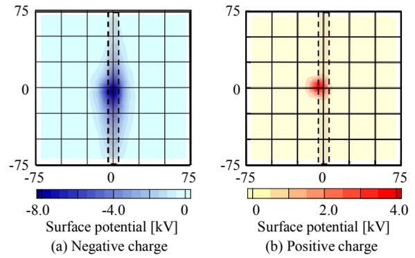
Fig. 3. Positive and negative 2-D surface potential distribution.
