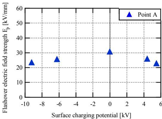
Fig. 8. Relationship between surface charging potential and electric field strength.
