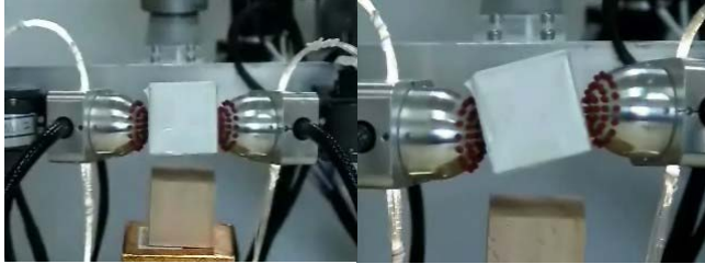
Figure 8. Verification experiment of robotic fingers manipulate paper box.
