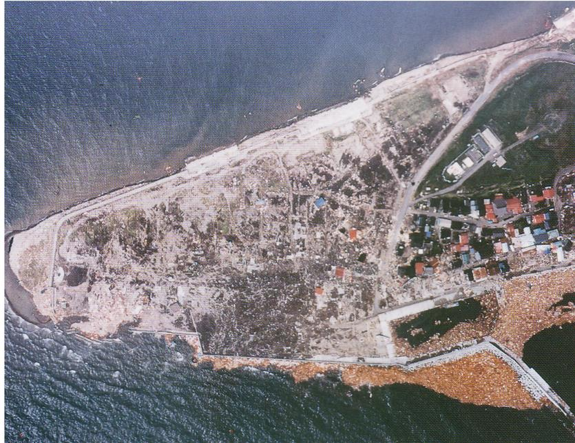
Photo 1.2 Damage on Okushiri island by Hokkaido Nanseioki earthquake tsunami in 1993
