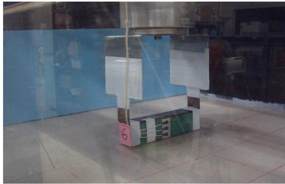
Photo 2.1 Container fixed by 6-component force transducers
