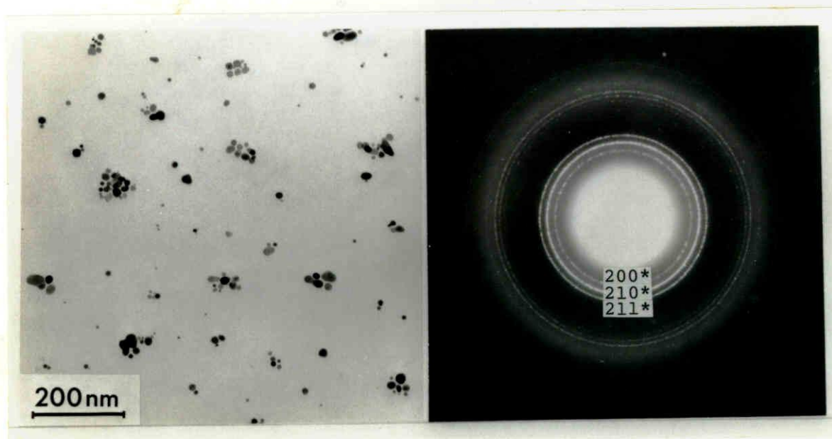
Fig. I-14. (a) Cr particles grown in the outside region of the outer zone. T = 2000^{\circ}\text{C} , p = 30 Torr and D = 5 cm. (b) Debye pattern, showing only \delta -Cr.
