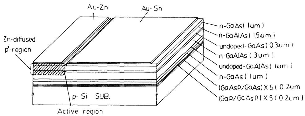
Fig. 4.7 Schematic illustration of the TJS LD on Si.
