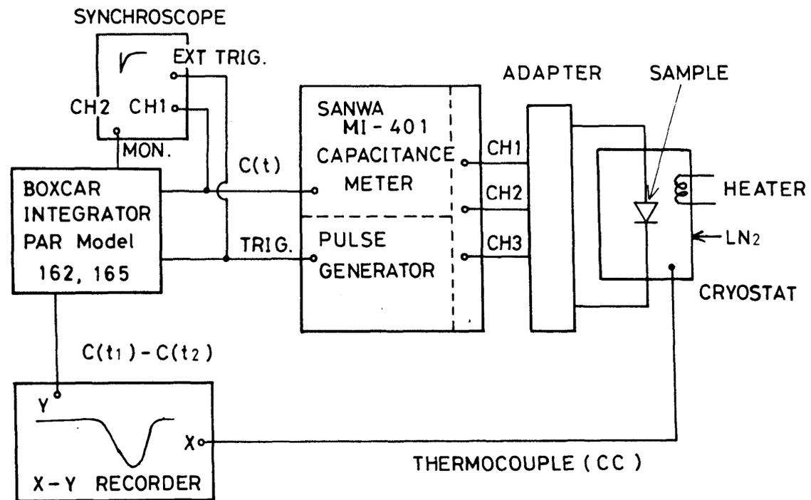
Fig. 3.19 DLTS measurement system.
