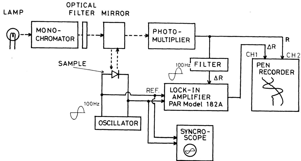
Fig. 3.12 Electroreflectance measurement system.
