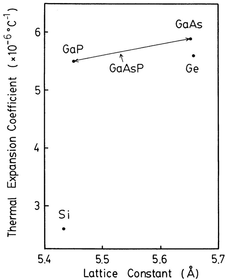
Fig.1.1 Lattice constants and thermal expansion coefficients of semiconductors.
