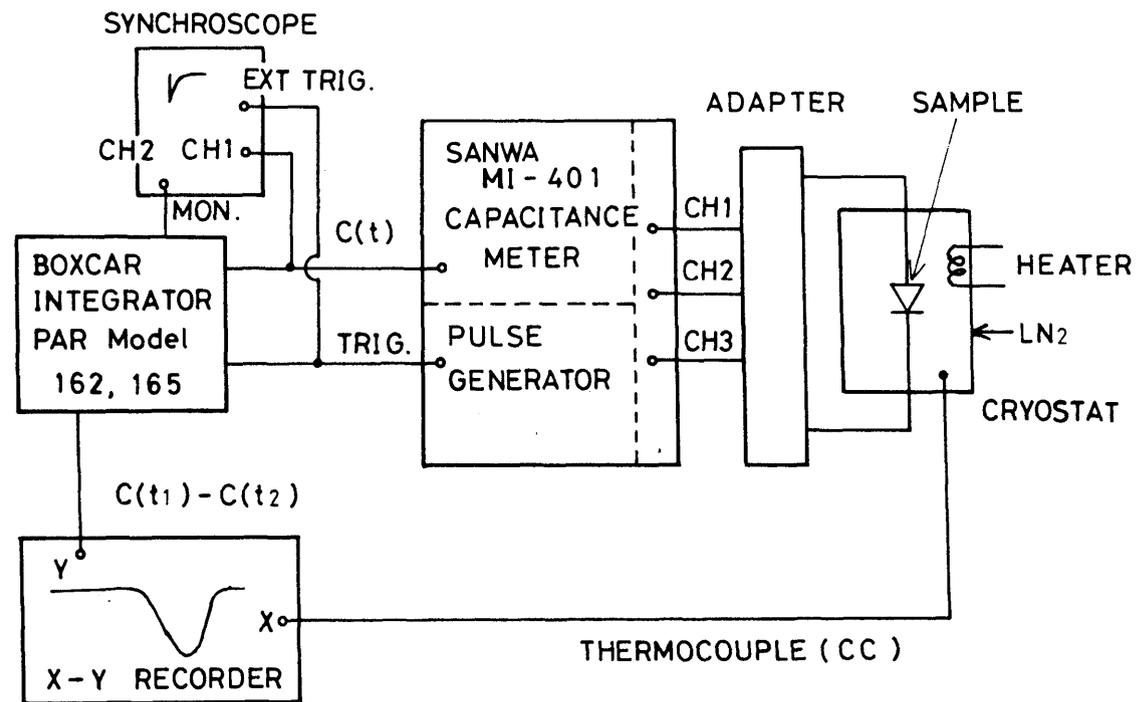
Fig. 3.19 DLTS measurement system.
