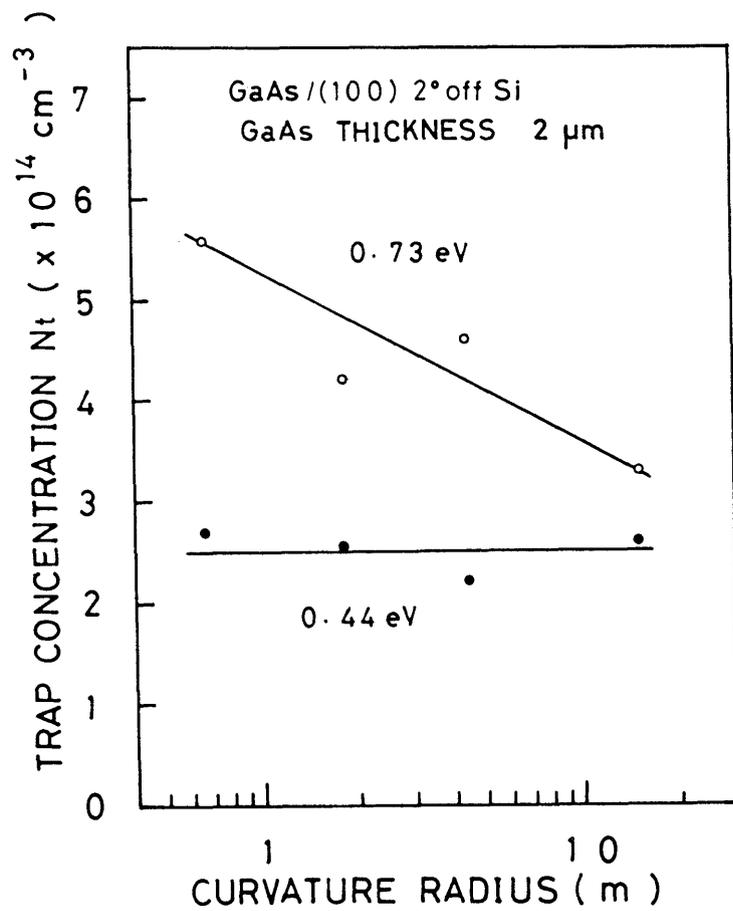
Fig. 3.26 Trap concentration as a function of the curvature radius of the wafer.
