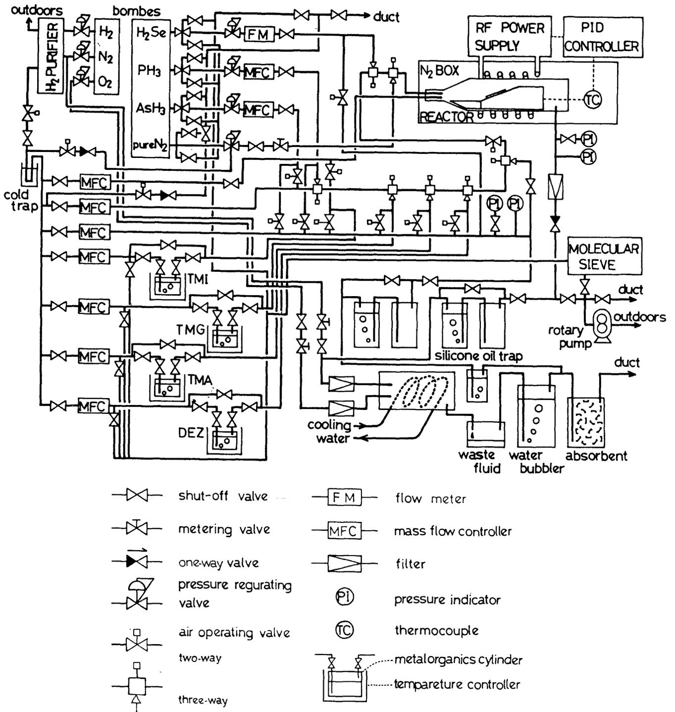
Fig. 2.1 Gas lines of the MOCVD growth apparatus.
