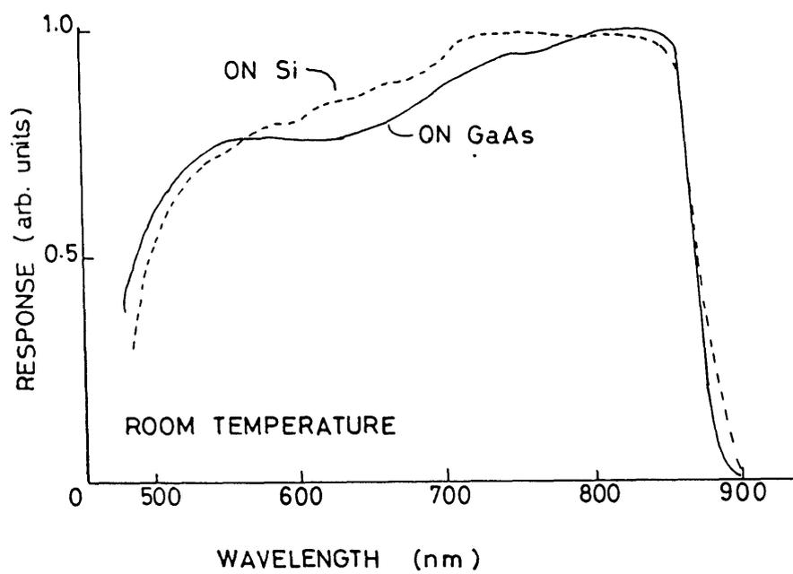
Fig. 3.30 Spectral photo-responses of the diodes grown on GaAs and Si.
