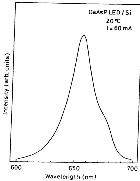
Fig. 5.11 Emission spectrum of  $\text{GaAs}_{0.6}\text{P}_{0.4}$  LED.
