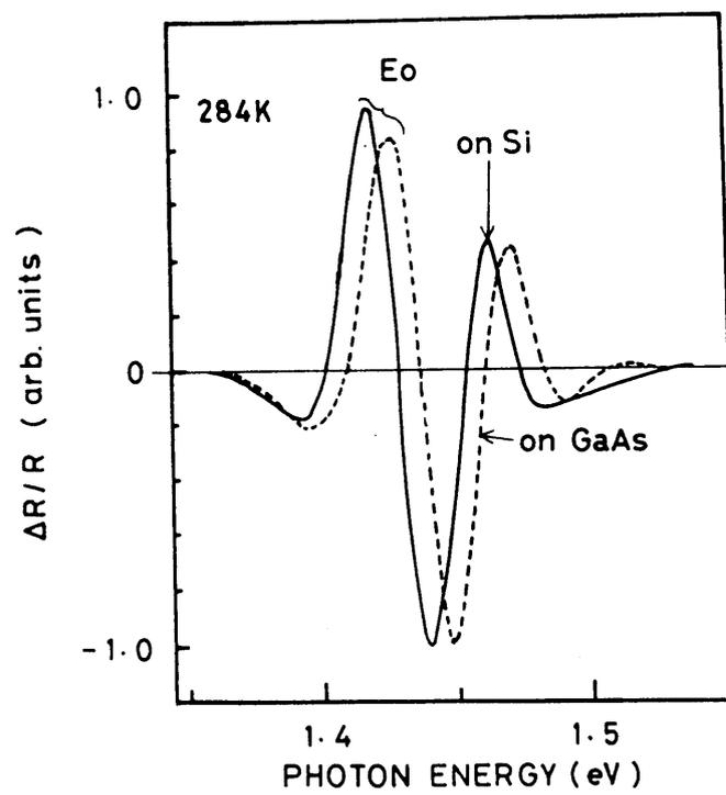
Fig. 3.13 Typical ER spectra of GaAs on Si and GaAs.
