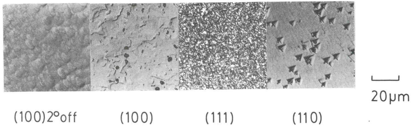
Fig. 2.14 Surface Nomarski micro photographs of GaAs grown at various Si substrate orientations.
