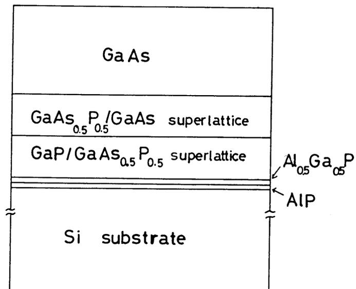
Fig. 2.3 Structure to grow GaAs on Si substrate
