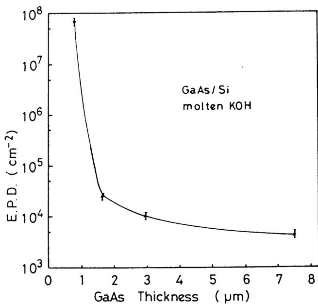
Fig. 3.6 EPD as a function of GaAs thickness.
