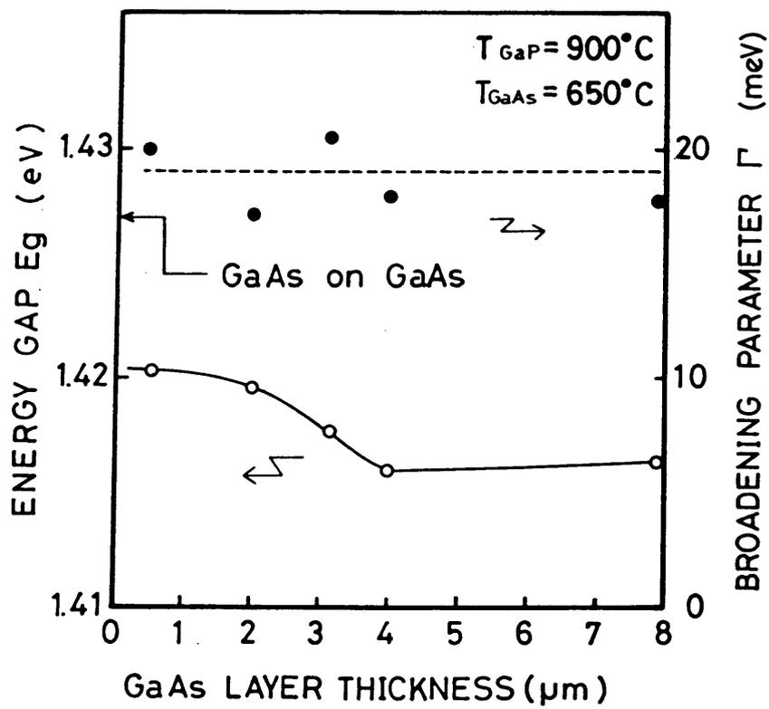
Fig. 3.14 Band gap energy and broadening parameter as a function of GaAs thickness.
