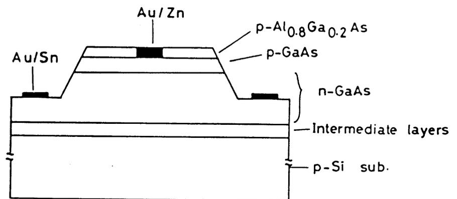
Fig. 3.27 Schematic illustration of the fabricated diodes.
