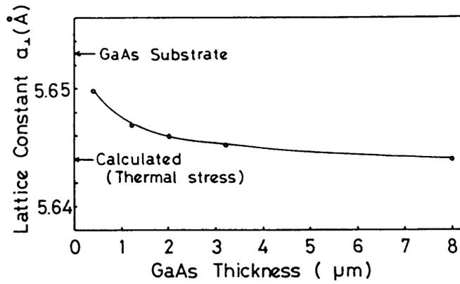
Fig. 3.10 Lattice constant perpendicular to the surface as a function of GaAs thickness.
