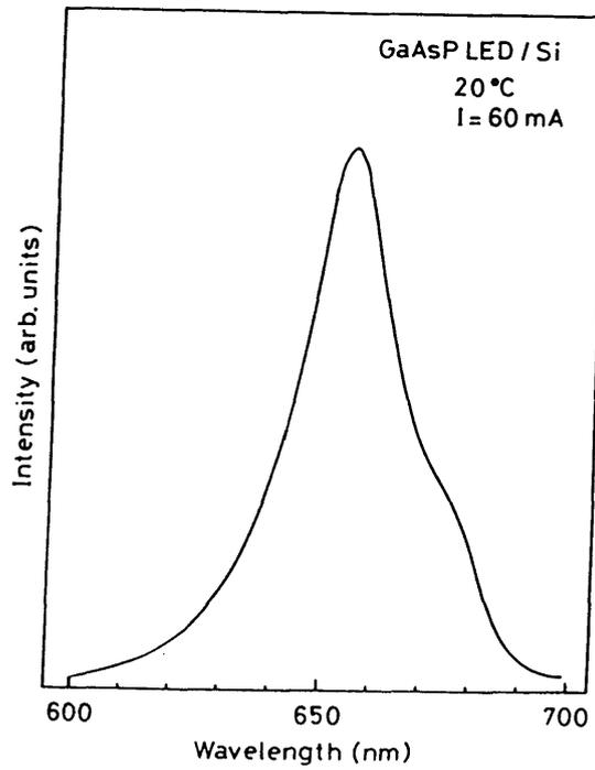
Fig. 5.11 Emission spectrum of  $\text{GaAs}_{0.6}\text{P}_{0.4}$  LED.
