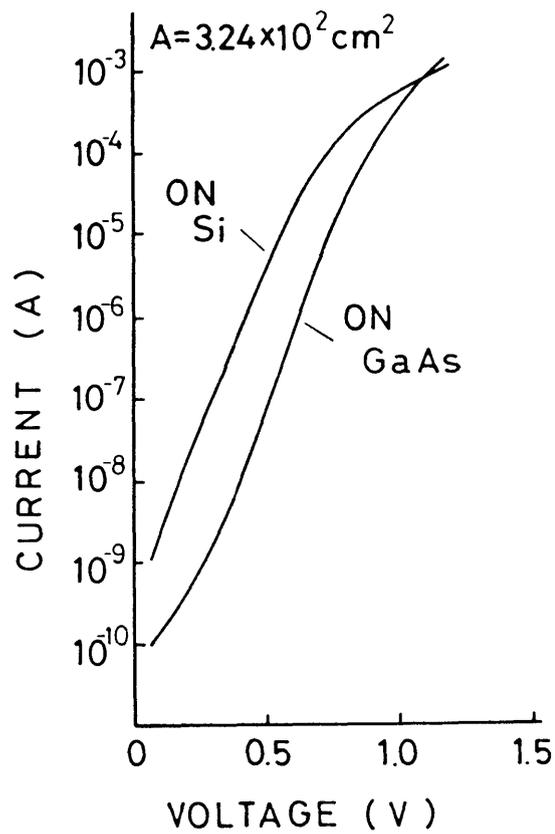
Fig. 3.28 Current voltage characteristics of the diode grown on GaAs and Si.
