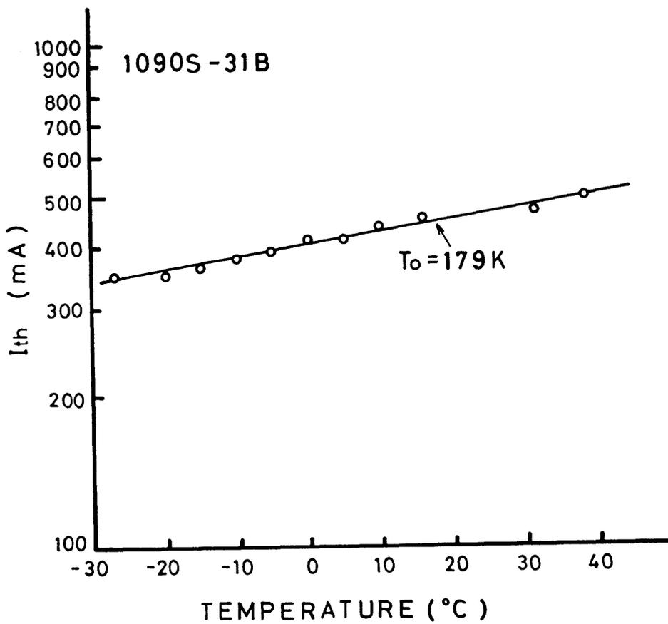
Fig. 4.6 Temperature dependence of the threshold current of the LD.
