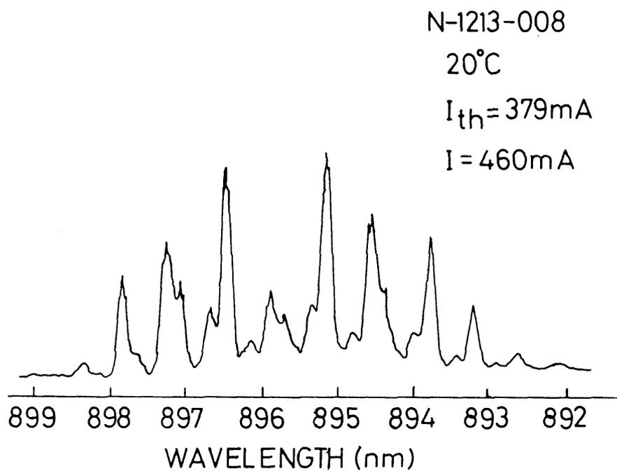
Fig. 4.9 Lasing spectrum of the TJS LD.
