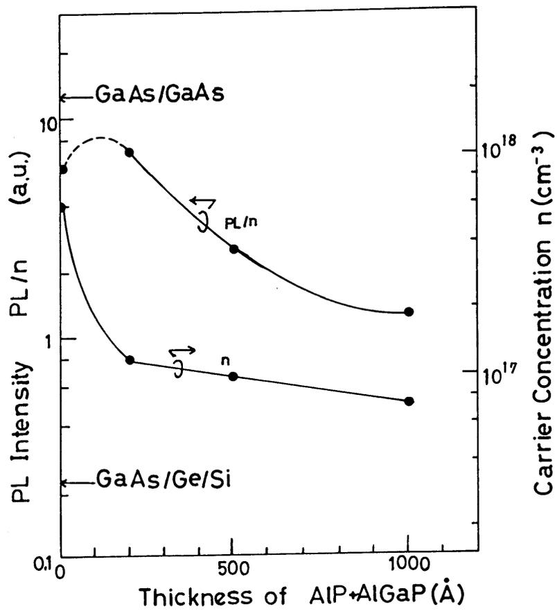
Fig. 2.7 PL intensity and carrier concentration vs. the thickness of AlP + AlGaP.
