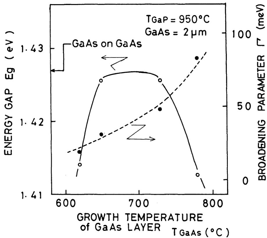
Fig. 3.17 Band gap energy and broadening parameter as a function of  $T_{\text{GaAs}}$ .
