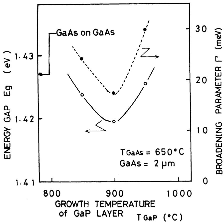
Fig. 3.18 Band gap energy and broadening parameter as a function of  $T_{GaP}$ .
