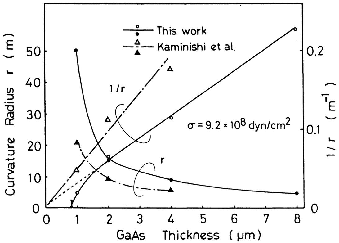
Fig. 3.8 Curvature radius of the wafer and its reciprocal as a function of GaAs thickness.
