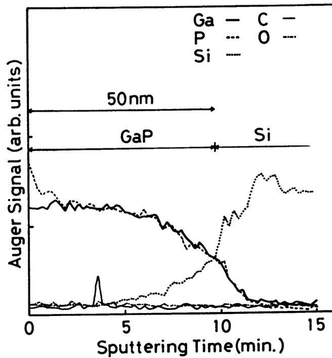
Fig. 3.16 In-depth Auger profile of GaP grown at 900°C.
