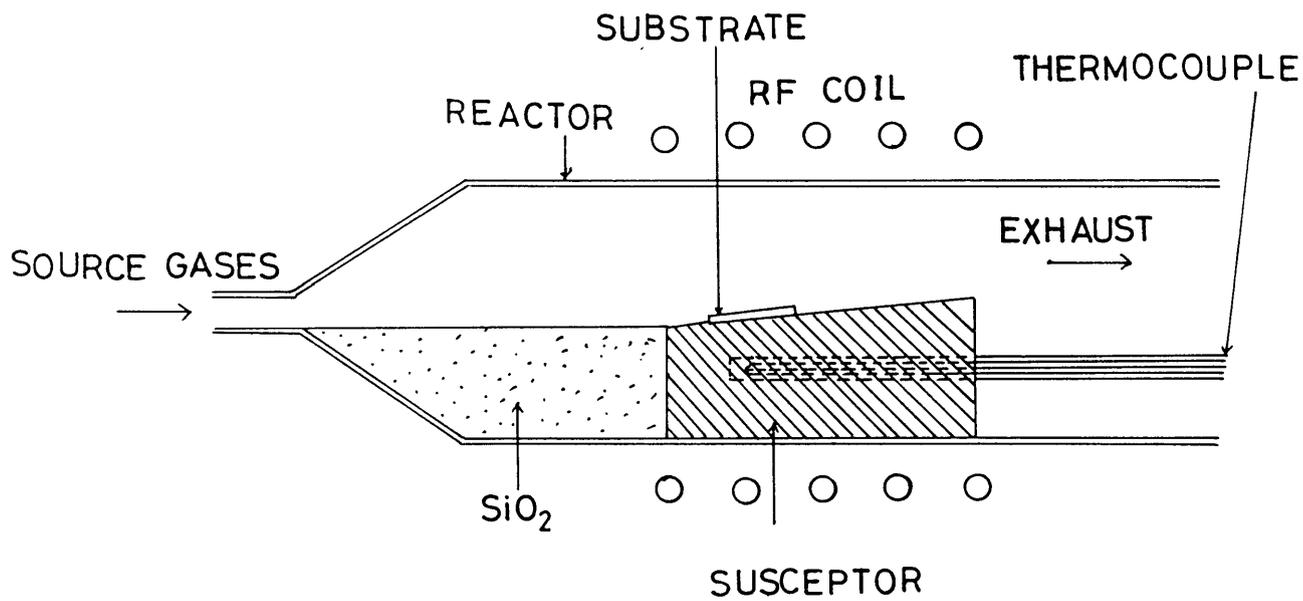
Fig. 2.2 Schematic view of the MOCVD reactor.
