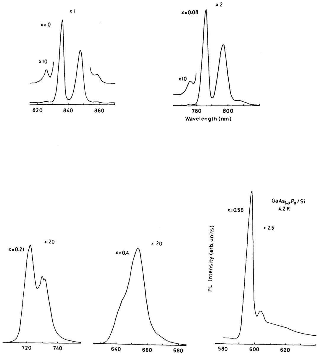
Fig. 5.6 4.2K PL spectra of  $\text{GaAs}_{1-x}\text{P}_x$  ( $x=0-0.56$ )/Si grown at 650 °C.
