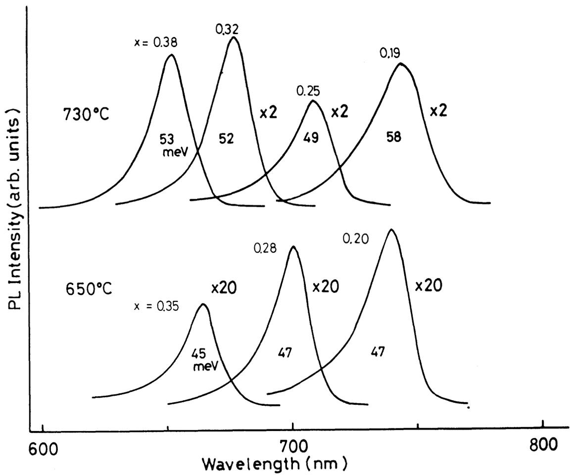
Fig. 5.5 Room temperature PL spectra and half width of GaAs<sub>1-x</sub>P<sub>x</sub> (x=0.2-0.4)/Si grown at 650 and 730 °C.
