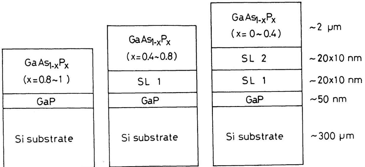
SL 1 : GaP / GaAs<sub>0.5</sub>P<sub>0.5</sub> superlattice
