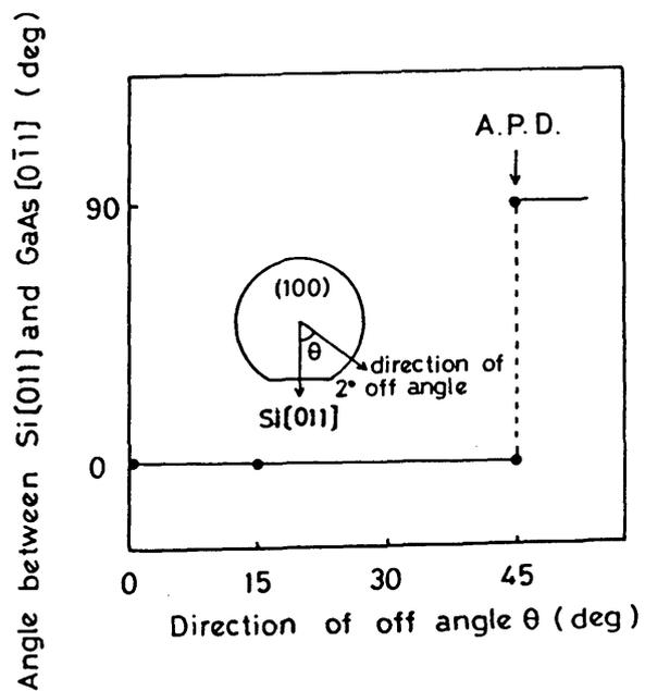
Fig. 3.2 Angle between Si[011] and GaAs[0 $\bar{1}$ 1] vs. direction of off angle.
