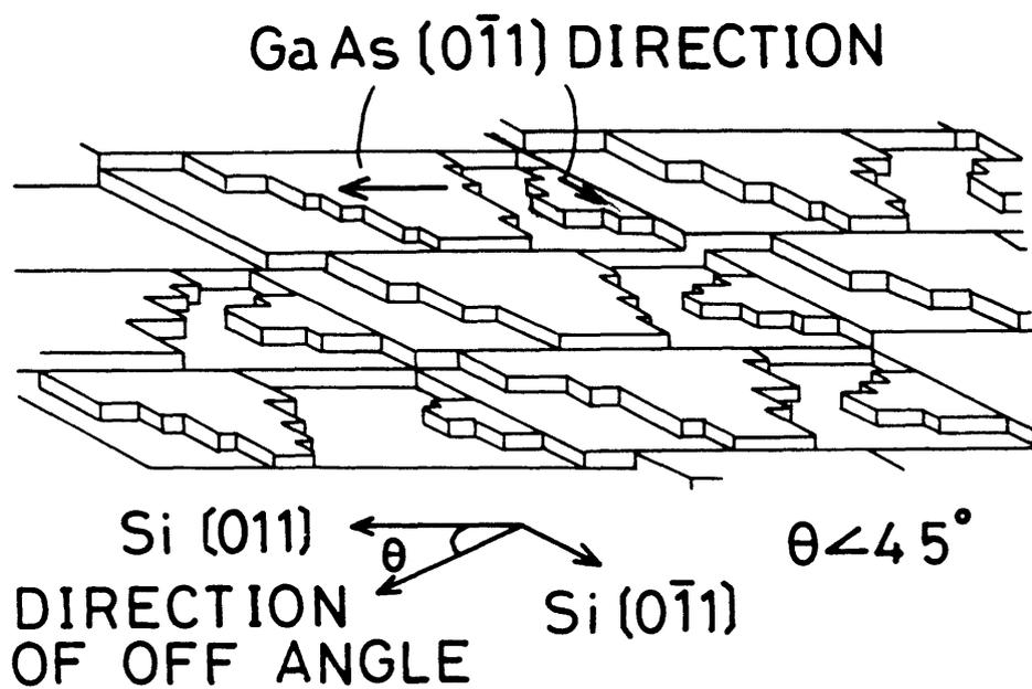
Fig. 3.3 Schematic illustration of GaAs growth on inclined (100) Si surface.
