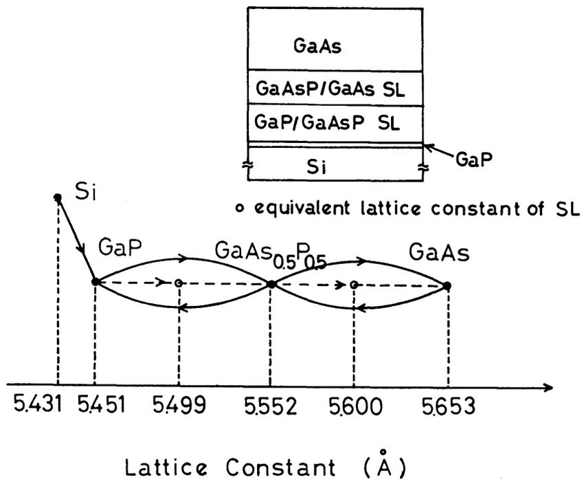
Fig. 2.13 Optimized structure to grow GaAs on Si and lattice constant of semiconductors used in this structure.
