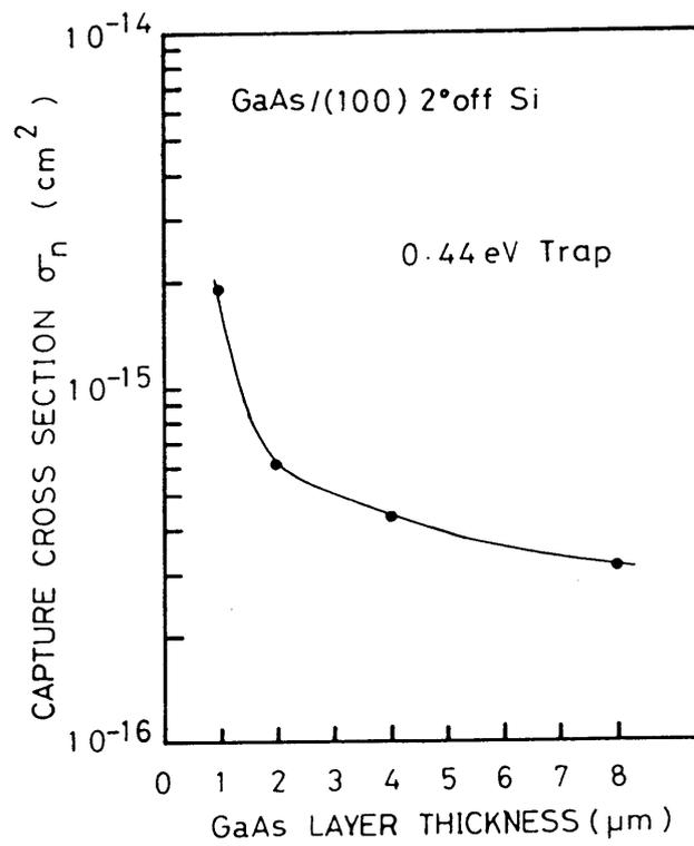
Fig. 3.23 Capture cross section of 0.44eV trap as a function of GaAs thickness.
