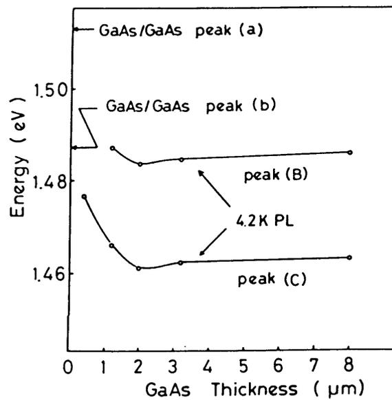
Fig. 3.11 PL peak energy as a function of GaAs thickness.
