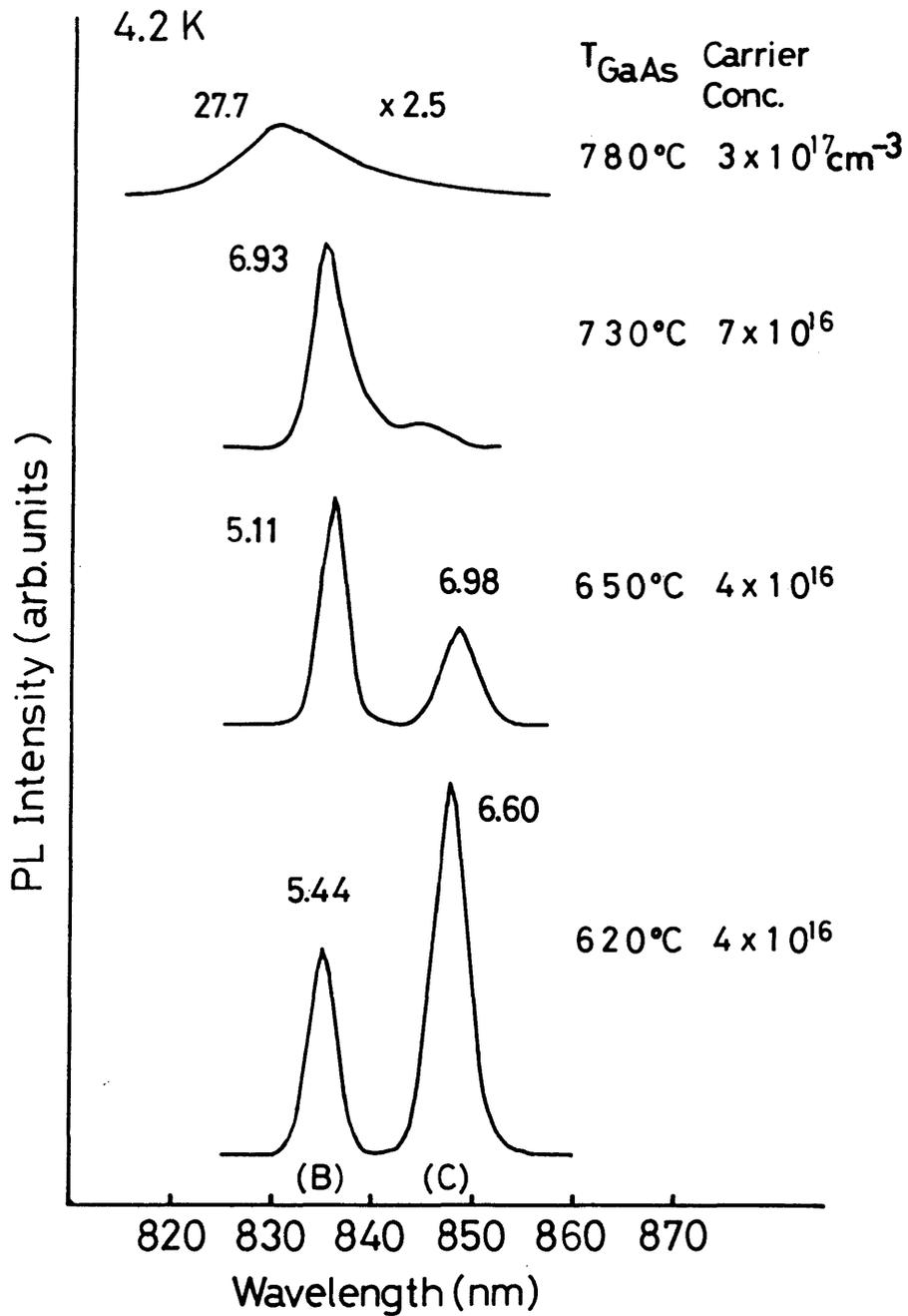
Fig. 2.16 4.2K PL spectra and room temperature carrier concentration at various growth temperature of GaAs. PL half width is indicated at the top of the peaks.
