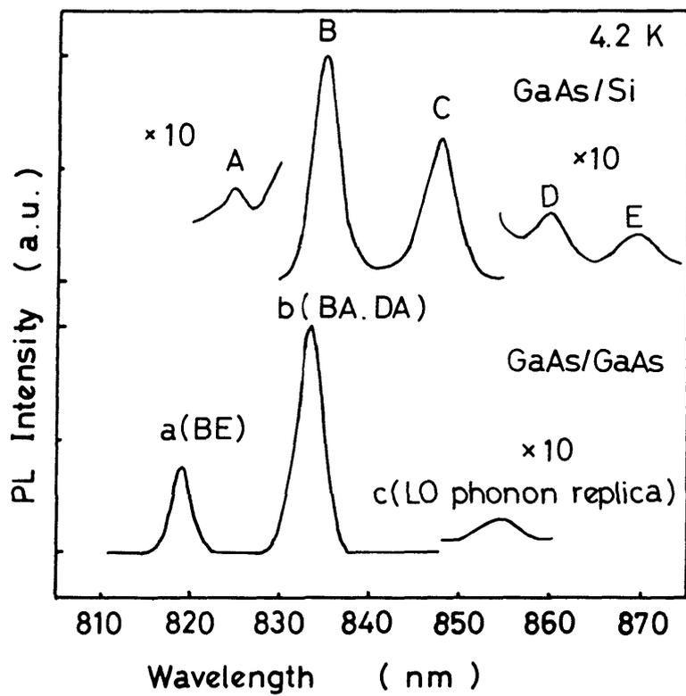
Fig. 3.7 PL spectra at 4.2K grown on Si (upper) and GaAs (lower).
