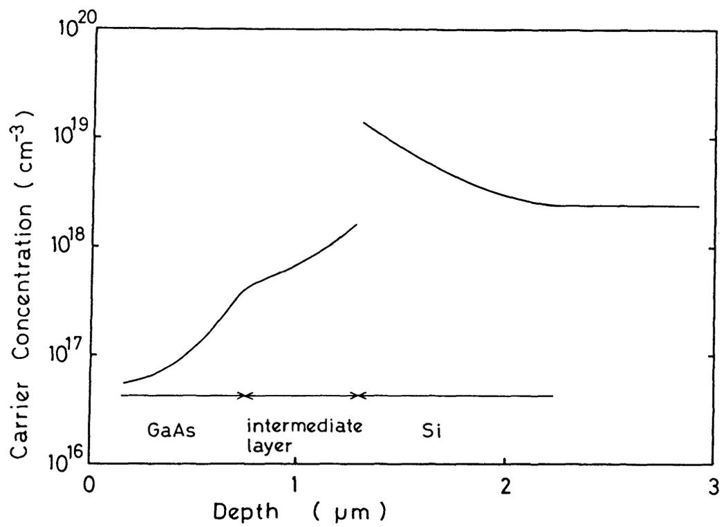
Fig. 2.11 In-depth carrier profile of GaAs on Si.
