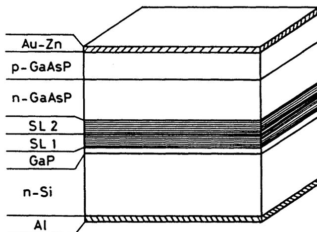
Fig. 5.7 Schematic illustration of the fabricated GaAs<sub>0.6</sub>P<sub>0.4</sub> LED on Si.
