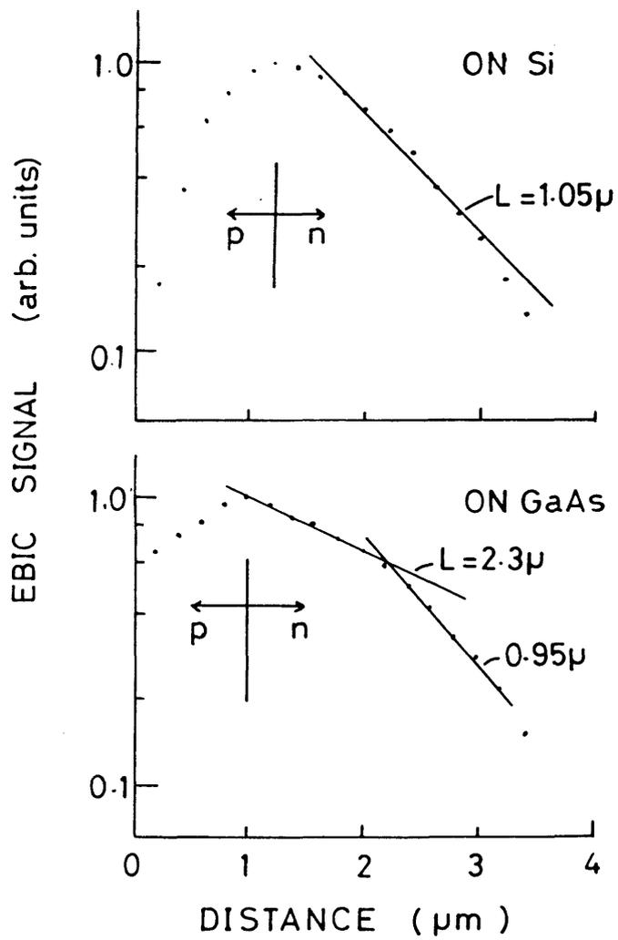
Fig. 3.29 Results of the EBIC measurement.
