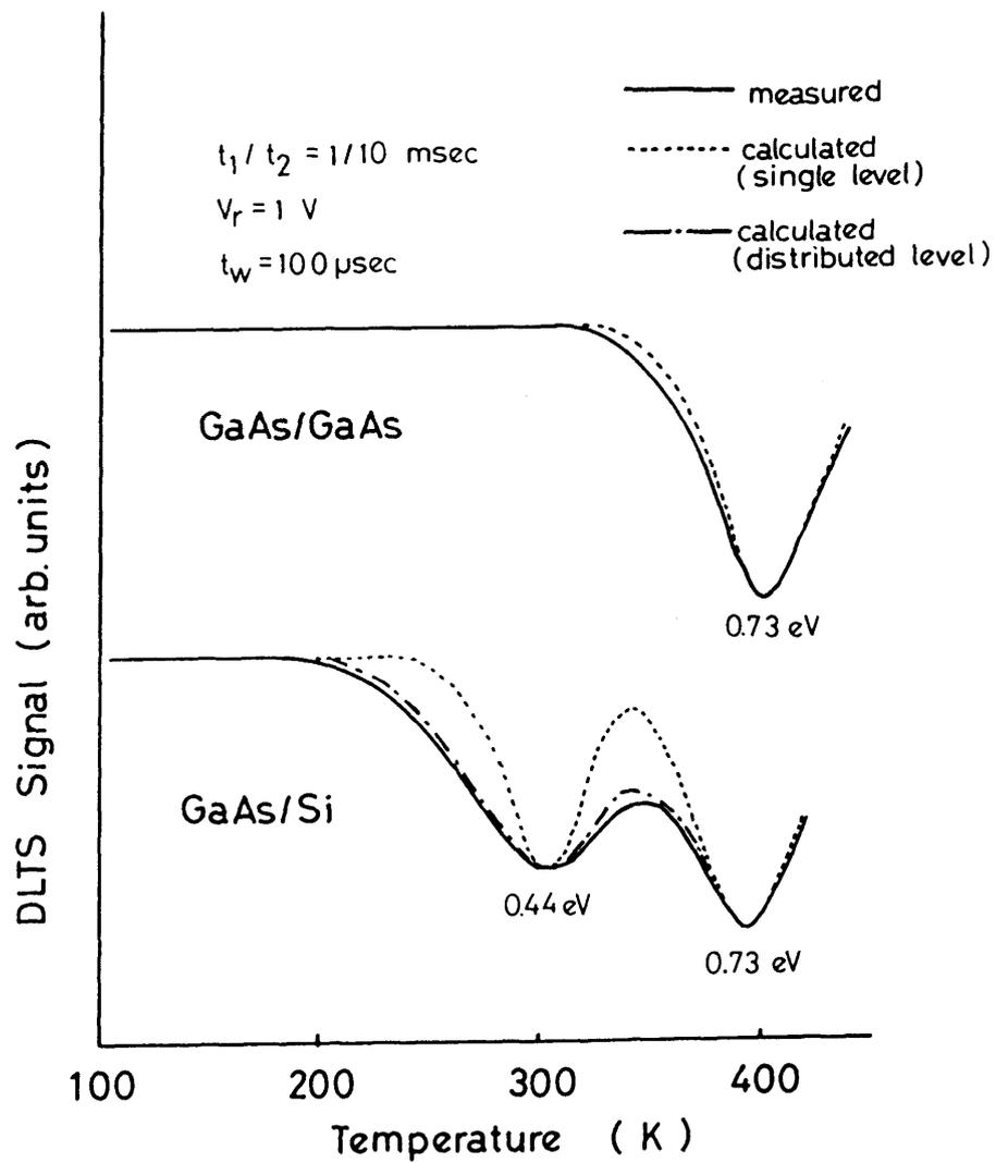
Fig. 3.20 Typical DLTS spectra of 2 $\mu$ m-thick GaAs grown on GaAs and Si.
