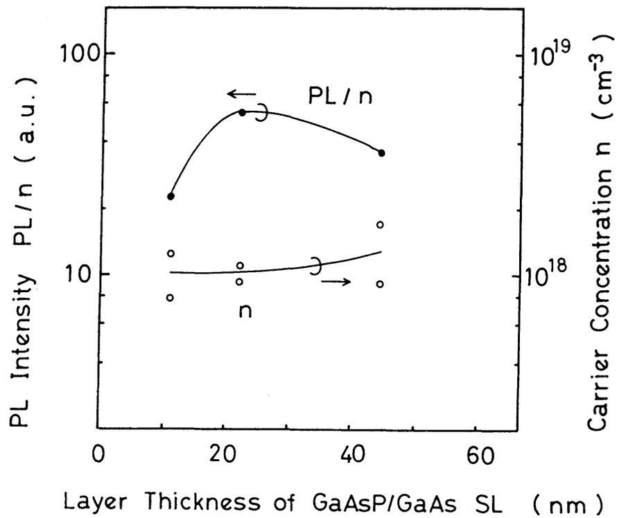
Fig. 2.9 PL intensity and carrier concentration vs. layer thickness in the superlattice.
