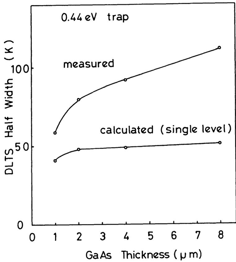
Fig. 3.24 DLTS half width of 0.44eV trap as a function of GaAs thickness.
