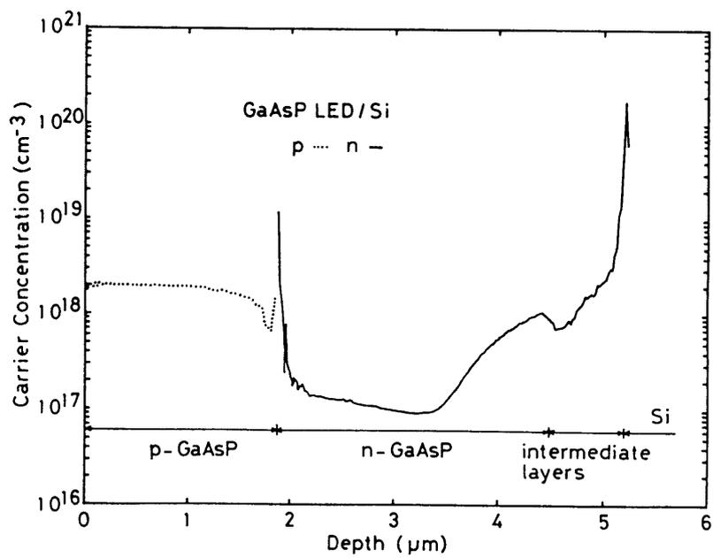
Fig. 5.9 In-depth carrier concentration profile of  $\text{GaAs}_{0.6}\text{P}_{0.4}$  LED on Si.
