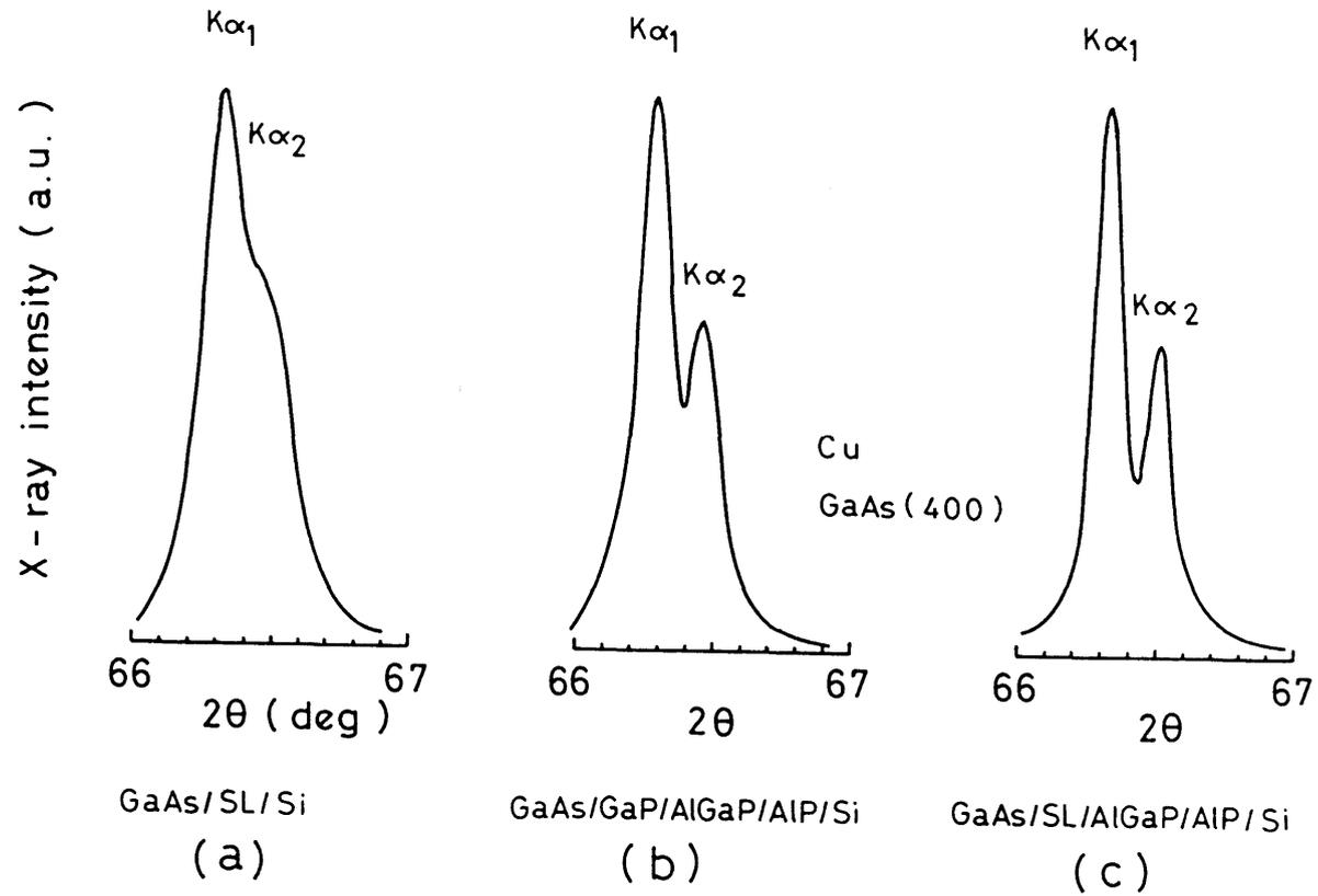
Fig. 2.4 X-ray diffraction patterns for various structures.
