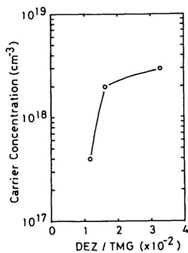
Fig. 5.8 Hole concentration of GaAs<sub>0.6</sub>P<sub>0.4</sub> as a function of DEZ/TMG mole ratio.
