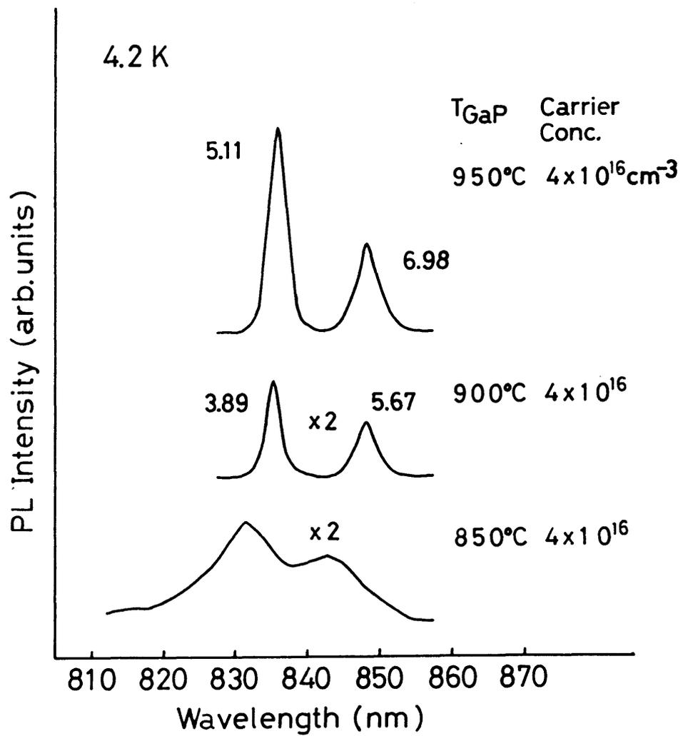
Fig. 2.17 4.2K PL spectra and room temperature carrier concentration at various growth temperature of GaP. PL half width is indicated at the top of the peaks.
