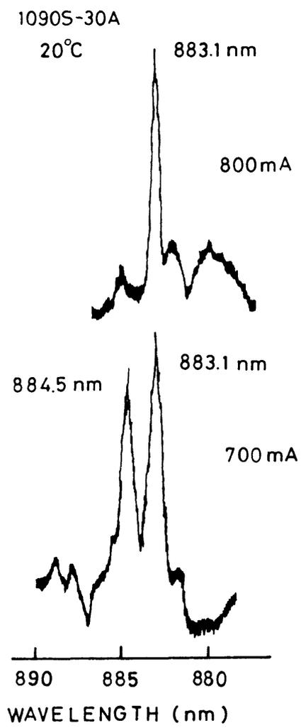
Fig. 4.5 Lasing spectra of the LD.
