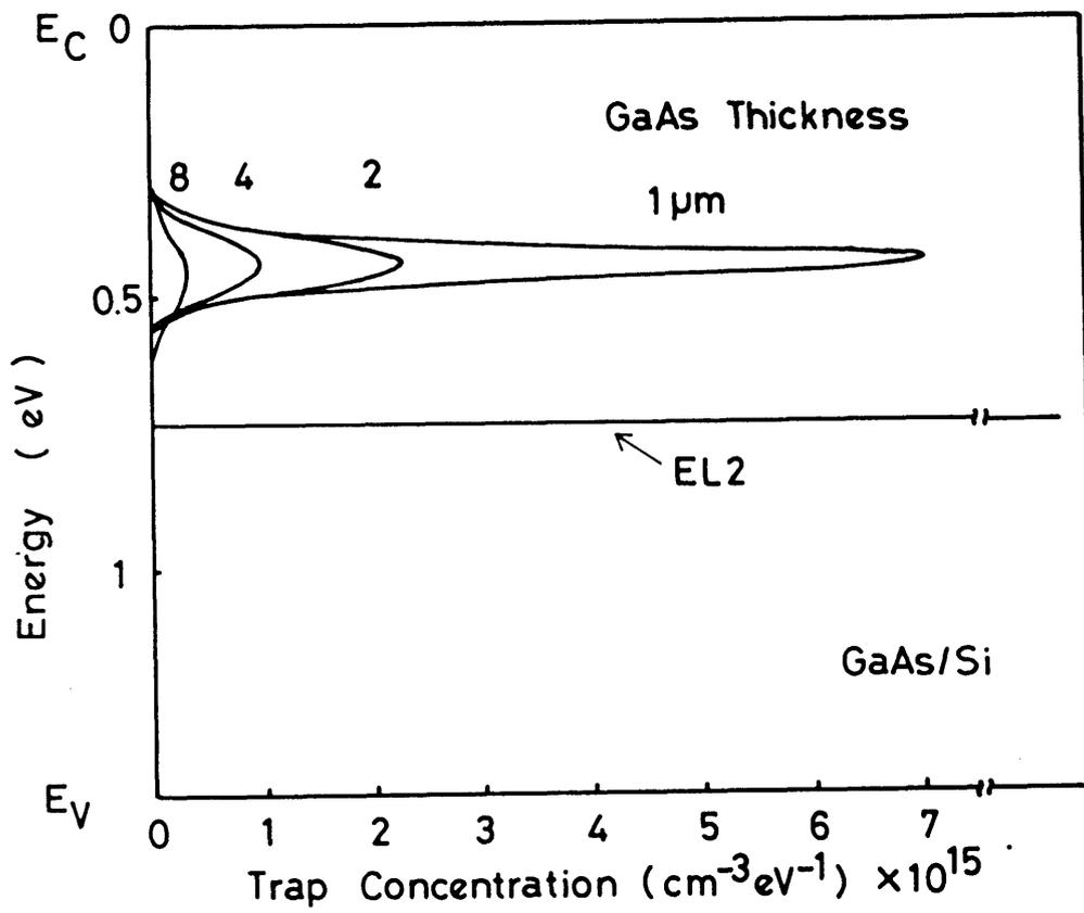
Fig. 3.25 Calculated trap levels in GaAs on Si.
