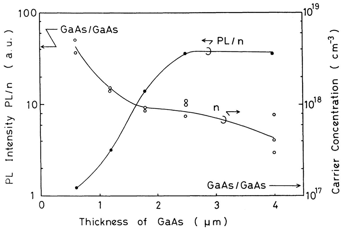
Fig. 2.10 PL intensity and carrier concentration vs. surface GaAs thickness. PL/n and n values for GaAs/GaAs epitaxial growth sample are shown by arrows.
