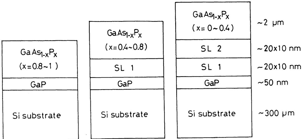
SL 1 : GaP / GaAs<sub>0.5</sub>P<sub>0.5</sub> superlattice
