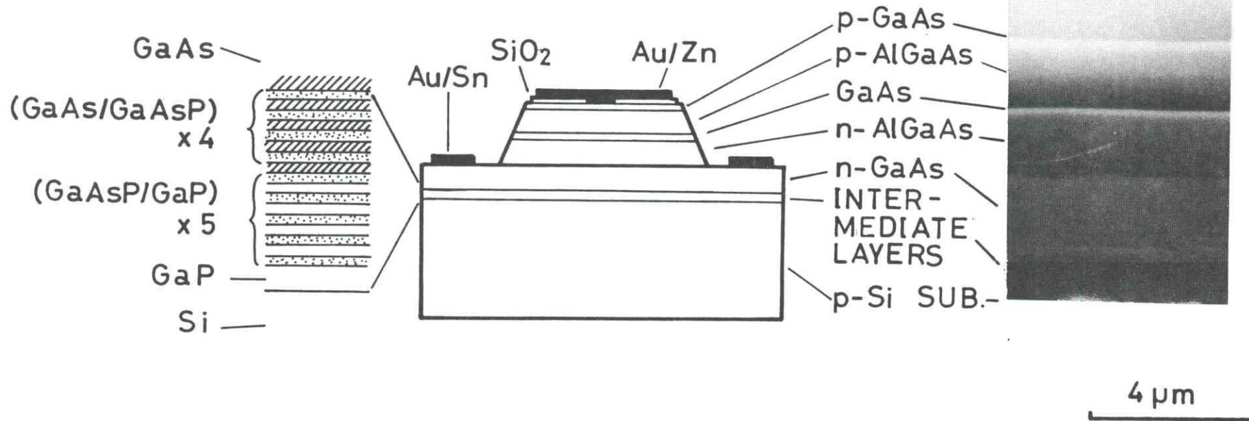
Fig. 4.2 Schematic illustration of the fabricated LD on Si and SEM microphotograph of the grown layer.
