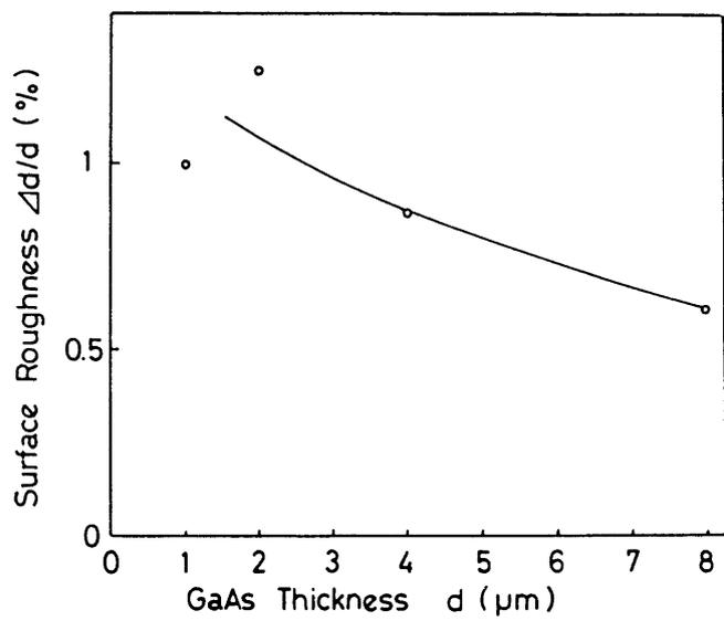
Fig. 3.5 Surface roughness of GaAs as a function on GaAs thickness.
