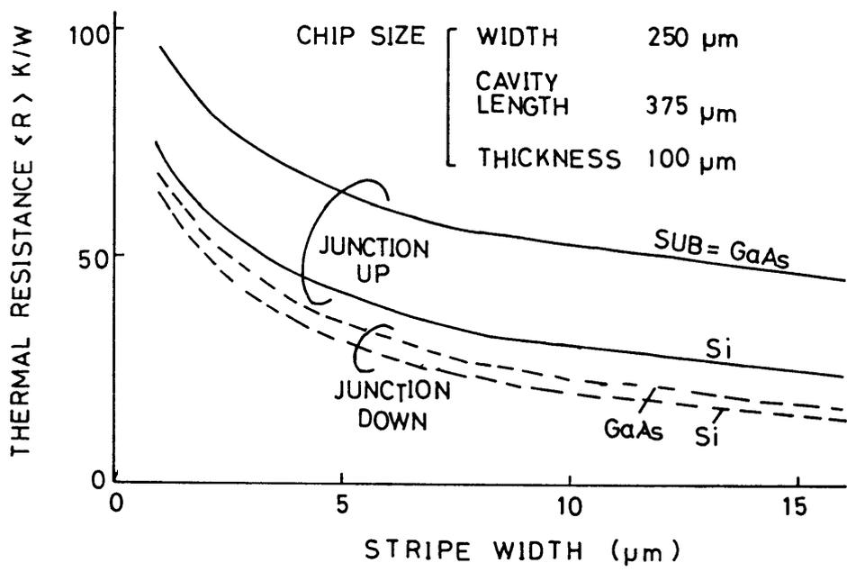
Fig. 4.1 Calculated thermal resistance of stripe LD on Si and GaAs as a function of stripe width.
