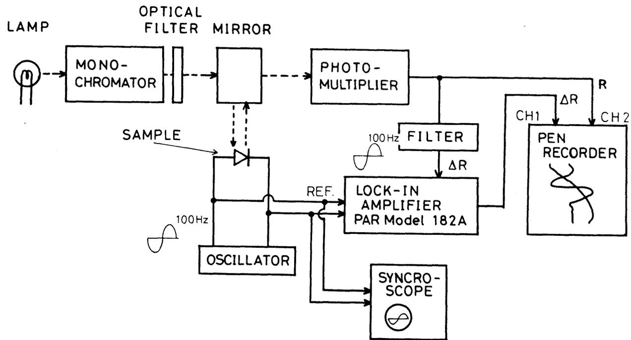
Fig. 3.12 Electroreflectance measurement system.
