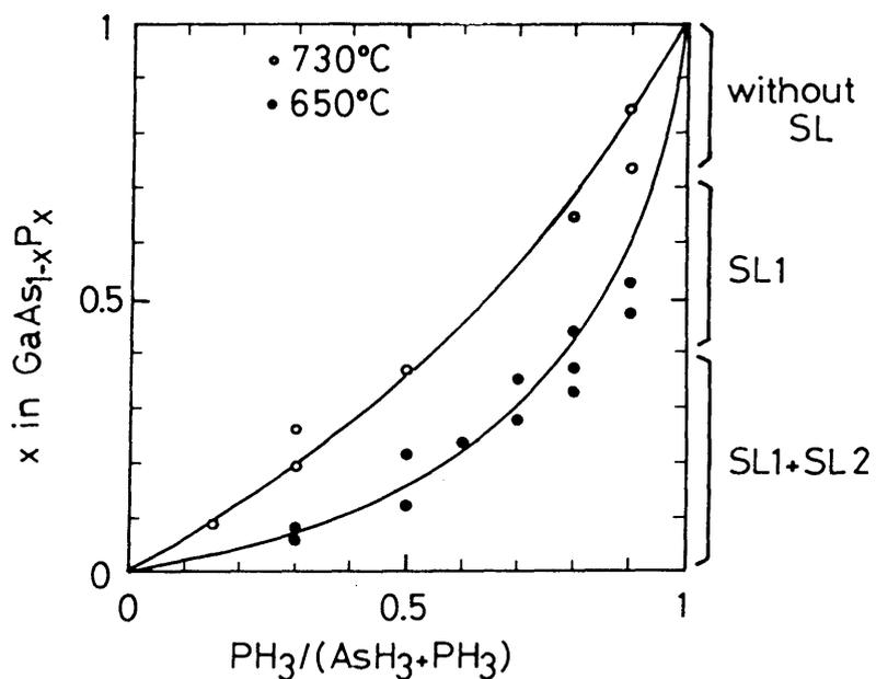
Fig. 5.2 GaAs<sub>1-x</sub>P<sub>x</sub> solid composition as a function of gas phase composition [PH<sub>3</sub>]/[AsH<sub>3</sub>+PH<sub>3</sub>] at 650 and 730 °C.
