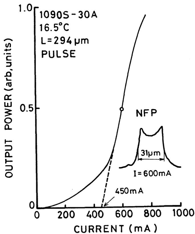
Fig. 4.4 Current/output power relation of the LD.
