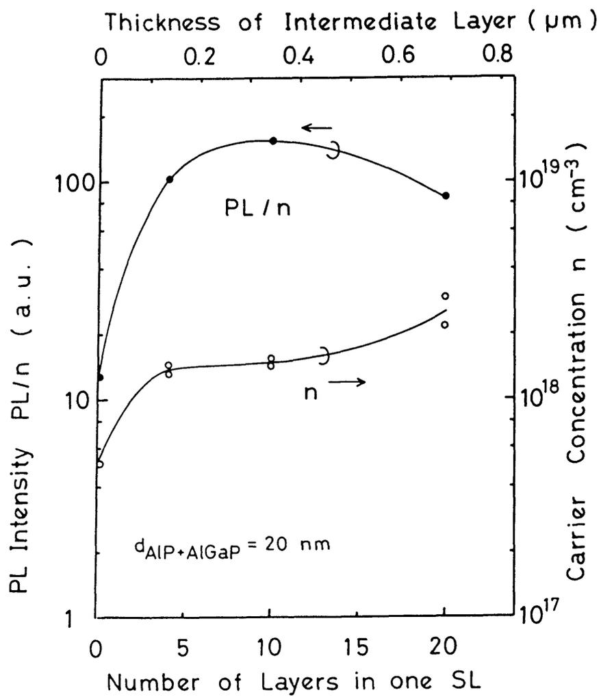
Fig. 2.8 PL intensity and carrier concentration vs. layer number in one superlattice.
