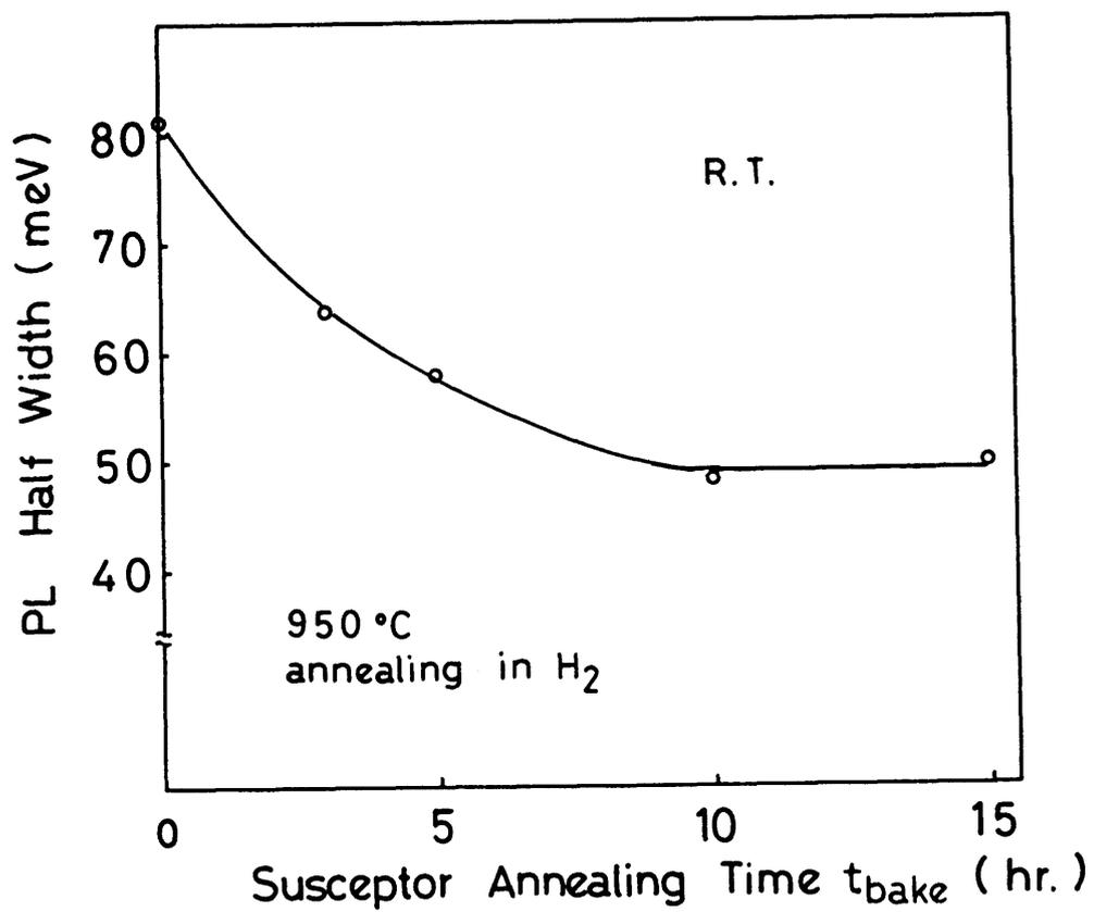
Fig. 2.15 Room temperature PL half width vs. annealing time of the susceptor.
