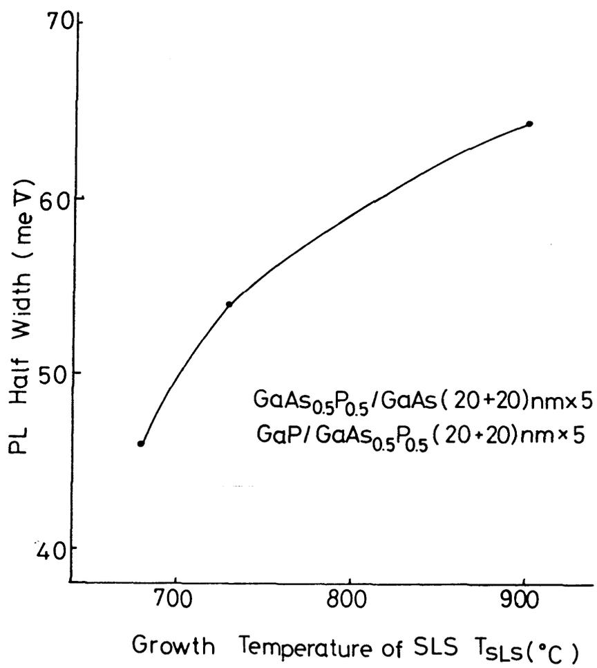
Fig. 2.18 Room temperature PL half width vs. growth temperature of SLS.
