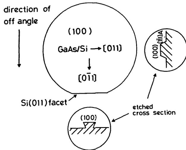
Fig. 3.1 Crystal orientation of GaAs on Si.
