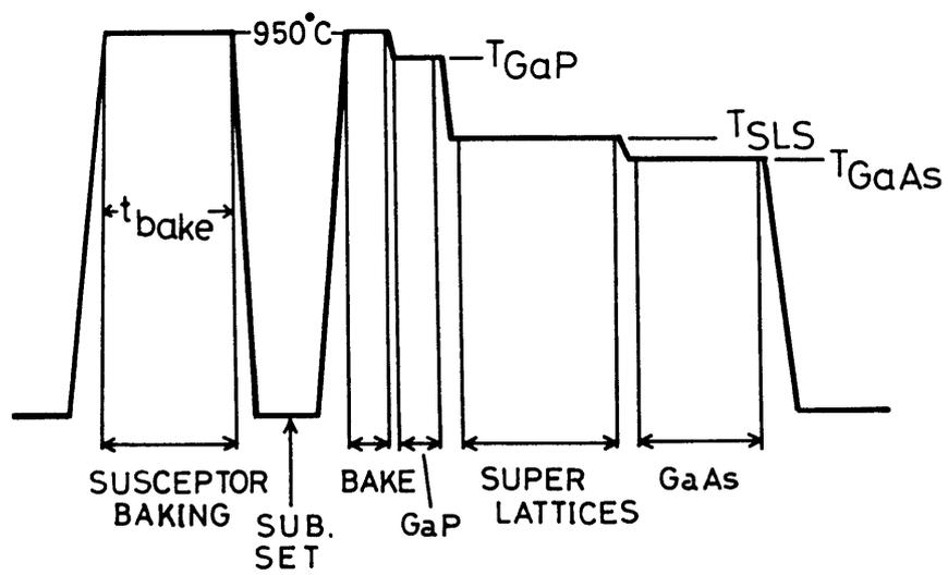
Fig. 2.12 Temperature program to grow GaAs on Si.
