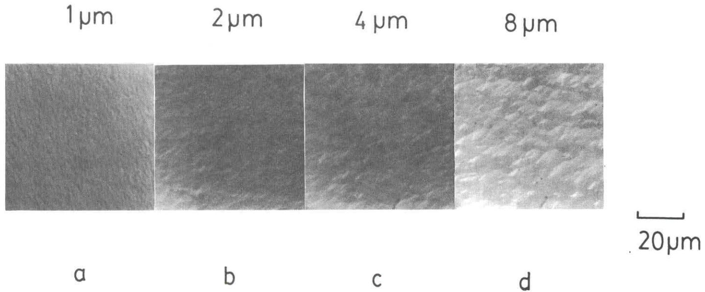
Fig. 3.4 Nomarski surface microphotographs of GaAs grown on Si.
