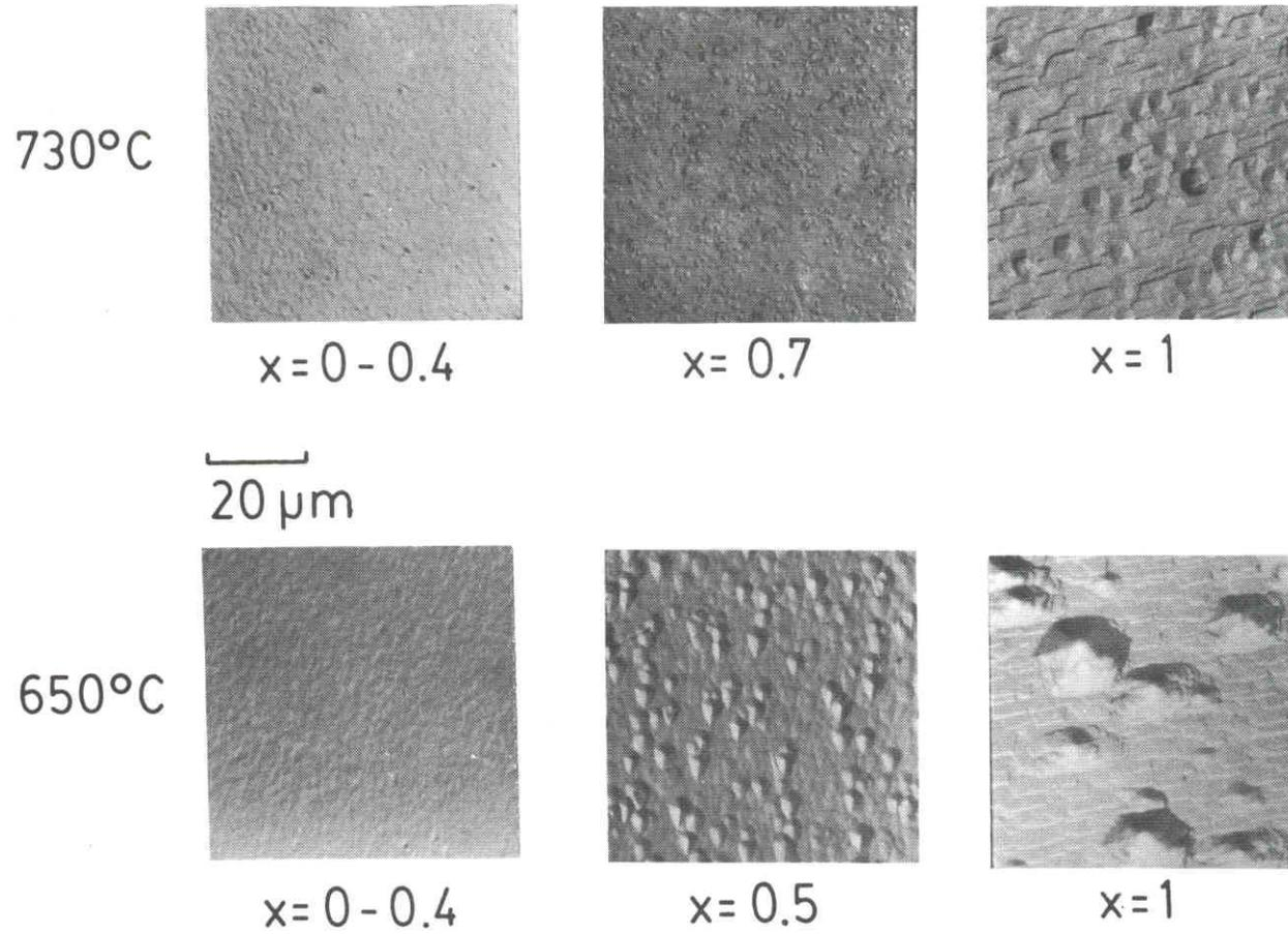
Fig. 5.4 Nomarski surface micro photographs of  $\text{GaAs}_{1-x}\text{P}_x$  grown at 650 and 730 °C.
