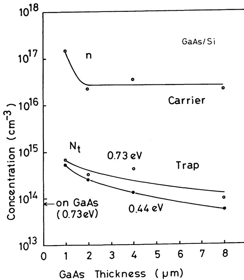
Fig. 3.22 Carrier concentration and trap concentration as a function of GaAs thickness.
