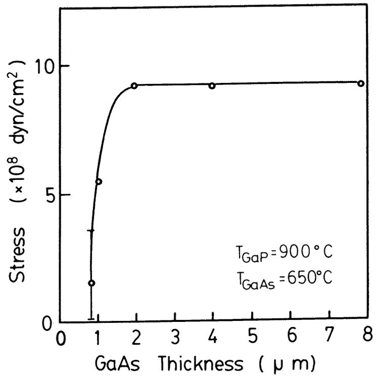
Fig. 3.9 Stress calculated from the curvature radius as a function of GaAs thickness.
