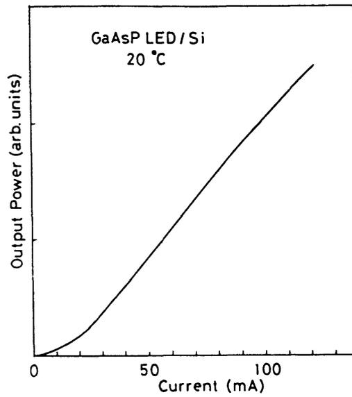
Fig. 5.10 Current/output power relation of the  $\text{GaAs}_{0.6}\text{P}_{0.4}$  LED on Si.
