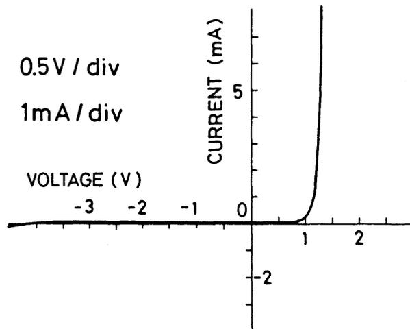
Fig. 4.3 Current/voltage relation of the LD.
