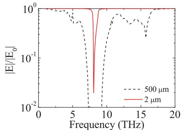
FIG. 4. (Color online) Calculated absorption spectra of GaAs due to phonon resonance using handbook data. (Ref. 11) Solid and dotted lines show calculations for GaAs thicknesses of 2 and  $500 \mu\text{m}$ , respectively. The absorption line and band widths at 10 dB above the bottom of the absorption line are 0.29 and 3.15 THz, respectively. The corresponding widths of experimental data in Fig. 3 are 0.52 and 3.37 THz, respectively.
