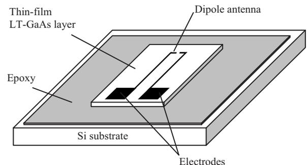
FIG. 1. Schematic illustration of an ELT-PCS. A thin-film LT-GaAs layer with an antenna is bonded onto a Si substrate with epoxy adhesive.
