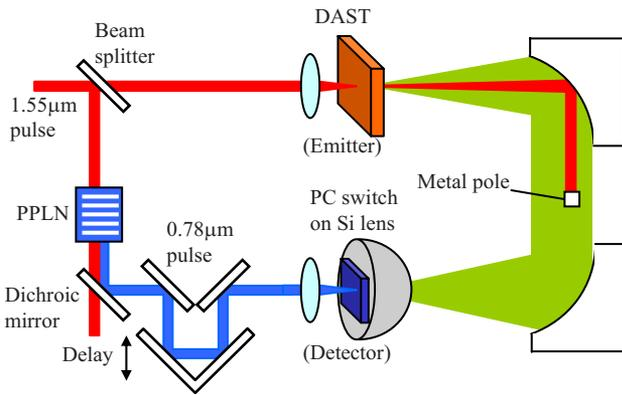
FIG. 2. (Color online) Experimental setup of broadband terahertz-TDS. Terahertz pulses were emitted from a DAST crystal using a  $1.55 \mu\text{m}$  wavelength ultrashort-pulse fiber-based laser. A detector PCS was operated by frequency-doubled ultrashort-pulse laser.
