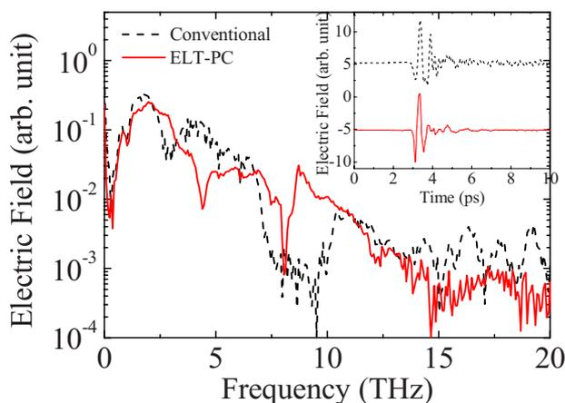
FIG. 3. (Color online) Terahertz time-domain wave forms (inset) and corresponding Fourier transform spectra. The absorption band of 7–10 THz of the conventional PCS (dotted line) was reduced by replacing it with an ELT-PCS (solid line), except for the sharp absorption at 8 THz.
