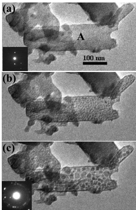
FIG. 1. Low-dose TEM observations of the dehydrating process of  $\text{AlH}_3$  particles. Selected area diffraction patterns from particle A are shown in the insets in (a) and (c). Each photograph was taken on an exposure of 5 s.
