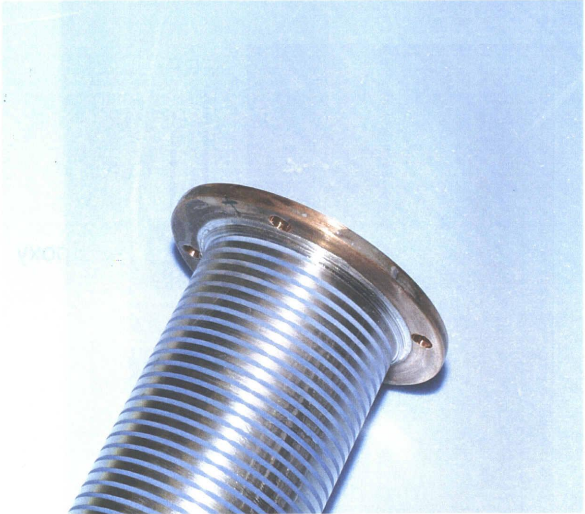
(b) Bi2212 coil without epoxy impregnation
