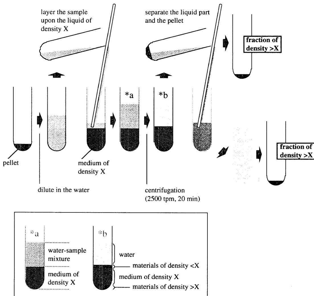
Fig. 2 : Procedure to separate different density fractions of the sediment (modified after Regnéll & Everitt, 1996).
