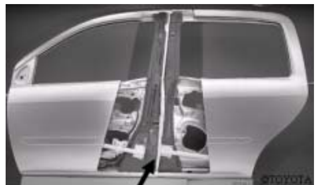
Fig. 1-9 Example of porous Al filling automobile parts. ( From the catalog of Ferrari and Alulight )
