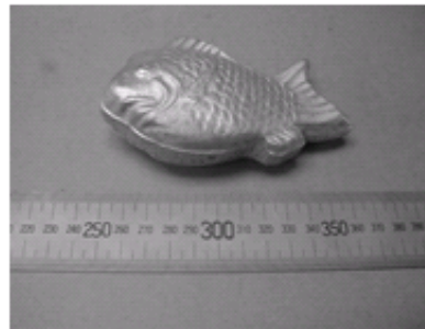
The fish-shaped aluminum foam with skin
