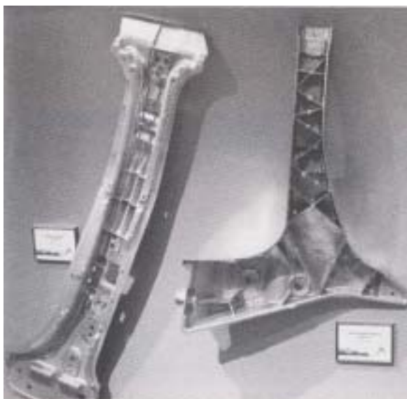
Center pillar (left) and lateral member (right) of Audi A2 (ALUMINUM, 8(2001)40, p. 9)
