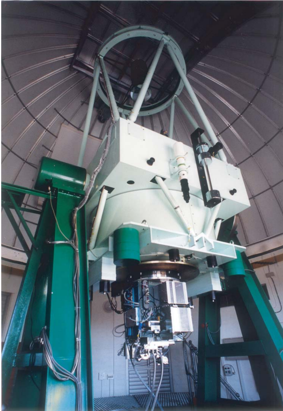
Figure 2.1: 1.4 m telescope and the SIRIUS camera. The camera is installed at the Cassegrain focus of the telescope.
