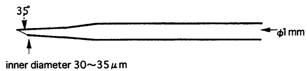
Fig. 2. Microneedle. Microneedles are prepared by pulling 1 mm (outer diameter) glass capillary tubing with a puller (NARISHIGE PN-3, supplied by Narishige Co., Tokyo). The tip of microneedle is sharpened with a needle sharpener (NARISHIGE EG-4). The inner diameter at the opening is 30–35 µm and the angle is 35°.
