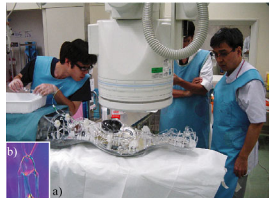
Fig. 1: a) Medical training with the simulation system for endovascular surgery. b) Birefringence produced by guide wire in urethane model of aneurysm.
