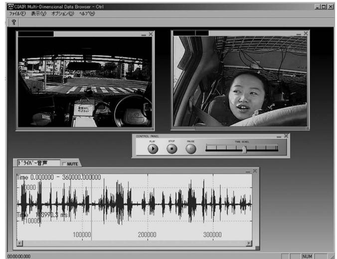
Fig. 2. Multimedia data browser utilized by taggers for subjective selection and ranking of potentially hazardous scenes from the database. In-car videos are shown at the top, and the speech waveform is shown at the bottom.
