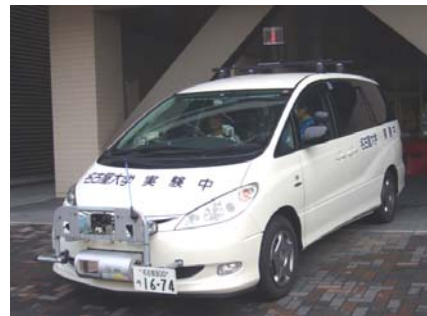
Fig.5 Data collection vehicle used for recording video
