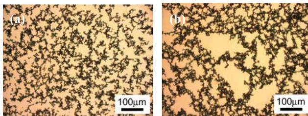
Figure 1: Aggregation of the magnetic particles in the liquid photocurable polymer matrix without additives (a) immediately after mixing and (b) 1 h later.
