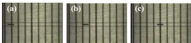
Figure 6: Photographs of the screw-type microactuator with a diameter of 0.1 mm swimming in the capillary with an inner diameter of 0.2 mm filled with water at a rotational frequency of 500Hz: (a) 0s, (b) 0.5 s and (C) 1 s later
