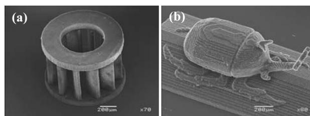
Figure 4: 3D magnetic microstructures fabricated by microstereolithography: (a) micro sirocco fan with a diameter of 1 mm and height of 0.7 mm; (b) beetle with a length of 2 mm, width of 1 mm, and height of 0.66 mm.
