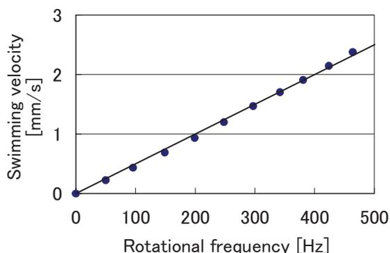
Figure 7: Relationship between the rotational frequency of the magnetic field and the swimming velocity of the screw-type microactuator with a diameter of 0.1 mm
