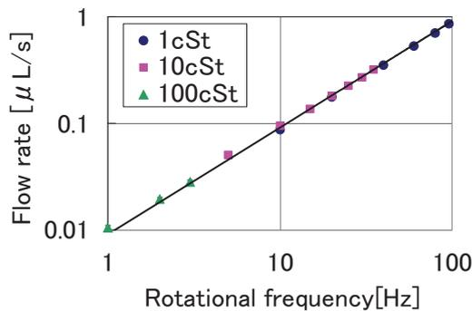
Figure 9: Relationship among the flow rate of micro-screw pump, the rotational frequency of magnetic field and the kinetic viscosity of fluid
