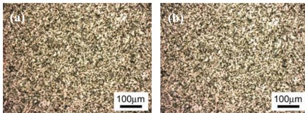
Figure 2: Dispersion of the magnetic particles in the liquid photocurable polymer matrix with the viscosity-increasing agent (a) immediately after mixing and (b) 1 h later.
