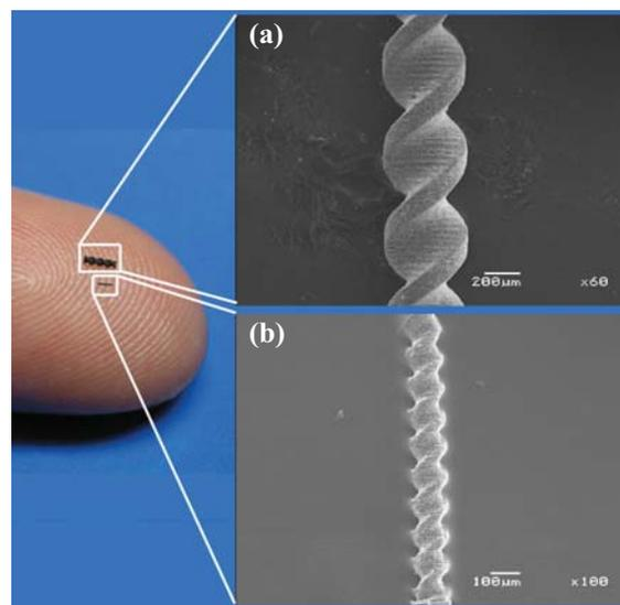
Figure 3: Magnetic microscrews fabricated by microstereolithography: (a) with a diameter of 0.5 mm, length of 2 mm, and spiral pitch of 1 mm and (b) with a diameter of 0.1 mm, length of 1 mm, and spiral pitch of 0.2 mm
