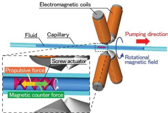
Figure 8: Schematic diagram of micro-screw pump
