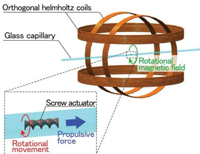
Figure 5: Schematic diagram of the wirelessly controllable swimming micromachine driven by magnetic force
