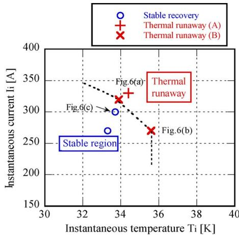
Fig. 7. Thermal runaway characteristics during load fluctuation compensating operation at operating temperature  $T_0 = 24$  K,  $dI/dt = -20$  A/s and  $I_0 = 270$  A. Dashed line represents the thermal runaway criterion for standby current  $I_0 = 270$  A.
