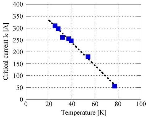
Fig. 2. Critical current  $I_c$  as a function of temperature.
