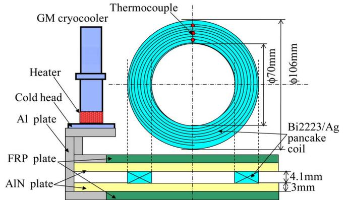
Fig. 1. Arrangement of a single pancake coil sample.
