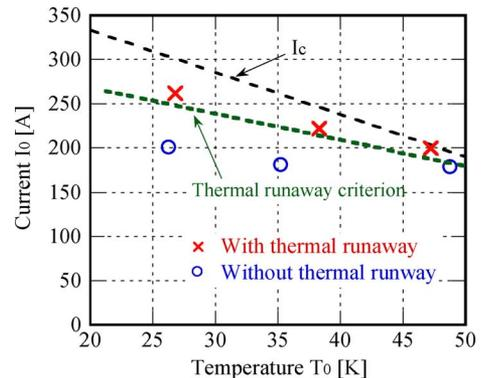
Fig. 4. Thermal runaway criterion for steady current  $I_0$  as a function of the operating temperature  $T_0$ .
