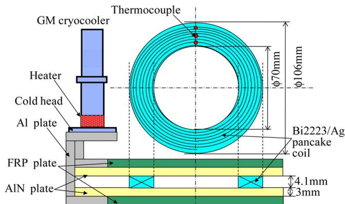
Fig. 1. Arrangement of a single pancake coil sample.
