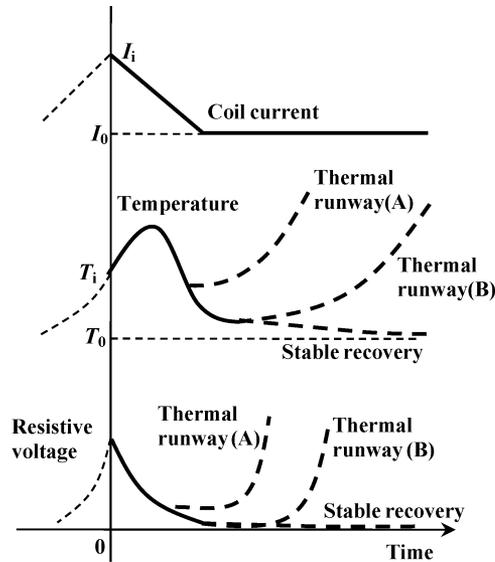
Fig. 5. Pattern of the injected coil current and typical temporal evolution of the temperature and the resistive voltage of the coil for simulating the recovery process in load fluctuation compensating operation.
