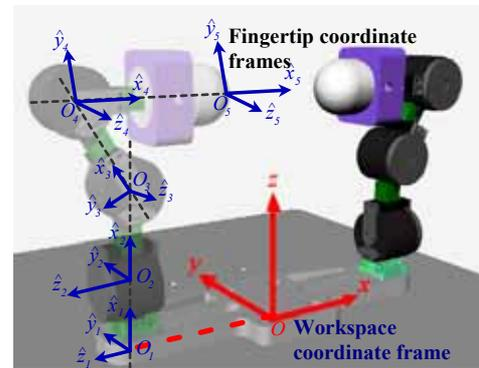
Fig. 2. Coordinate frames at robot finger and workspace.
