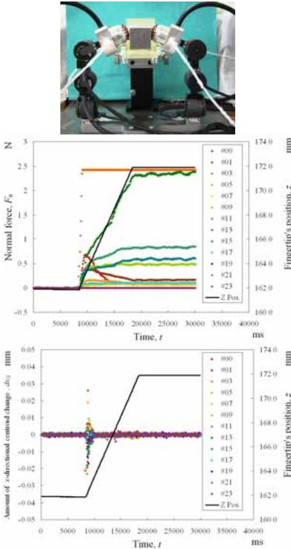
Fig. 3. Relationship between normal (*top*) and shearing (*bottom*) forces with fingertip position at  $z$ -axis for experiment with aluminum block at right finger.
