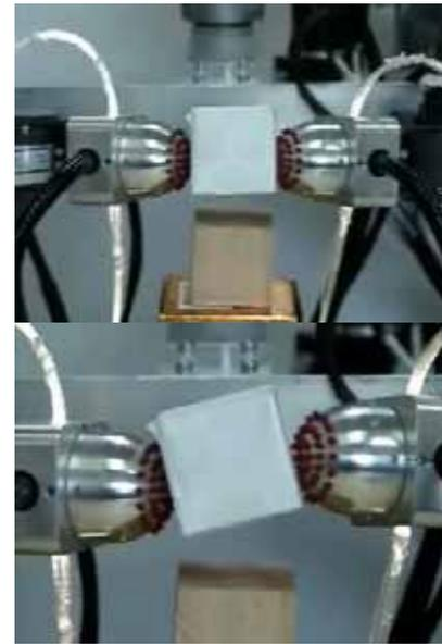
Fig. 5. Verification experiment I: Robot fingers grasp and twist paper box.
