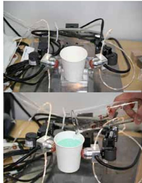
Fig. 6. Verification experiment II: Robot fingers grasp an empty cup and then water is poured inside it.
