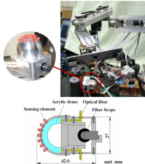
Fig.1. A multi-fingered humanoid arm mounted with optical three-axis tactile sensors at fingertips, and the structure of the tactile sensor.
