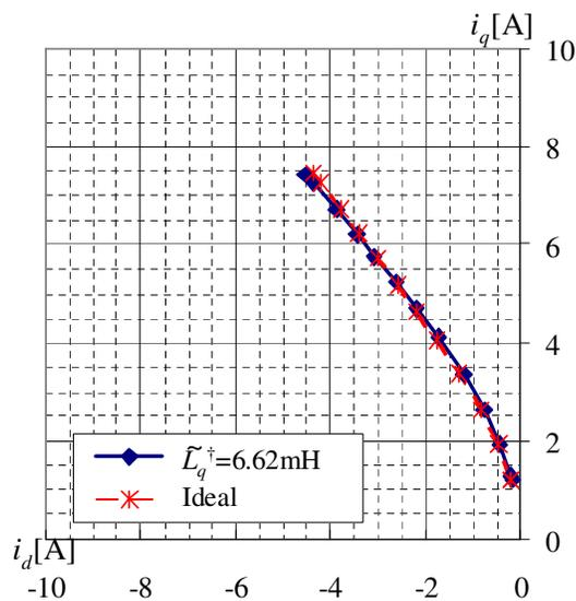
Fig. 7. Loci of the current vector on  $d$ - $q$  axes.
