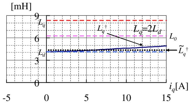
Fig. 4. Inductance setting for low saliency without magnetic saturation.
