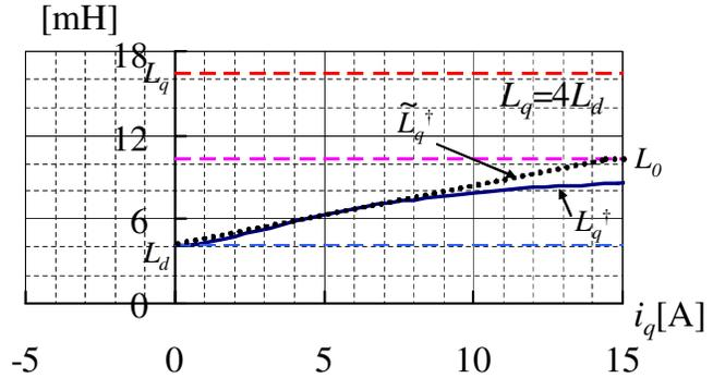
Fig. 5. Inductance setting for high saliency without magnetic saturation.
