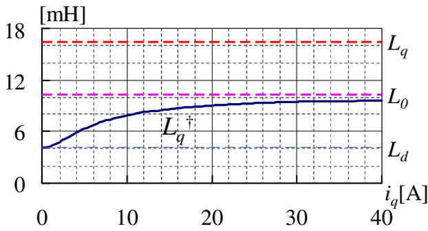
Fig. 3. Inductance – current ( $L_q^\dagger$ - $i_q$ ) characteristics.
