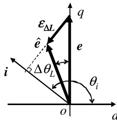
Fig. 1. Position estimation error caused by inductance errors.
