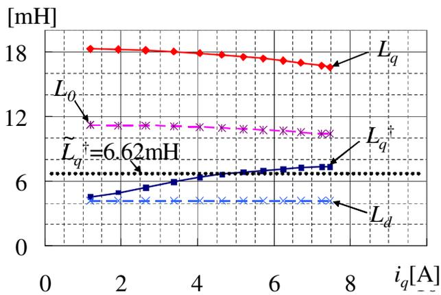
Fig. 6. Measurement results of  $L_q$  and  $L_q^\dagger$ .
